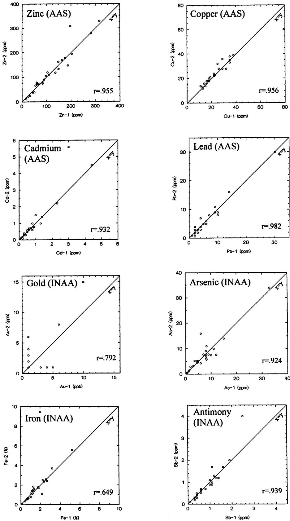
Figure 4. Scatterplots of field duplicate pairs (N=26) for zinc, copper, cadmium and lead (AAS) and for gold, arsenic, iron and antimony (INAA).
