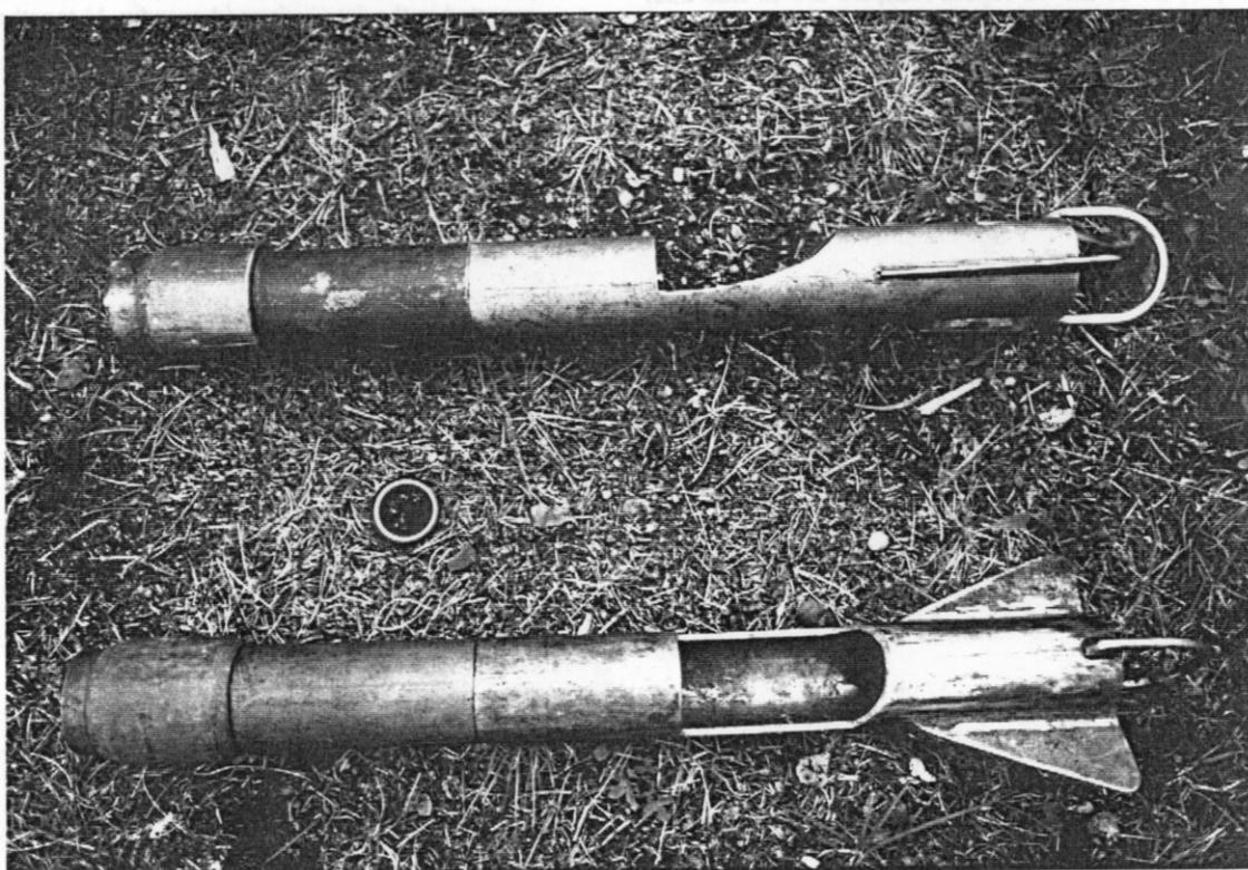
Photo 4. Hornbrook-type lake sediment sampler used in regional geochemical surveys
