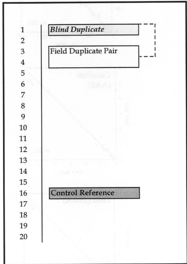
Figure 3. Typical Regional Geochemical Survey sample collection scheme used during the lake sediment survey. The 20-sample collection block incorporates 17 routine samples, a field duplicate sample, a blind duplicate sample and a control reference standard. Blind duplicates are routinely taken from the first sample of each field duplicate pair.
