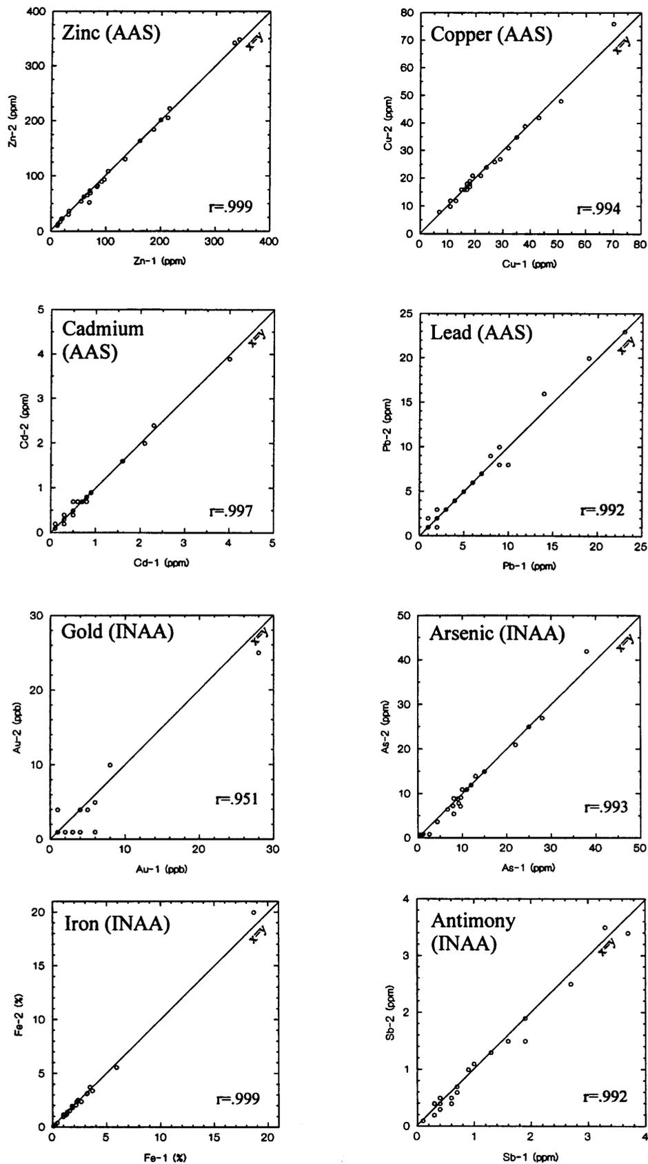
Figure 5. Scatterplots of blind duplicate pairs (N=27) for zinc, copper, cadmium and lead (AAS) and for gold, arsenic, iron and antimony (INAA).
