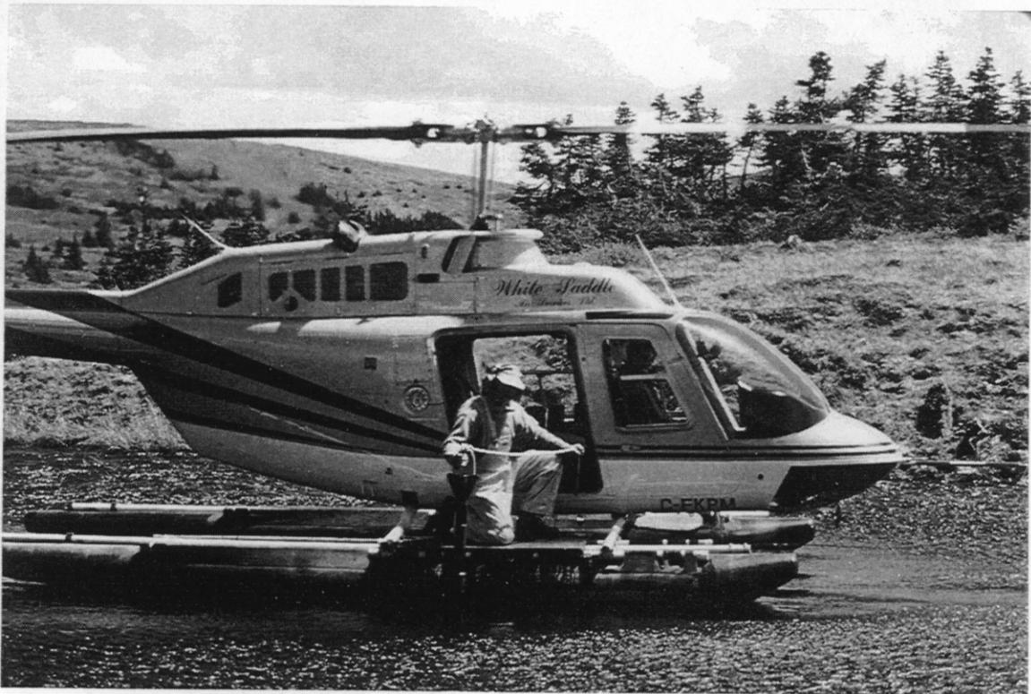
Photo 1. Regional lake sediment and water sampling in the Interior Plateau using a float-equipped helicopter (Fawnie Range, southern Nechako Plateau, June 1993).
