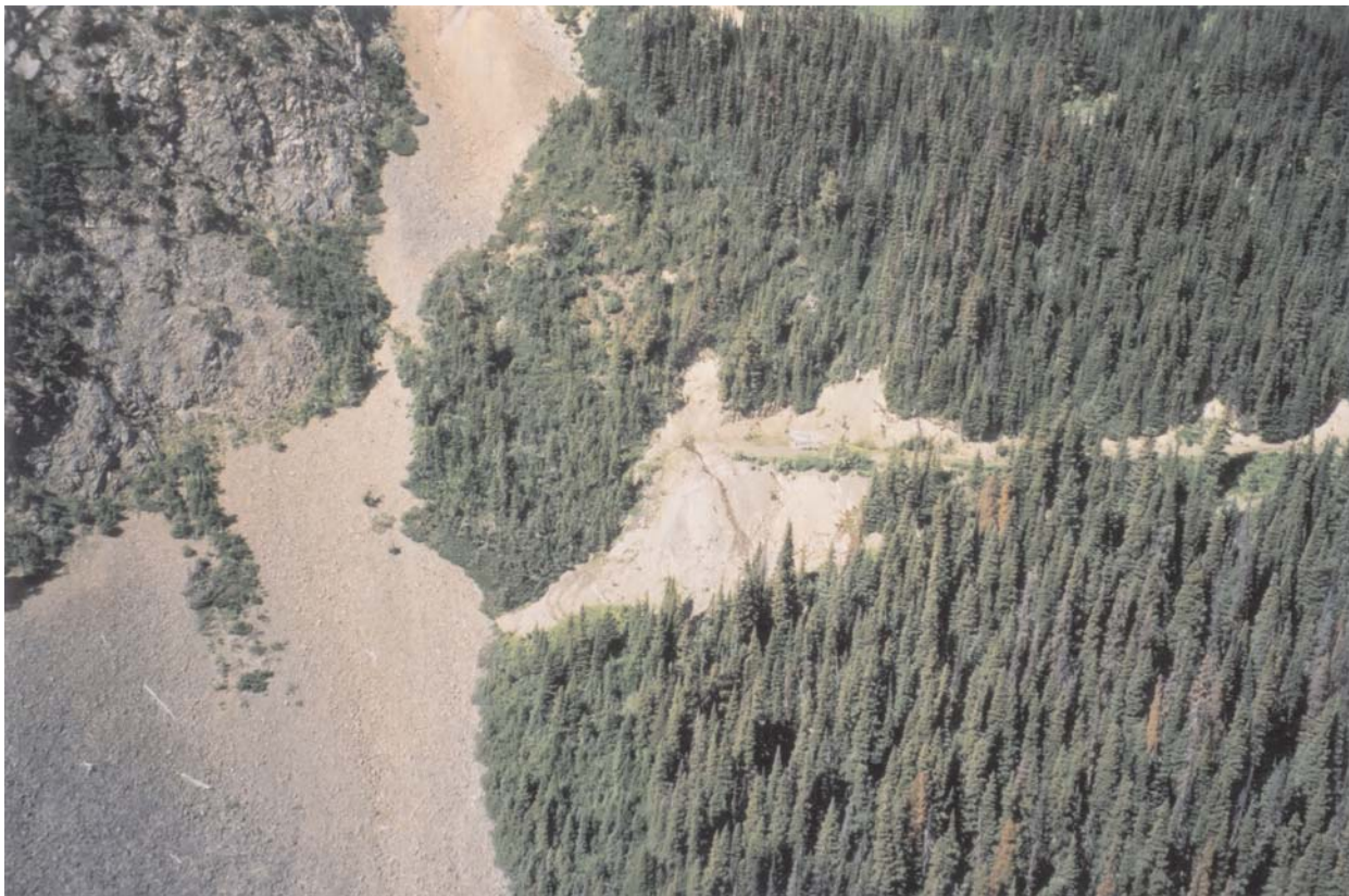
Photo 5. Cronin lower portal. Note the adit drainage flowing over the dump.
