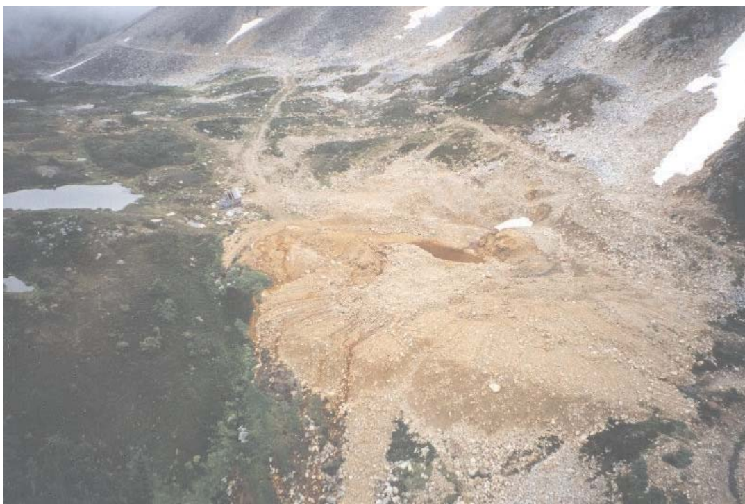
Photo 10. Area of disturbance at the Sultana mine site. The portal is located under the patch of snow. Note the drainage pooling and draining from the portal (dark red).
