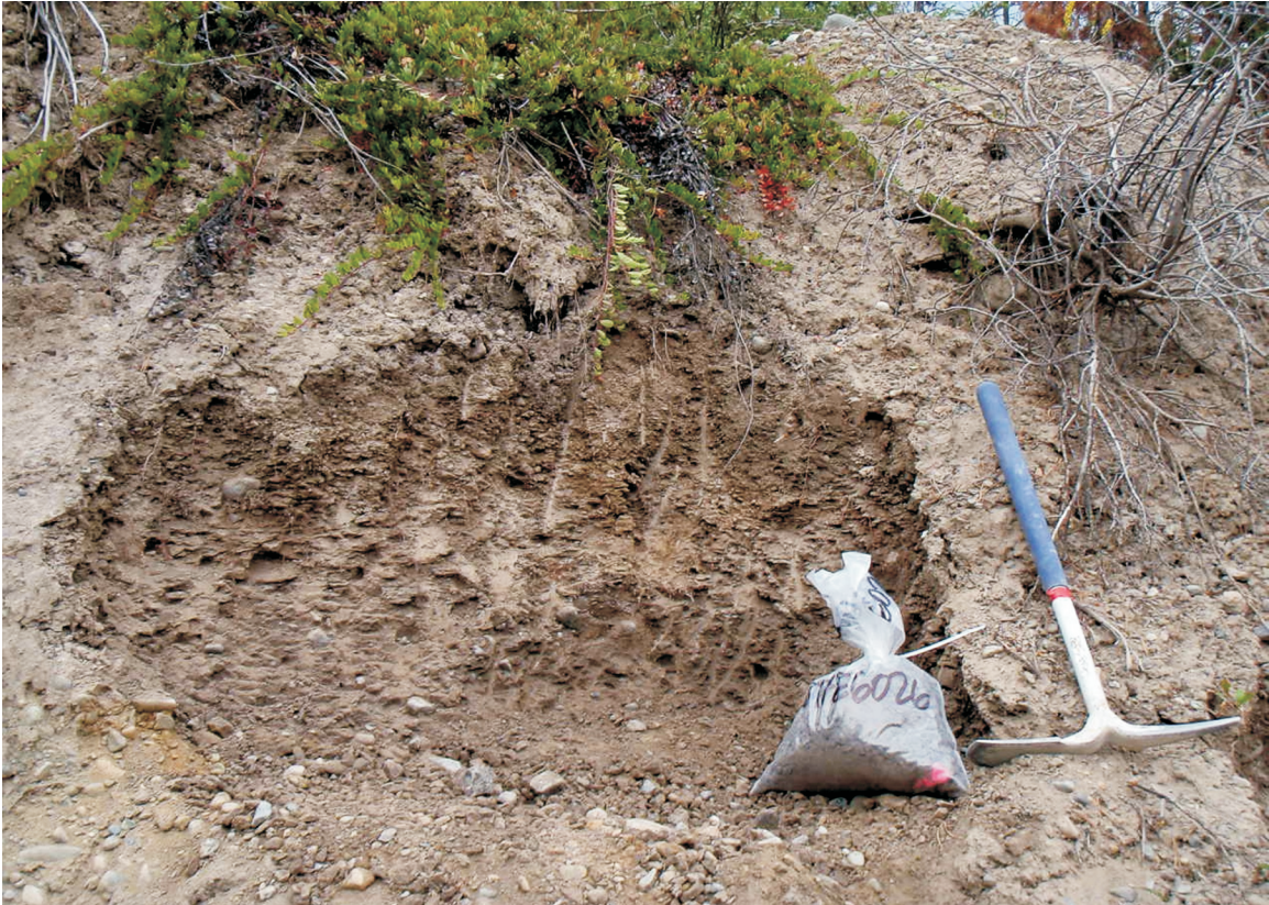
Figure 8. Example of a sample site in NTS 93B/05 (08TFE6026). Note blocky structure of basal till. This sample was collected 85 cm below surface.
