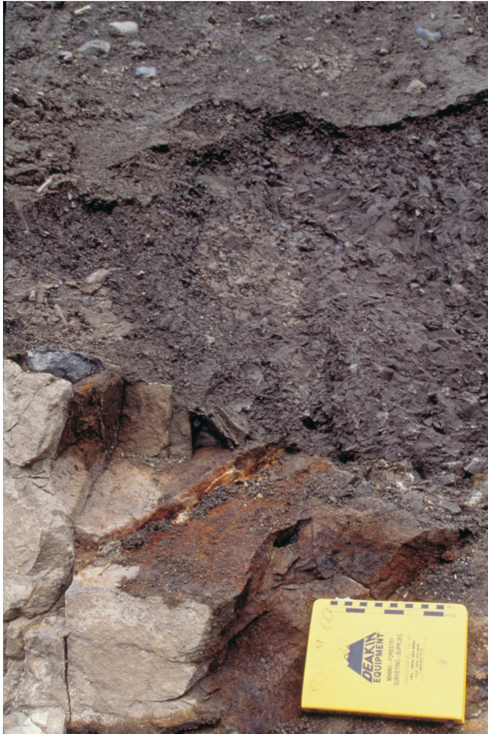
Figure 4. A typical example of a dark grey, overconsolidated, clayey-silt basal till at Huckleberry Mine. The blocky appearance is due to well developed joint and fissility planes. In this photo, basal till is overlying mineralized andesite (pyrite±chalcopyrite) of the East Zone orebody.
