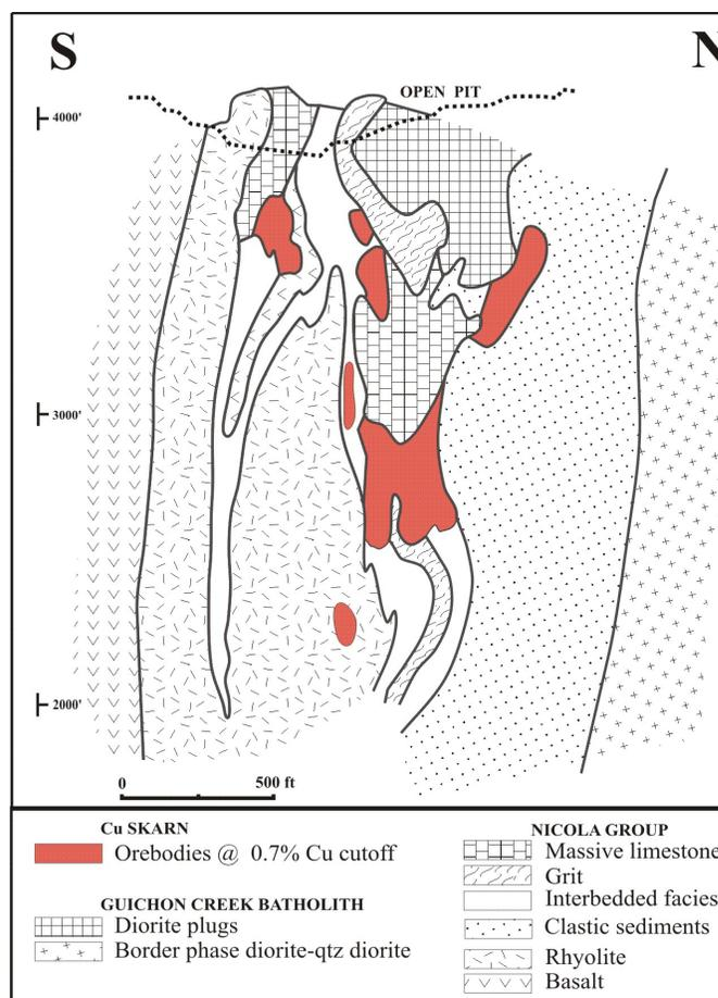
**Fig. 10.** Simplified north-south section across the Craigmont Cu skarn deposit, southern BC. After Morrison (1980).
