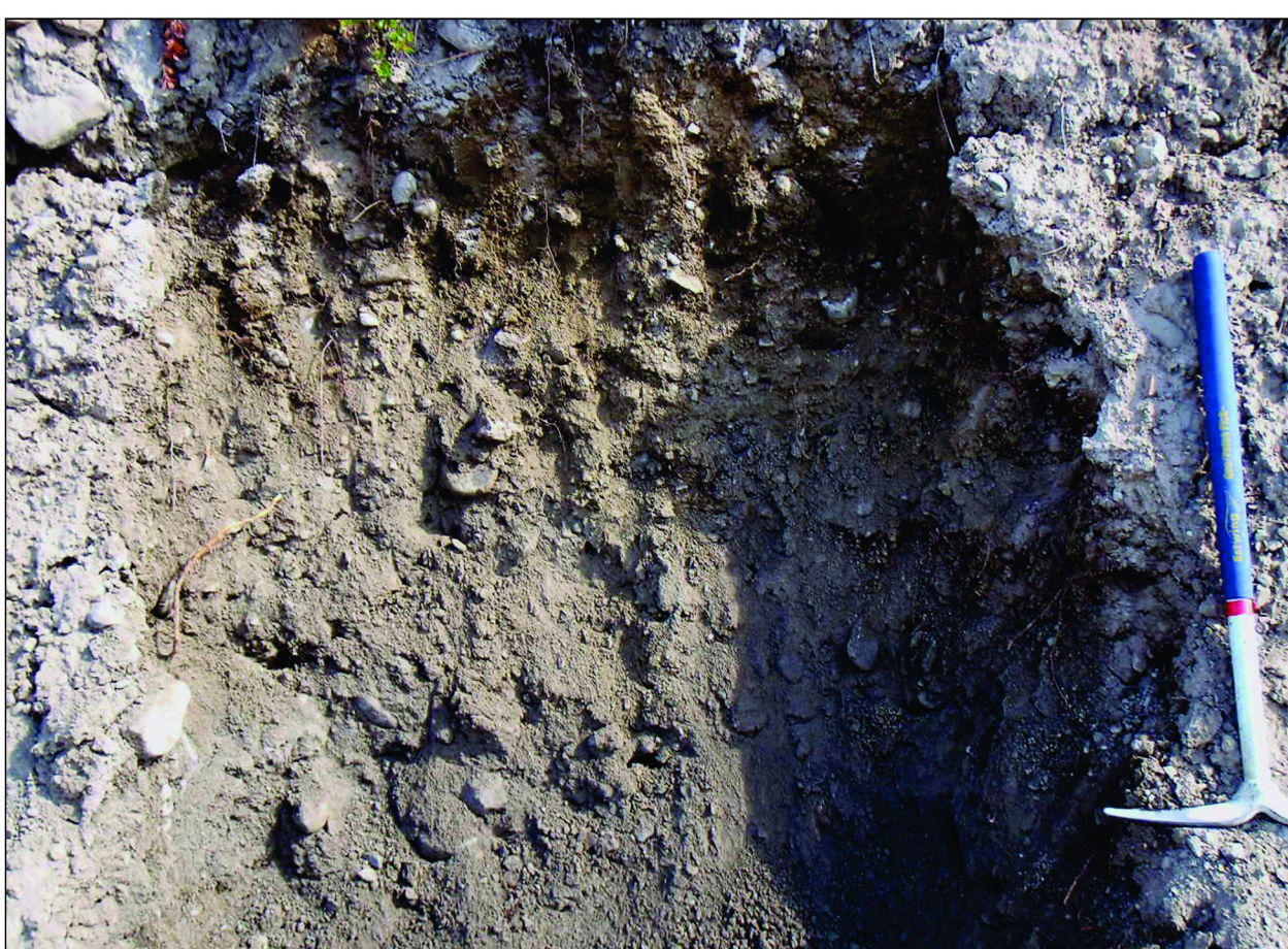
Figure 3. Ablation till exposed in road cut (65 cm pick for scale both photos). There is a higher percentage of sand and gravel, compared to typical basal till (see Figure 2), and lower density.
