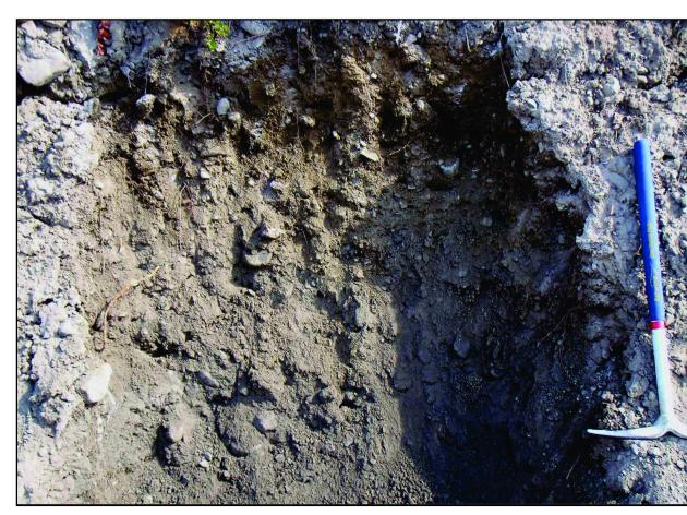
Fig. 3. Ablation till exposed in road cut with higher percentage of sand and gravel, and lower density, compared to typical basal tills (see Fig. 2). Pick for scale (65 cm).
