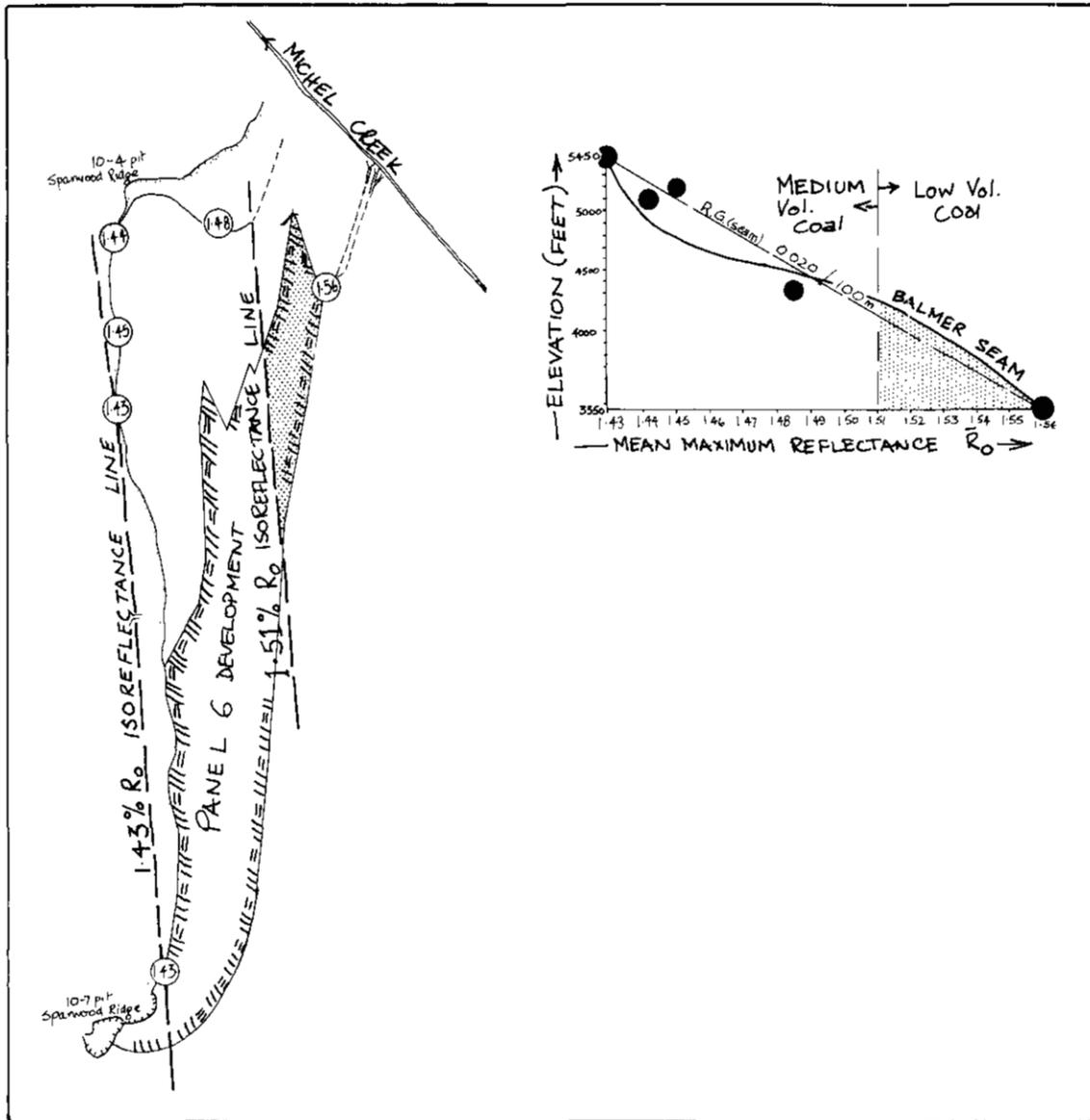
Figure 12. Coalification map of Balmer seam over the 'Panel 6' development with location of petrographic samples, location of isorank lines, and cross-section of Balmer seam showing rank change with elevation.
