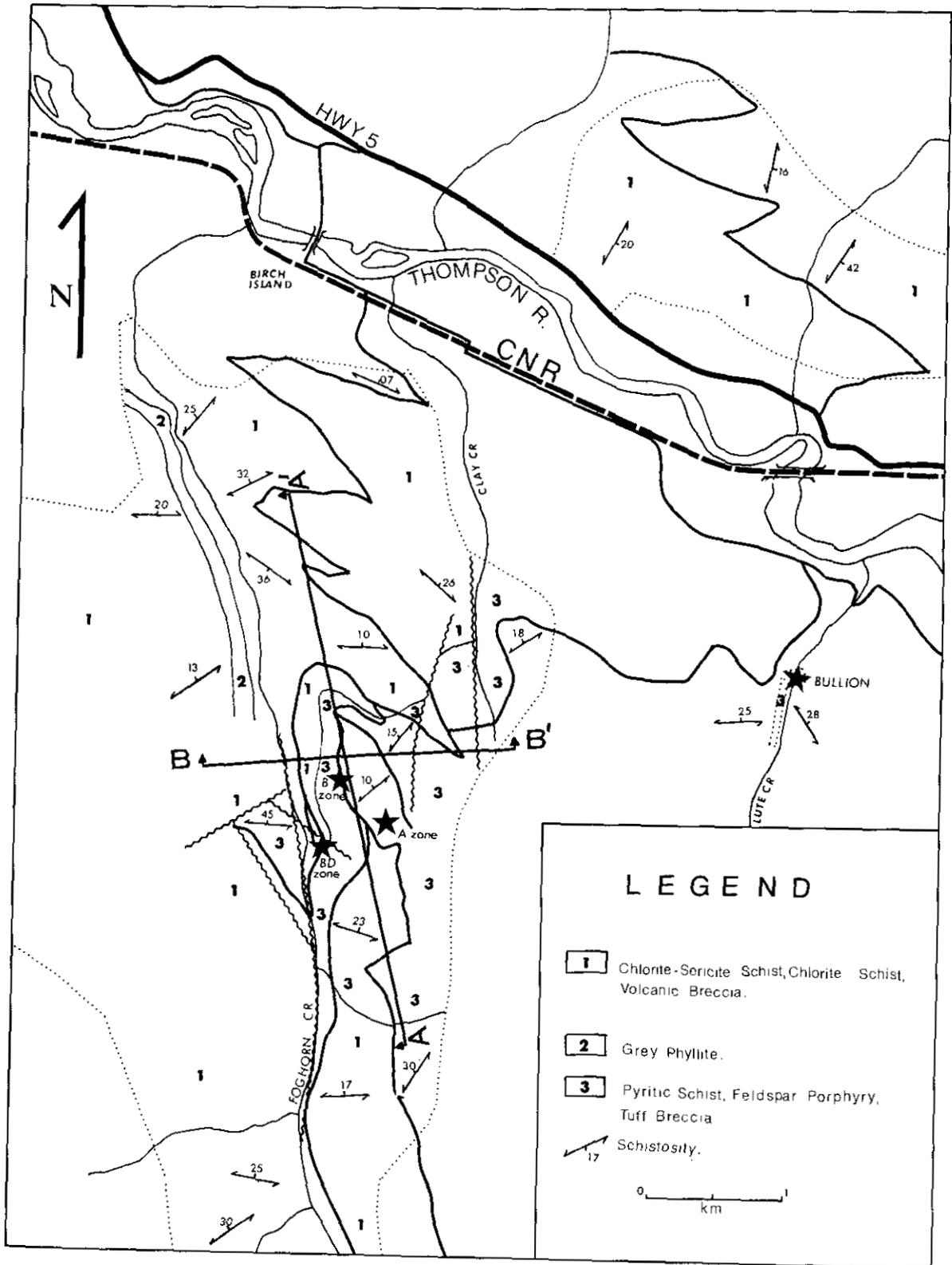
Figure 3. Generalized geology of the Rexspar property.
