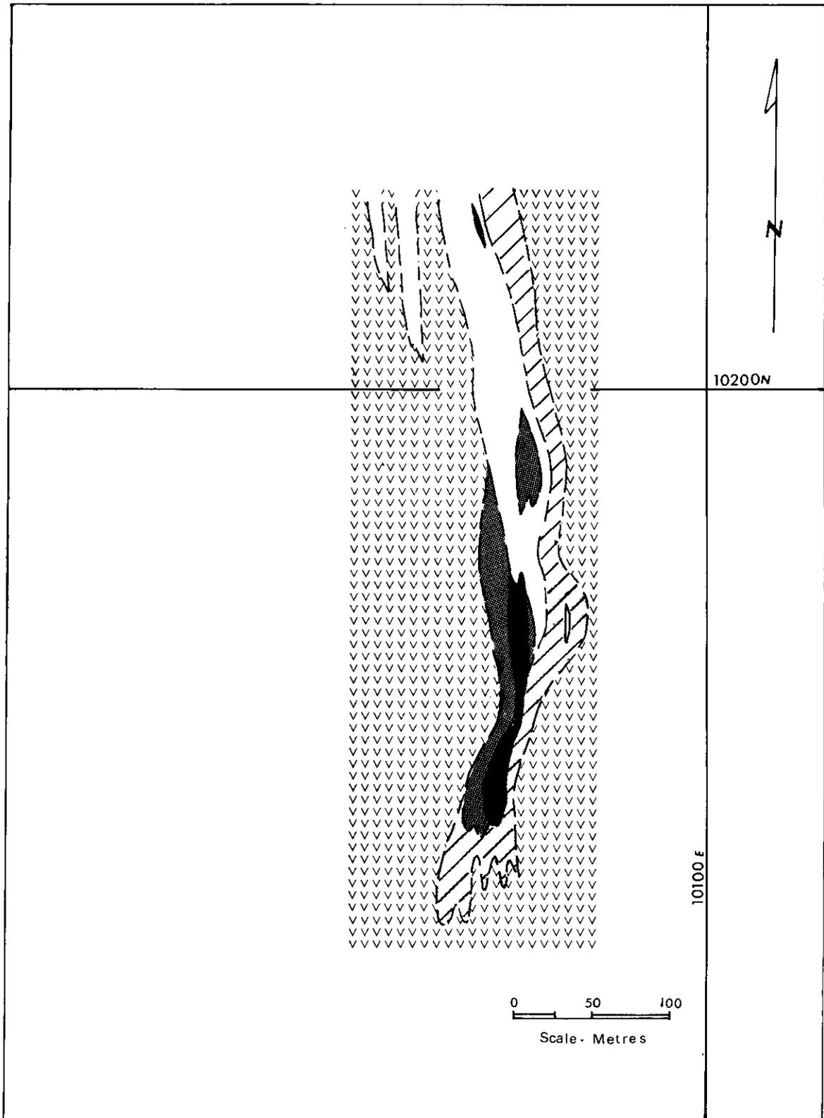
Figure 11b. CC property, plan view of geology and alteration at elevation 1 750 metres (based on projections from drill-hole information). For legend, see Figure 11a.
