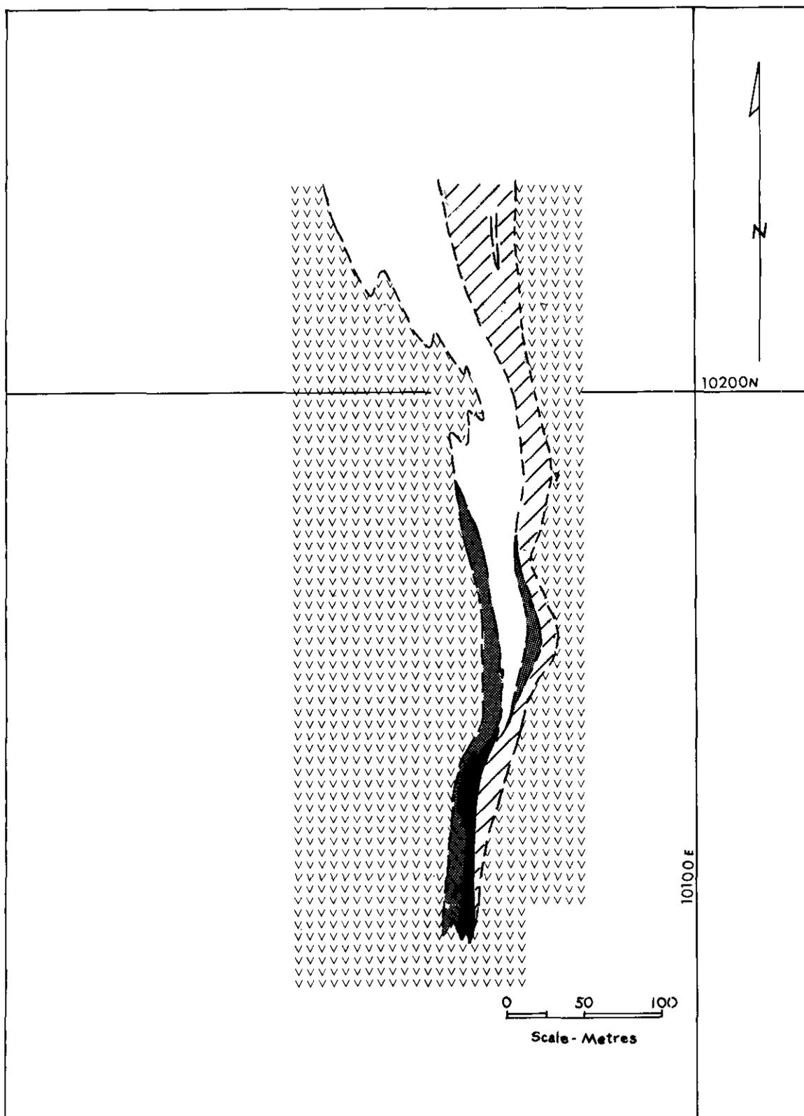
Figure 11c. CC property, plan view of geology and mineralization at elevation 1 700 metres (based on projections from drill-hole information). For legend, see Figure 11a.
