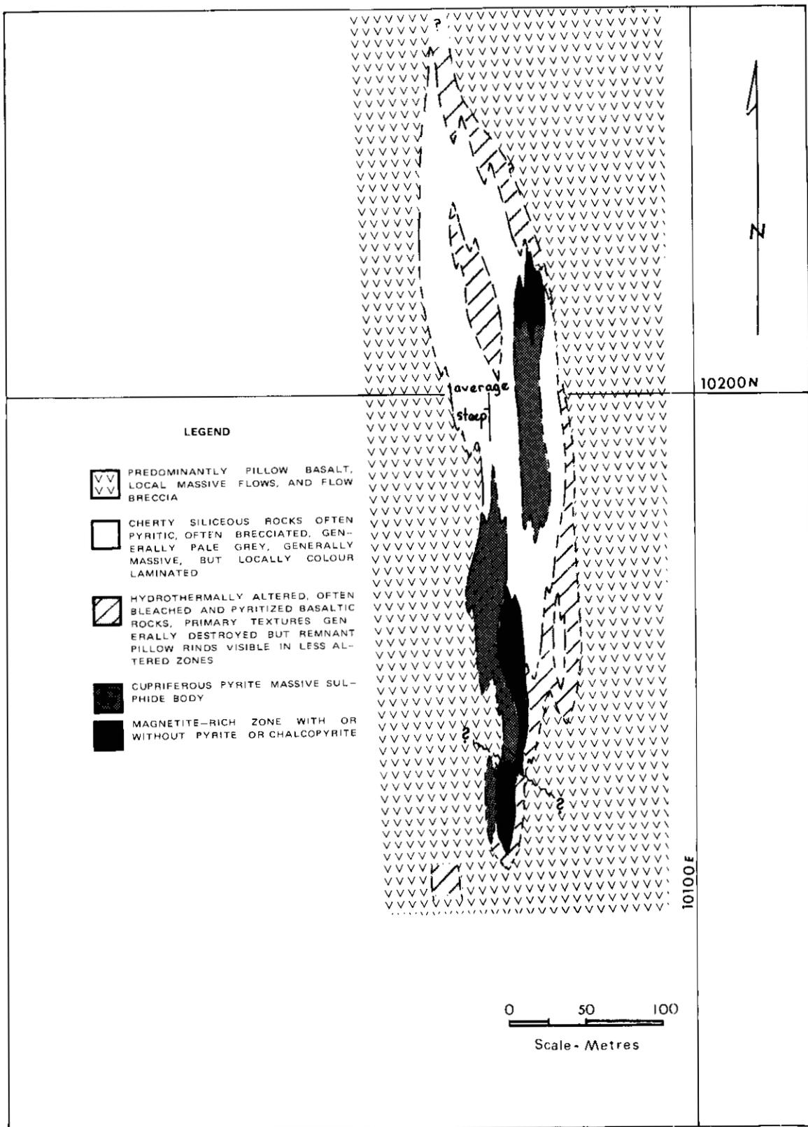
Figure 11a. CC property, plan view of geology and mineralization at elevation 1 800 metres (based on projections from drill-hole information).
