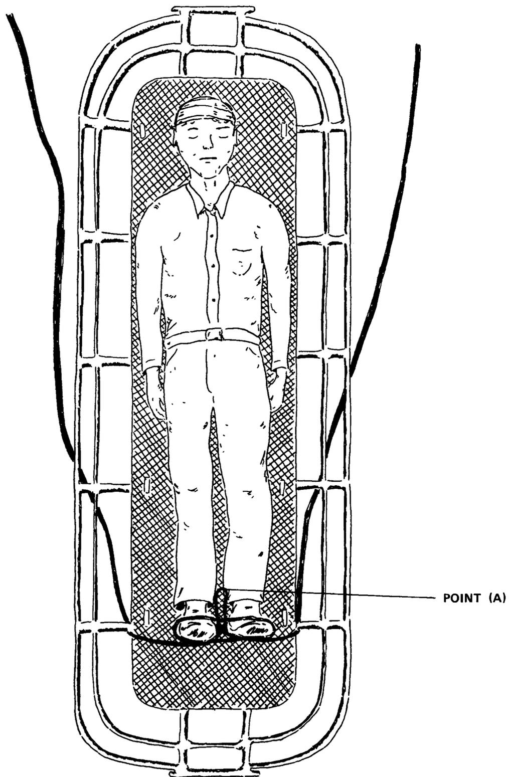
**STEP 2:** Grasp rope at Point (A) and pull slack to make loop approximately 6 inches long running loop between feet as shown.
