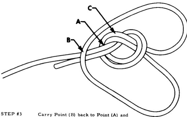
**STEP #3** Carry Point (B) back to Point (A) and hold under thumb of left hand as shown in Step #3. Grasp double rope at Point C and pull up through thumb knot as in Step #4.
