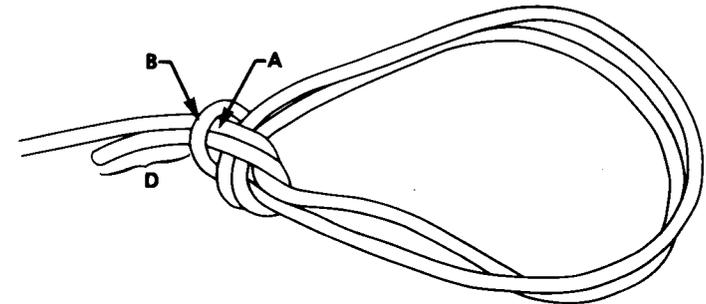
**STEP #5** With completed knot, you should be left with two equal loops as long as you have held the rope secure with no slippage where Point (B) crosses over Point (A). Note dead end of rope at Point (D) should be at least 12" long.
