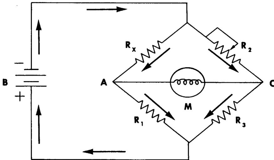
1. Resistor  $R_1$  is the reference element. It is a fixed resistor, but its value will vary slightly with atmospheric temperature. It is mounted near the sensing element to compensate for atmospheric effects upon  $R_x$ .
