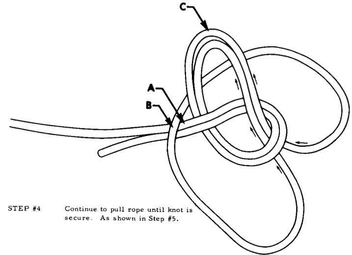
**STEP #4** Continue to pull rope until knot is secure. As shown in Step #5.
