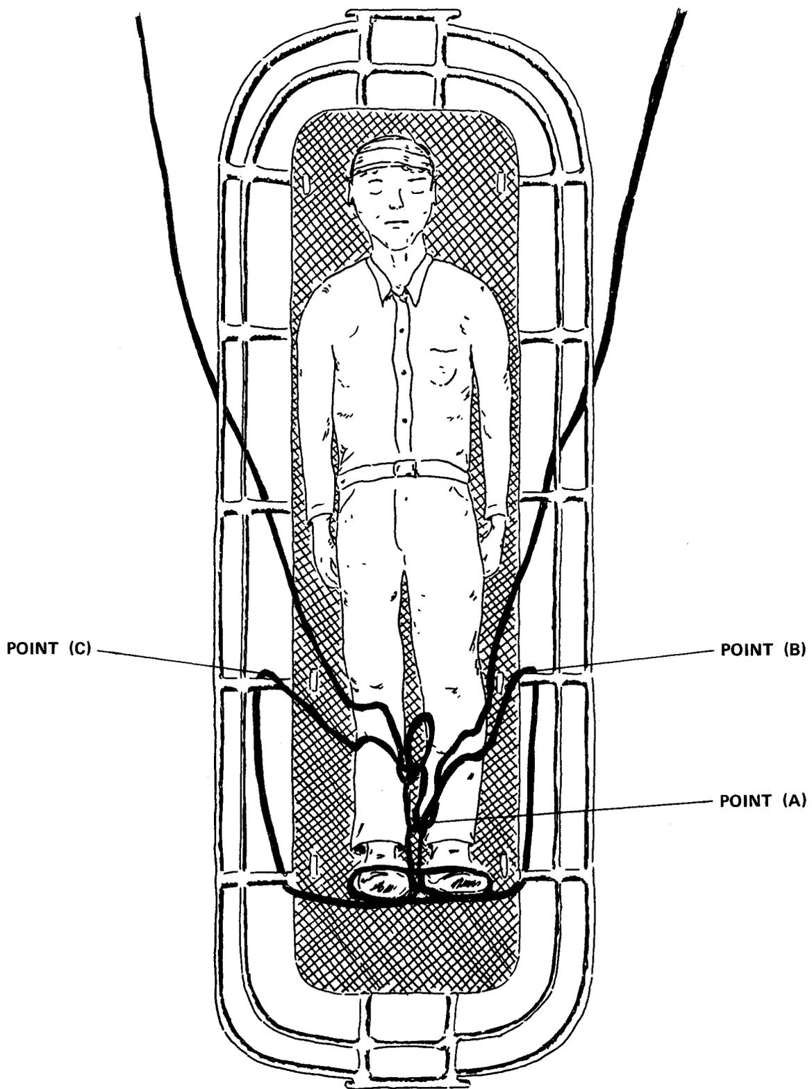
**STEP 3:** Grasp rope at Point (B) pulling enough slack to form loop and passing it through loop and passing it through loop at Point (A) doing the same at Point (C) keeping rope under bottom bar of stretcher at all times.
