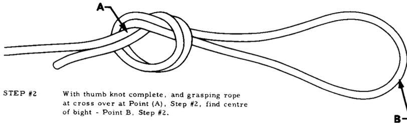
**STEP #2** With thumb knot complete, and grasping rope at cross over at Point (A), Step #2, find centre of bight - Point B. Step #2.
