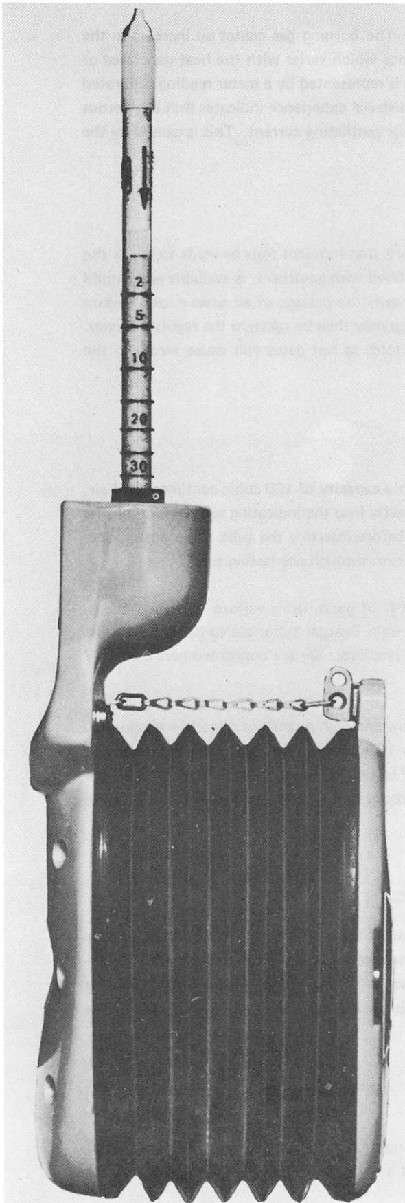
Fig. 1 Multi Gas Detector ready for use
