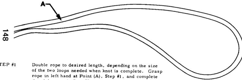
**STEP #1** Double rope to desired length, depending on the size of the two loops needed when knot is complete. Grasp rope in left hand at Point (A), Step #1, and complete thumb knot as in Step #2.
