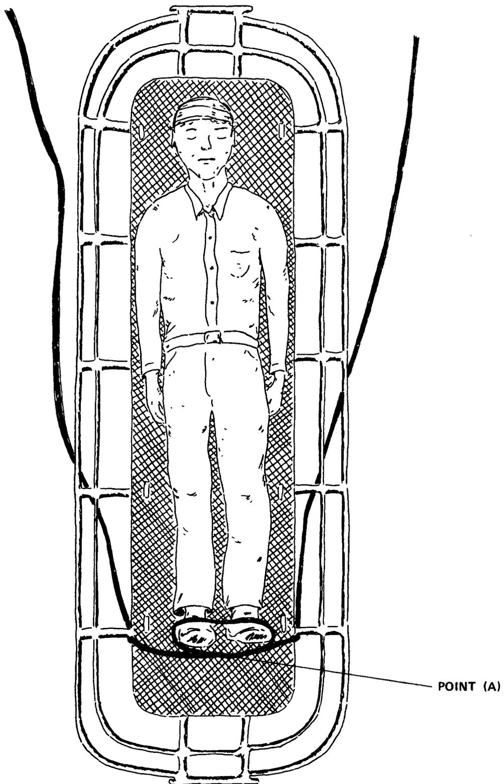
**STEP 1:** Thread rope at least 60 feet in length through bottom section of stretcher under lower bar, and take rap around both feet. Centre of rope should be at Point (A).
