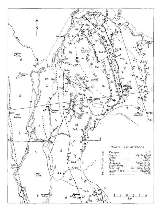
Figure 1. Generalized geological map of the Clearwater-Chu Chua area.
