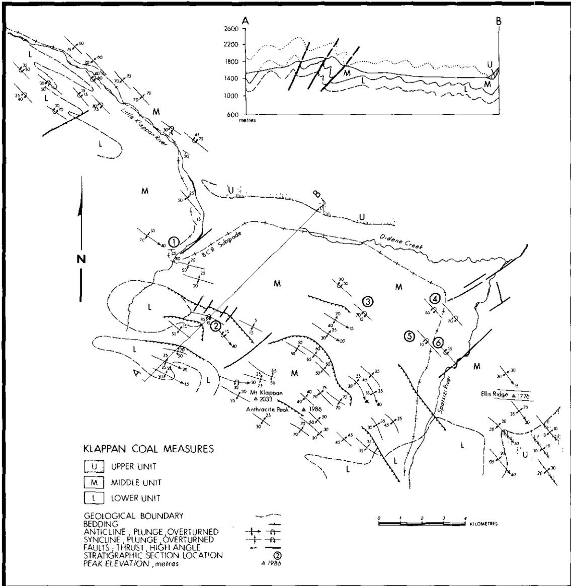
Figure 32. Simplified geology of the Mount Klappan area.
