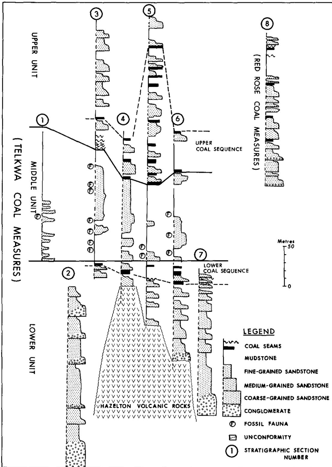
Figure 31. Stratigraphic sections of the Telkwa and Red Rose coal measures.
