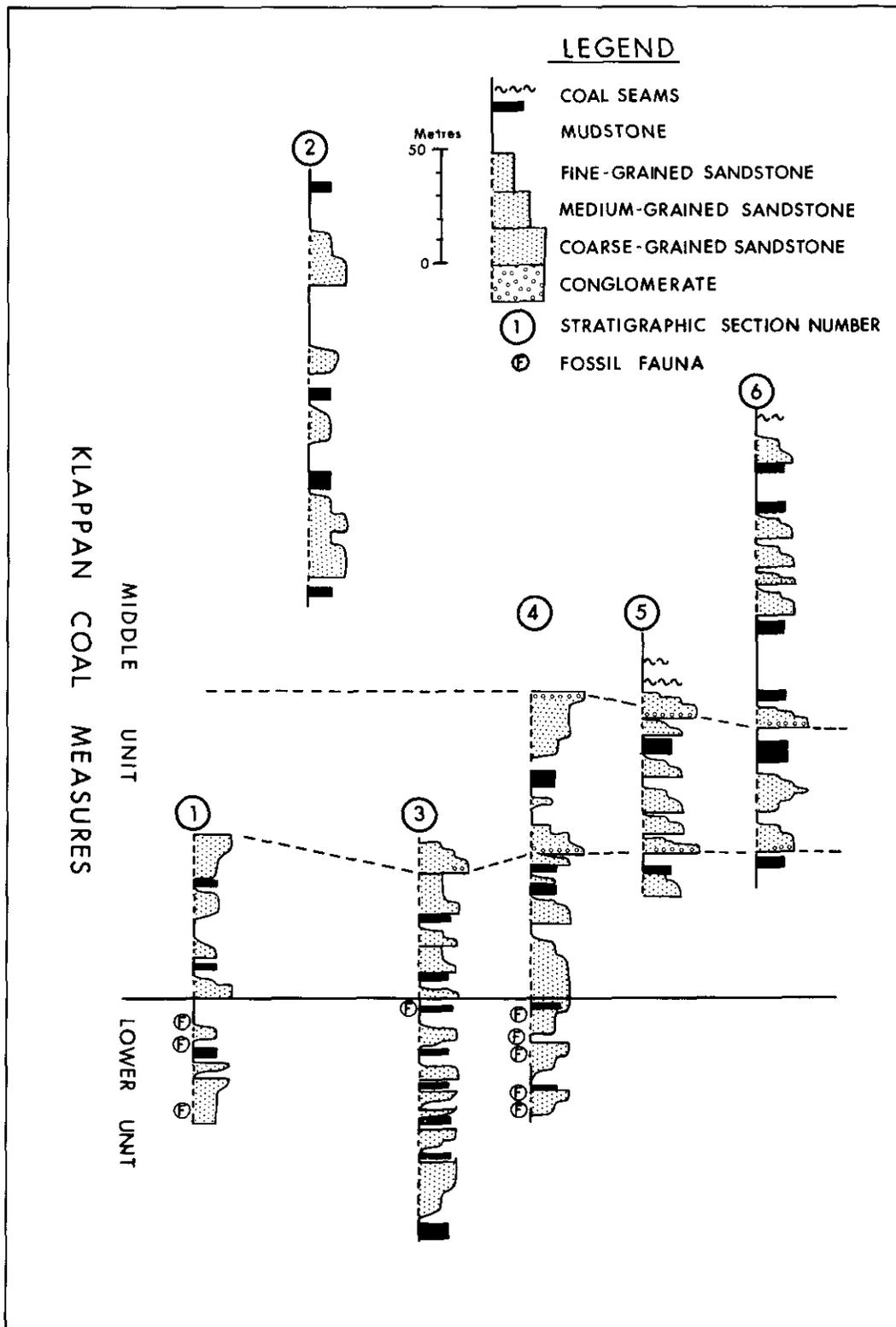
Figure 33. Stratigraphic sections of the Mount Klappan coal measures.
