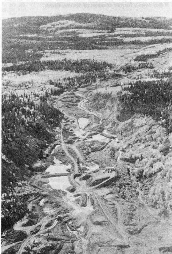
View to southwest downstream along McKee Creek. The steep faces of early hydraulic mining cuts are visible along both sides of the creek. The present operation of Eldorado McKee Mining is in the foreground, while the operation of ABC Mining is in the centre of the picture. Atlin Lake is in the background.
