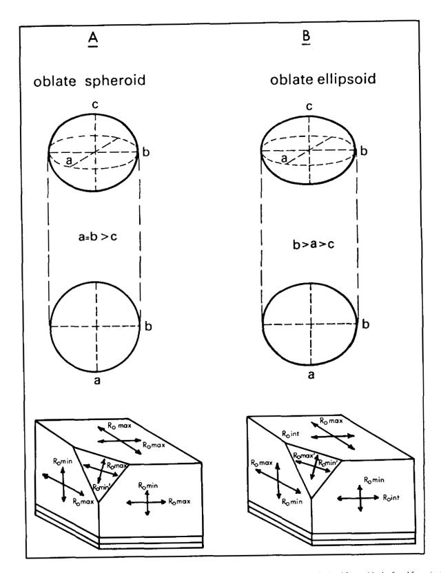
Figure 19-1. Reflectance indicatrix shapes and corresponding reflectance readings which may be obtained from a block of coal for uniaxial (a) and biaxial (b) coals.
