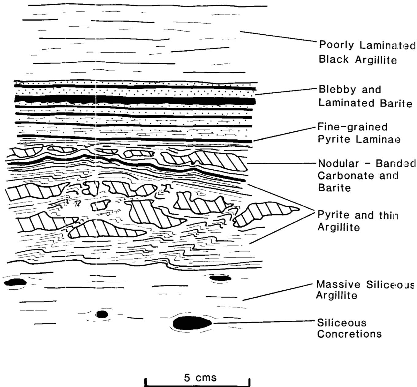
Figure 53-7. Detailed lithological section through a rhythmic cycle within TH, showing chemical differentiation with laminated sulphides at the base passing upward into massive barite and nodular carbonate. The top of the unit is characterized by sulphide-poor, laminated to blebby barite.
