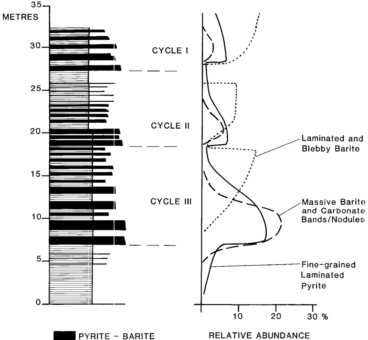
Figure 53-8. Logged section through TH mineralization showing three rhythmic cycles. Variations in the relative abundance of the three principal components are also shown.
