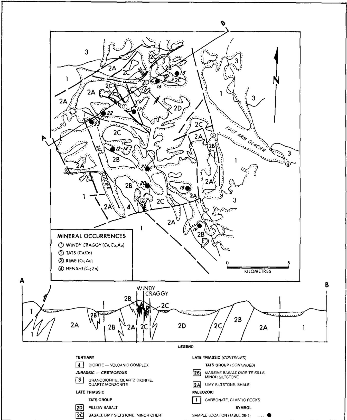
Figure 28-5. Geology and sample locations, Windy-Craggy area. Geology after MacIntyre (1984).
