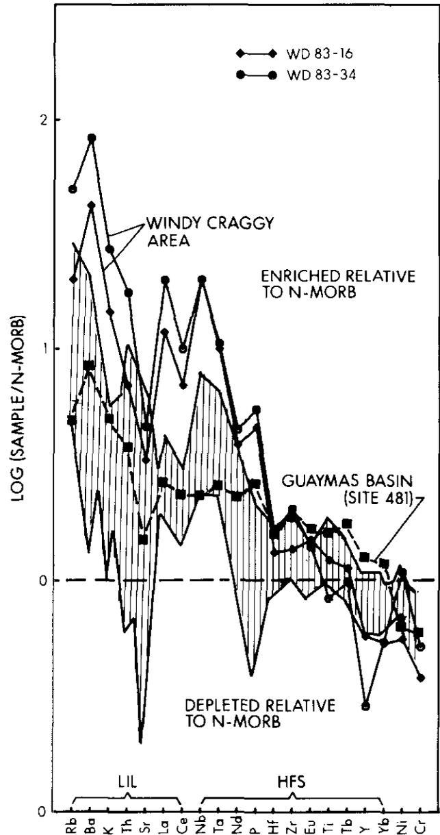
Figure 28-16. Plot showing variation of large ion lithophile (LIL) and high field strength (HFS) elements for samples from the Windy-Craggy area normalized against typical MORB concentrations (see Table 28-2). Also shown for comparison is the range of values for samples from the Chilkat Peninsula, Taku terrane (Davis and Plafker, 1985), and a sample of basalt from the Guaymas Basin of the Gulf of California. Plot after Saunders and Tarney (1984).
