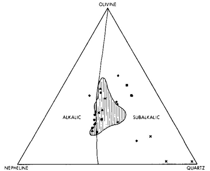
Figure 28-9. Normative olivine-quartz-nepheline ternary plot showing alkalic and subalkalic fields as defined by Irvine and Baragar (1971). See Figure 28-7 for explanation of symbols.
