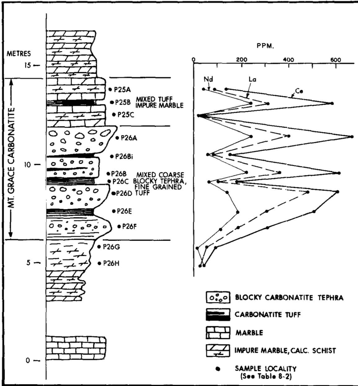
Figure 8-7. Detailed section of the Mount Grace carbonatite, Blais Creek (stations H85P25 and H85P26), showing La, Ce, and Nd values of selected samples.
