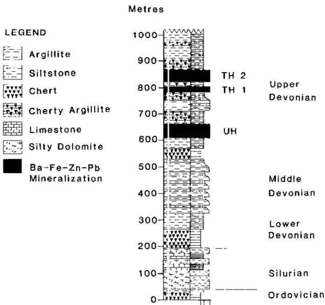
Figure 53-4. Stratigraphic column for the Driftpile Creek area.
