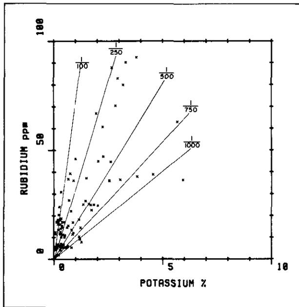
Figure 20-9. Cross-plot showing the relationship between Rb and K<sub>2</sub>O content. Rubidium/potassium ratios are also displayed.
