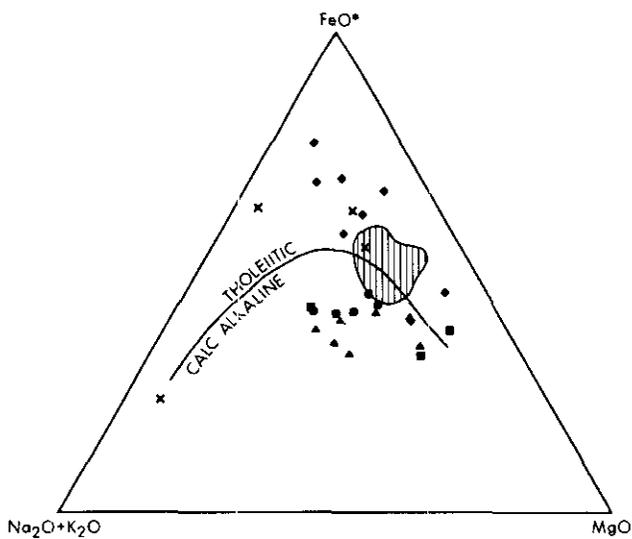
Figure 28-12. Alkalies-total iron as FeO-MgO ternary plot showing calc-alkaline and tholeiitic fields. See Figure 28-7 for explanation of symbols.
