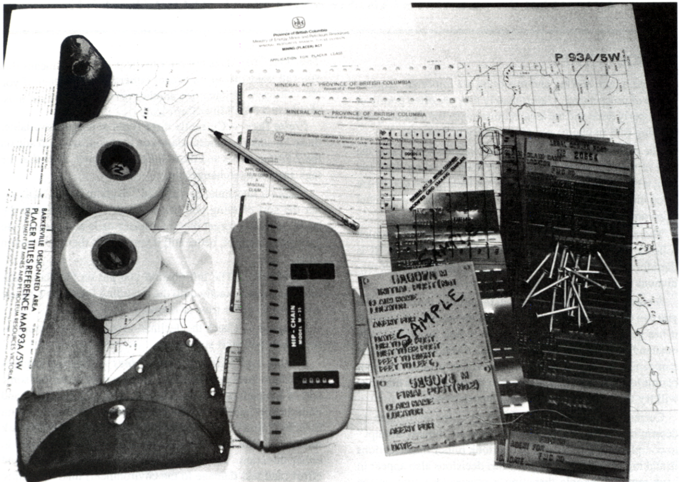
Figure 9-1. Examples of field equipment for staking. (Underneath; a claim map and the right forms! From left: hand axe; plastic flagging; an old ball-point pen for marking claim tags — you can also use a nail; belt or hip chain; 2-Post, Placer and Modified Grid claim tags; a plastic template for plotting claims; the all-important nails!)
