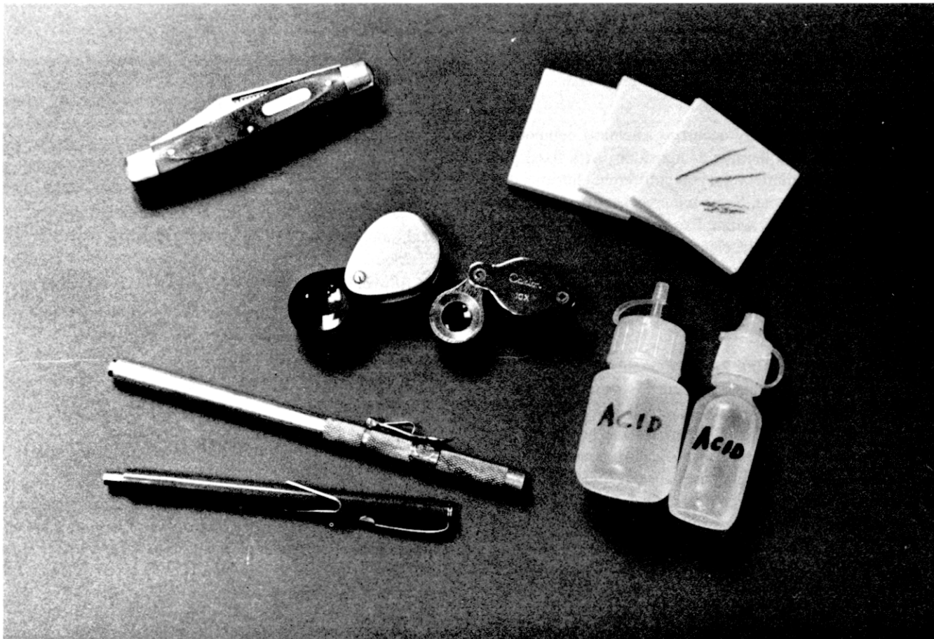
Figure 1-1. Basic equipment for mineral and rock identification. (Clockwise from top left: penknife; streak plates; two styles of acid bottle; two popular types of pencil magnet. Centre: two low-cost \times 10 hand lenses.)
