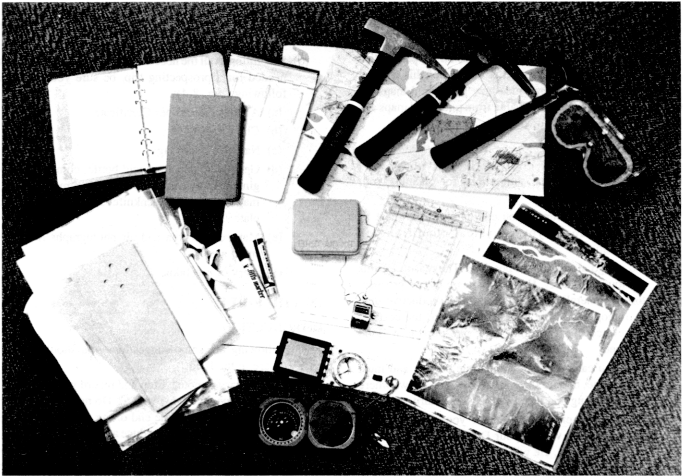
Figure 8-4. Examples of field equipment for prospecting. (Underneath: topographic and geologic maps. Clockwise from top left: three styles of field notebook; geologic hammers — pick and chisel type with fibreglass handles, all-steel chisel type; eye protection; air photos — one in a protective plastic cover; compasses — Silva above and Brunton below; plastic and cloth sample bags with a paper soil sample bag on top. Centre: felt-tip markers; first aid kit; two styles of protractor for plotting traverses; hand tally counter.)
