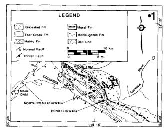
Figure 2-7-1. Regional geology of the Bend property, Cummins River canyon area (after Sirnony *et al.*, 1980). Geology is shown only for the area surrounding the North Road and Bend showings. The northwest-trending axis of the Porcupine Creek anticlinorium passes approximately through point 1.
