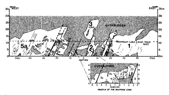
Figure 2-7-3. Profile of the Bend occurrence, Cummins River canyon. Zero on the vertical scale is the level of McNaughton Lake in June 1985; 11 metres is the maximum level of the lake. Unit numbers correspond to Figure 2-7-2.
