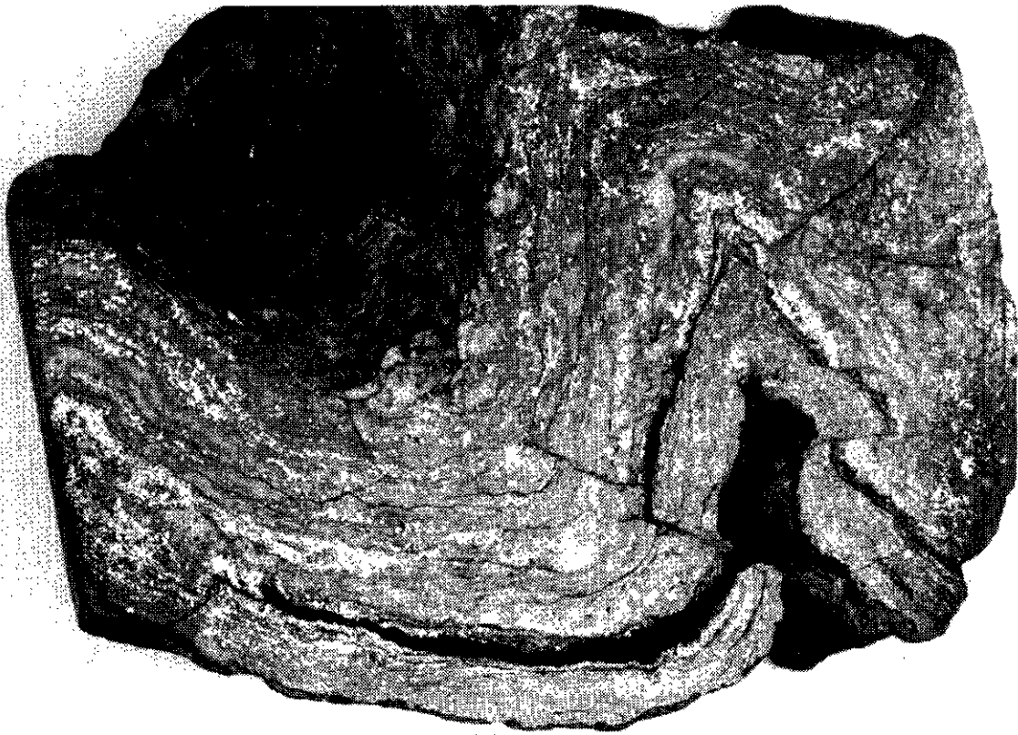
Plate 3-8-7. Folded quartz vein with bands of broken pyrite and chalcopyrite grains. Sample is from the Raven vein adit.
