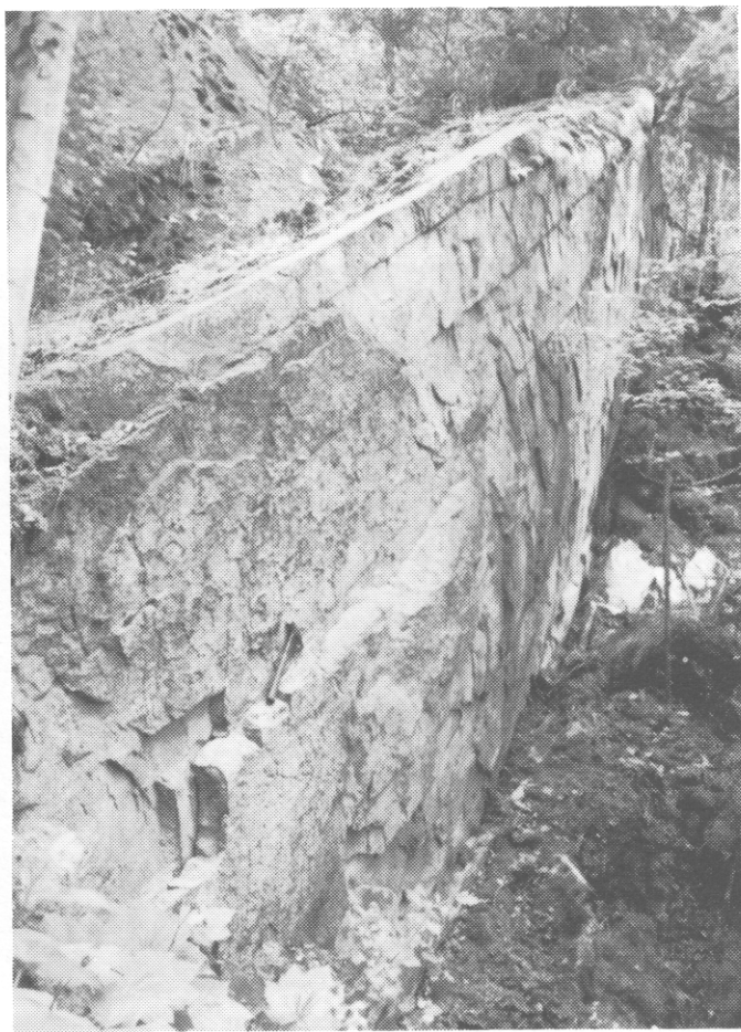
Plate 4-8-2. Three Mile Point quarry (82F/11W). Site 1. Note reserves of granodiorite and horizontal joints.
