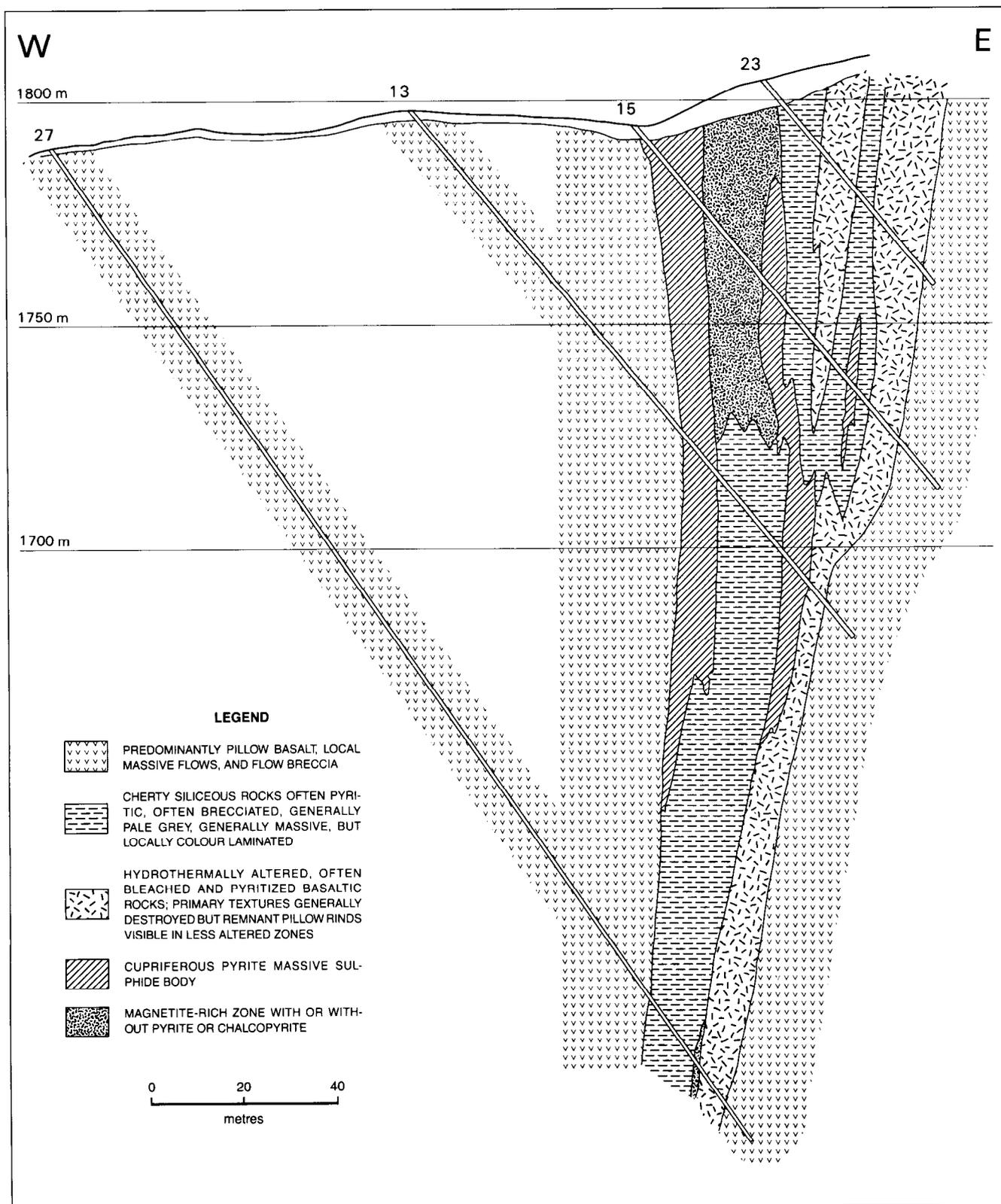
Figure 16. Cross-section through Chu Chua massive sulphide deposit, after McMillan (1980).
