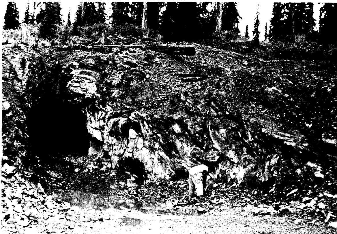
Plate 27. Exploration adit on the Spar (EX) lead-zinc-silver showing, Adams Plateau.
