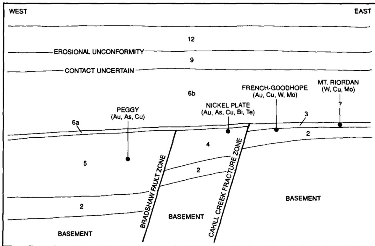
Figure 1-5-2. Schematic east-west stratigraphic section of the Hedley district showing location of skarn mineralization in relation to sedimentary facies changes (see Figure 1-5-1 for legend).
