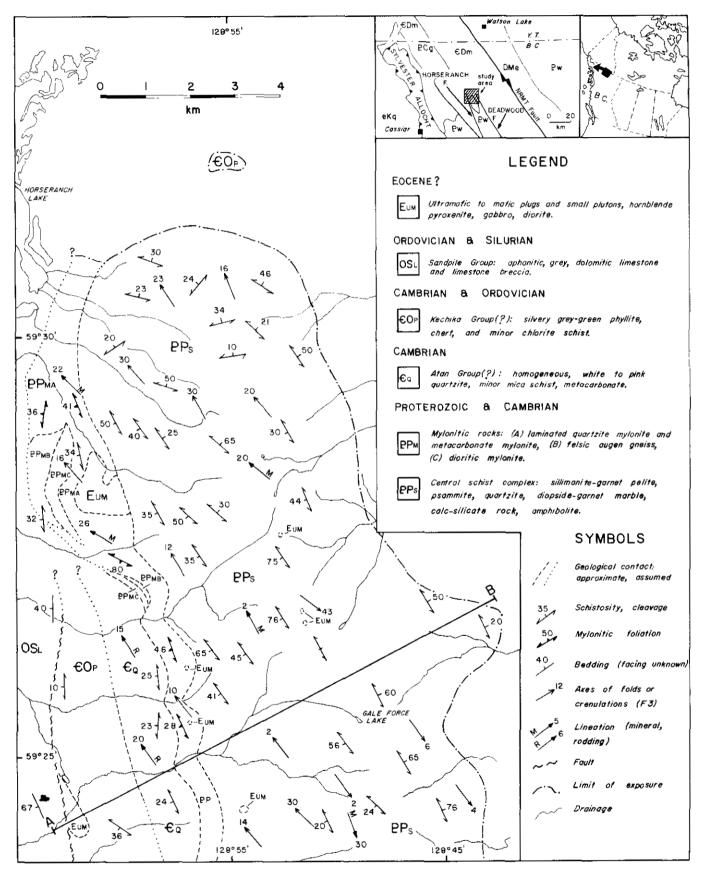
Figure 1-24-1. Geology of the northern Horseranch Range. Inset shows index map and regional geology. Line A-B is the location of the crosssection in Figure 1-24-2.
