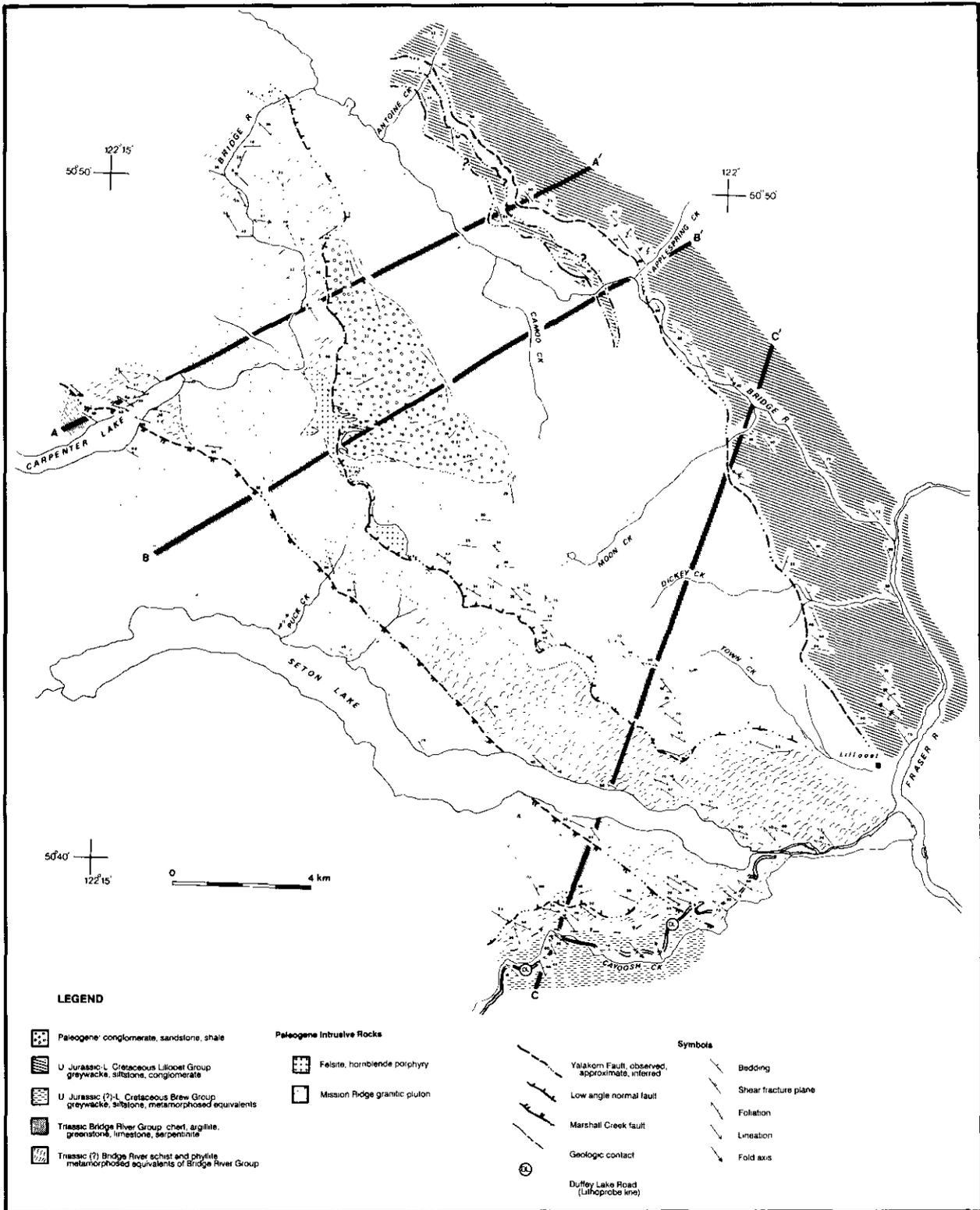
Figure 1-12-2. Geological map of Mission Ridge area. Local relief is more than 2200 metres and accounts for the arcuate trace of some of the major faults.
