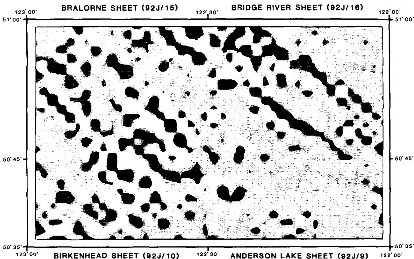
Figure 1-13-6. Double-derivative plot of the total magnetic field based on the G.S.C. regional magnetic Map 8548G – (blank area for values less than 500 /Mi<sup>2</sup> units, dark grey greater than 500 /Mi<sup>2</sup> units).
