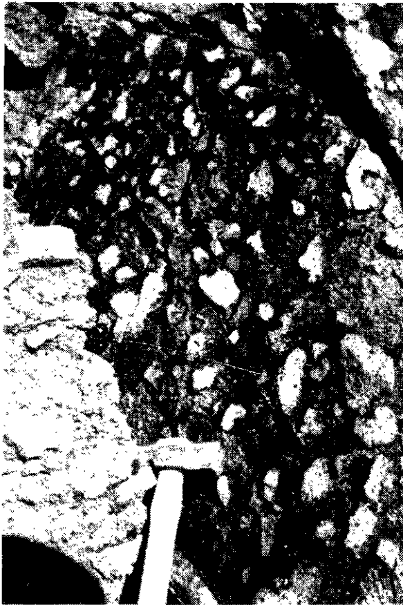
Plate 1-26-4. Typical, coarse-grained polymictic volcanogenic breccia. Fragments shown are of varied composition and texture.
