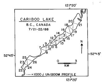
Figure 2-3-6. Cariboo Lake (Figure 2-3-1) showing location of 26 high-resolution seismic traverses.
