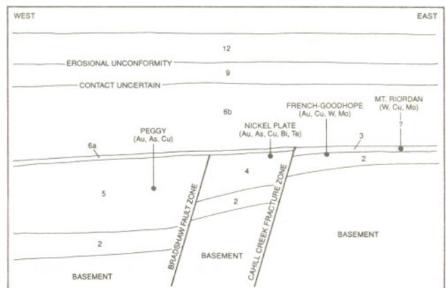
Figure 12. Schematic stratigraphic section of the Hedley district showing location of skarn mineralization in relation to sedimentary facies changes (after Ray *et al.*, 1988). See legend for Figure 11.
