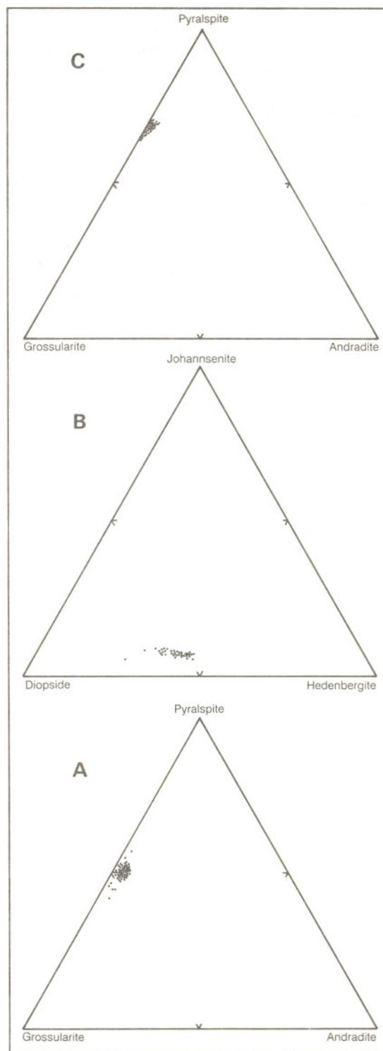
Figure 31. Composition of exoskarn garnets and pyroxenes from the PME skarns, Tillicum Mountain camp. (Analyses by G.E. Ray and G.L. Dawson at The University of British Columbia, Vancouver.)
