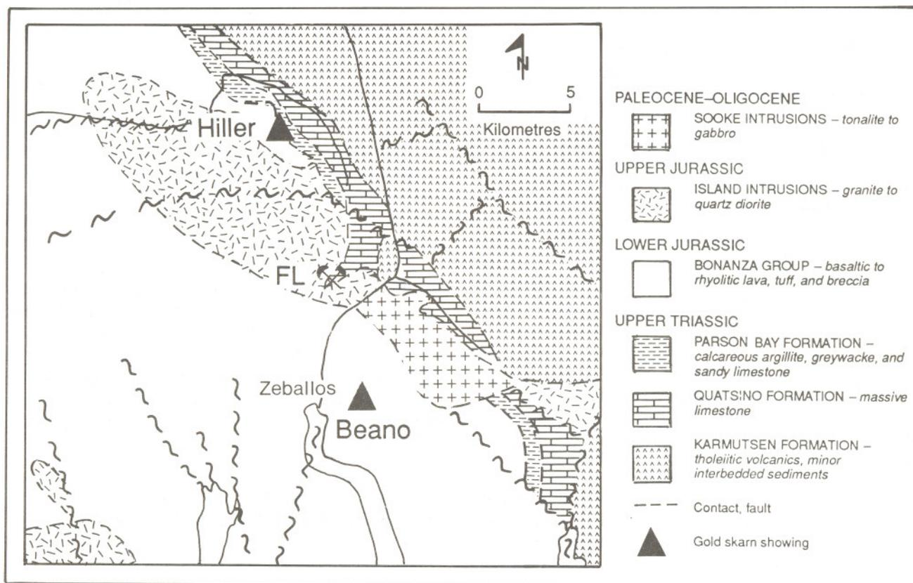
Figure 34. General geology of the Zeballos camp, Vancouver Island, and location of the skarn deposits. (Modified after Hoadley, 1953, and Falconbridge Limited, unpublished reports.)
