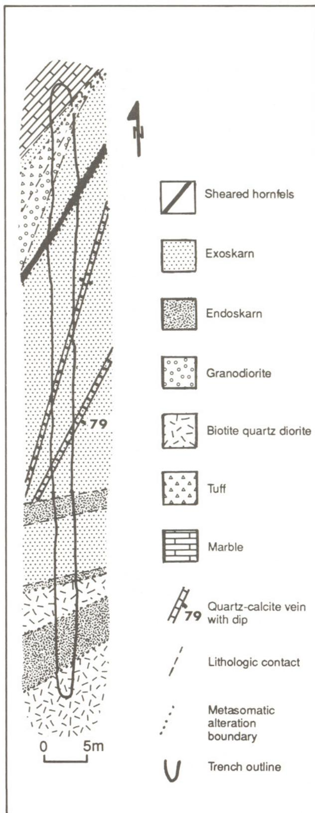
Figure 26. Geology of Trench No. 1, Iron Horse showing, Oka claims. (Geology by A.D. Ettlinger.)
