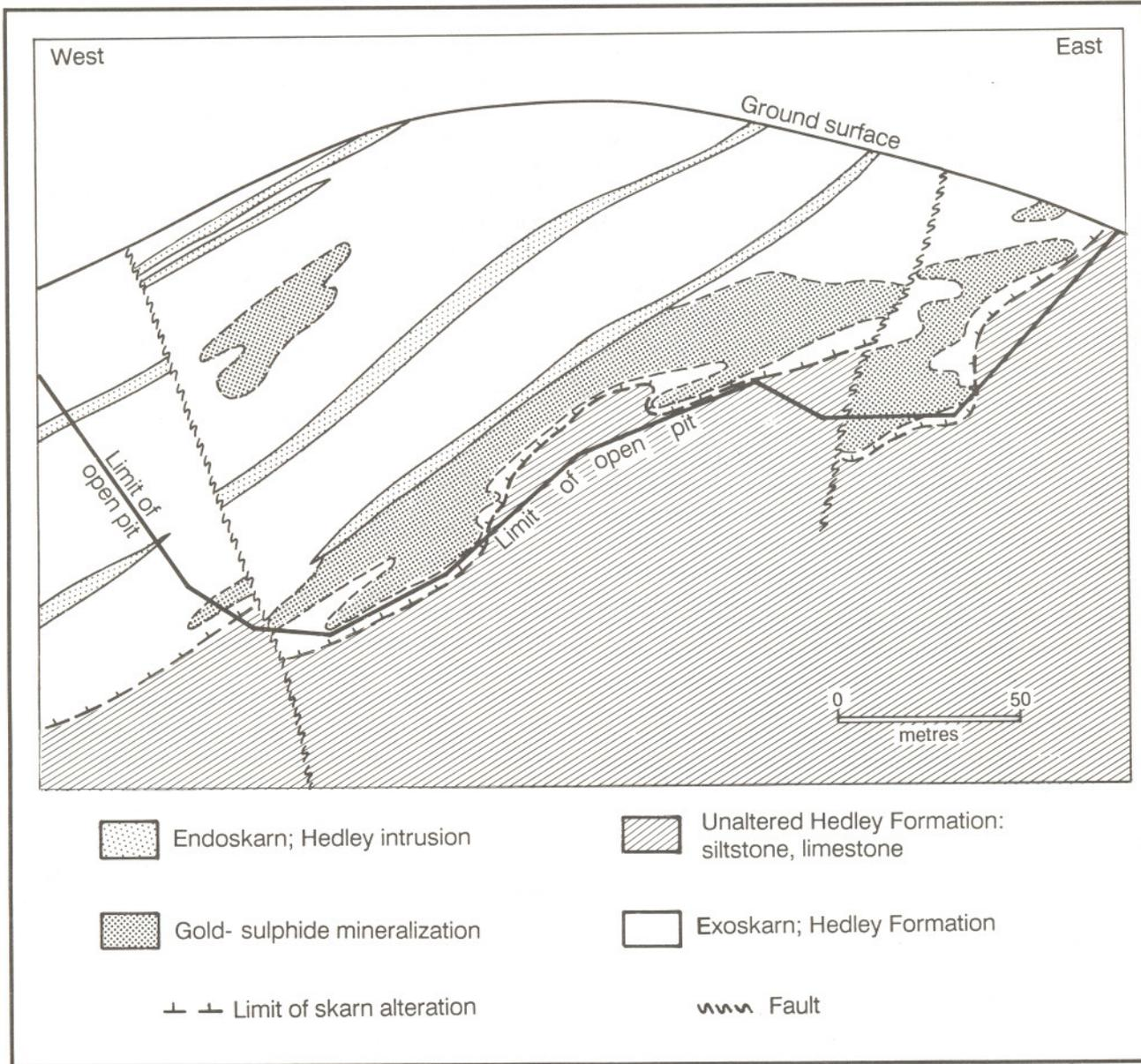
Figure 15. Generalized section through the southern part of the Nickel Plate deposit, Hedley camp. For location see Figure 14. (Compiled from Simpson, 1988 and unpublished reports and drill sections, courtesy of Mascot Gold Mines Ltd.)
