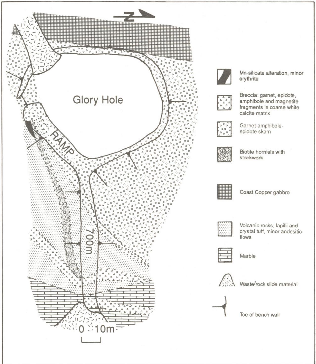
Figure 37. Geology of the Merry Widow mine glory hole, 700-metre level. (Geology by A.D. Ettlinger.)
