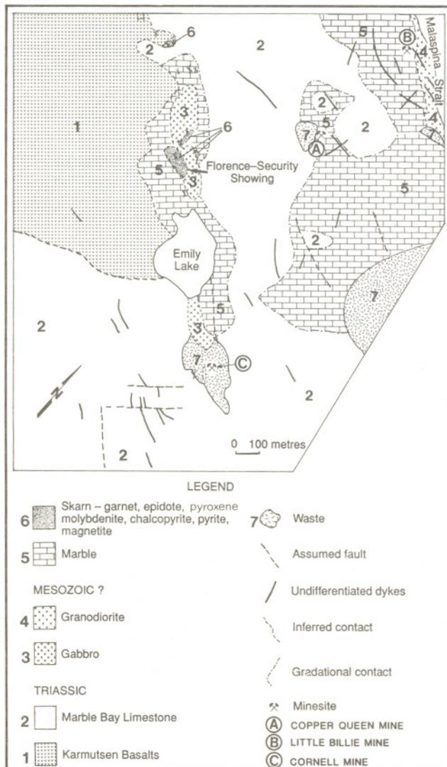
Figure 33. General geology of the Little Billie - Copper Queen mines area, Texada Island. (For location see Figure 32; geology by A.D. Ettlinger, courtesy of Vananda Gold Ltd.)
