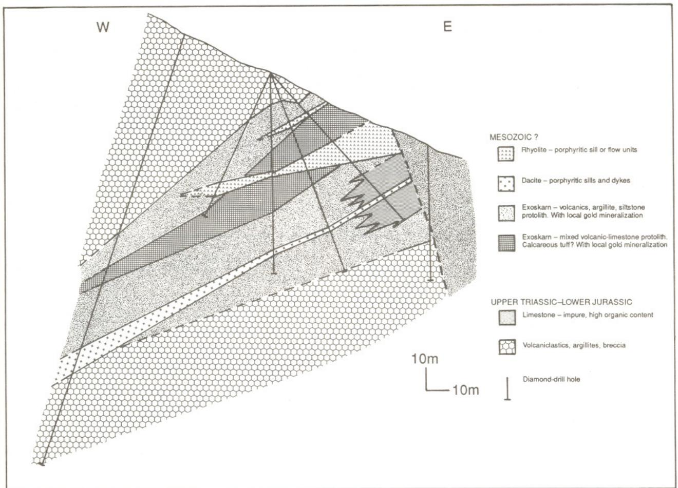
Figure 35. Geological cross-section through the Hiller (Artlish) PME skarn. (Compiled from drill-hole data logged by A.D.Ettlinger.)
