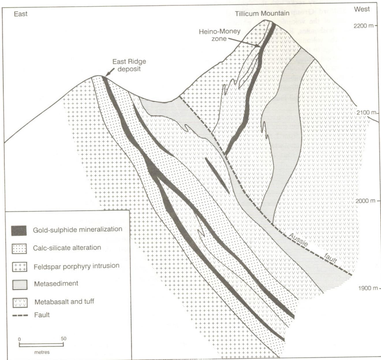
Figure 30. Schematic section through the Heino-Money zone and East Ridge deposit, Tillicum Mountain camp. (Modified from unpublished data, courtesy of Cordilleran Engineering Ltd.)
