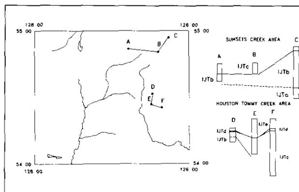
Figure 1-10-5. Stratigraphic sections illustrating unit thickness variations across the Thautil River map area. See legend Figure 1-10-2 for explanation of symbols.
