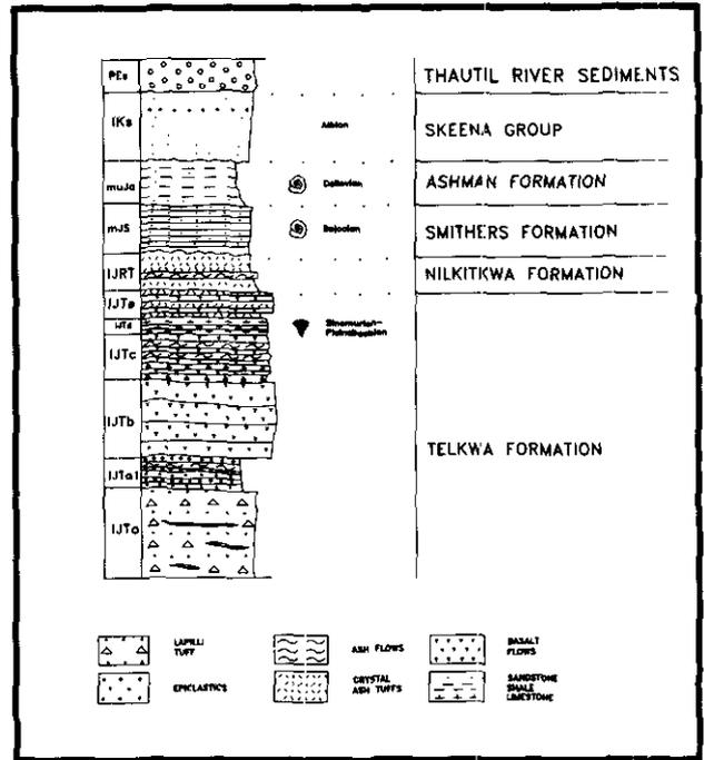
Figure 1-10-4. Generalized stratigraphic column for the Thault River map area. See legend Figure 1-10-2 for explanation of symbols.
