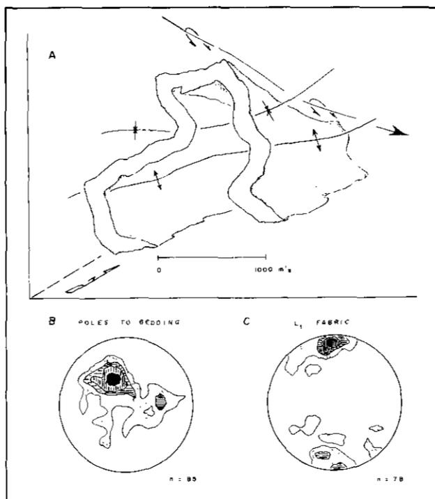
Figure 1-16-4. Isometric down-plunge projection through the Tatsamenie antiform (4A), stereographic equal-area contoured poles to bedding (4B) and contoured linear fabric (4c). Stereographic contour intervals are in area increments of 2%.
