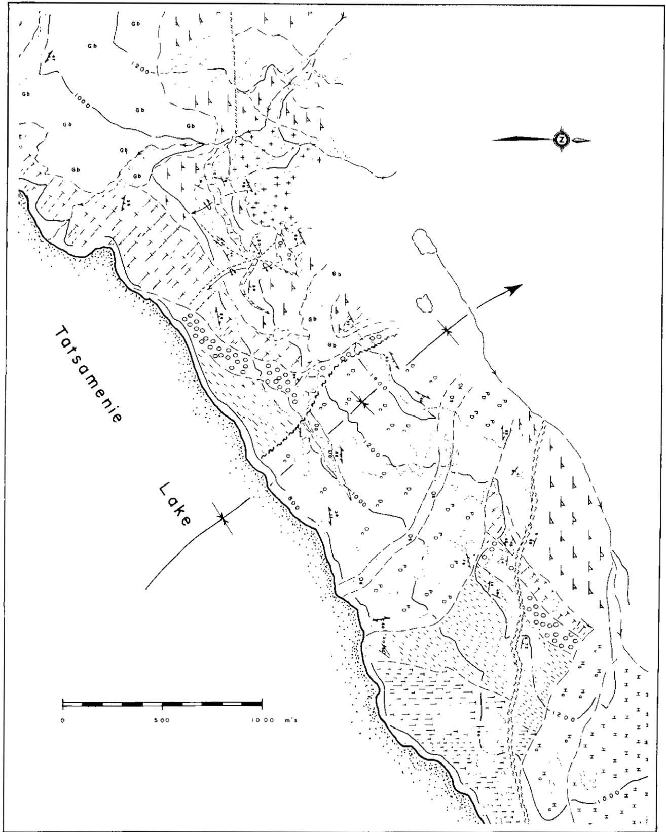
Figure 1-16-5. Geological plan of the Tatsamenie alteration zone. Lithologic patterns correspond to those of the stratigraphic column, Figure 1-16-2.
