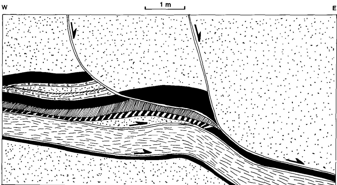
Figure 4-2-3. Extensional faults flattening into bedding plane shear zone in Comox No. 1 coalbed, Tsable River canyon.
