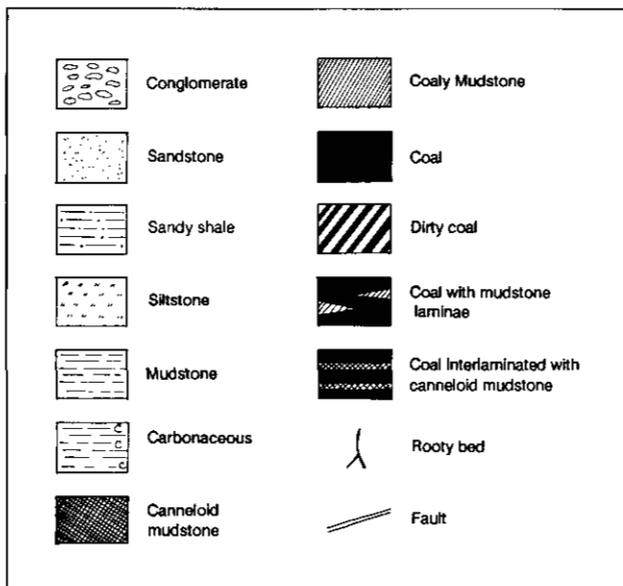
Figure 4-2-2a. Standard symbols for coal-measures sections.
