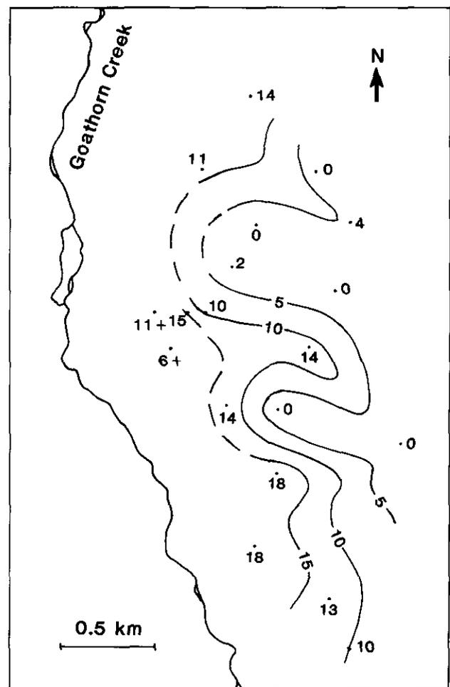
Figure 4-5-3. Isopach map (in metres) of three-sand, Telkwa coalfield.
