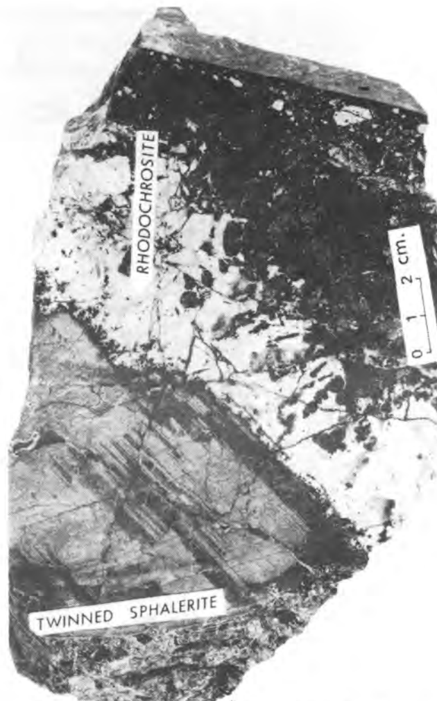
Plate 5.10. Polished section of ore sample from No. 4 vein of Wrinch vein system, showing large twinned sphalerite crystal (Silver Queen mine).
