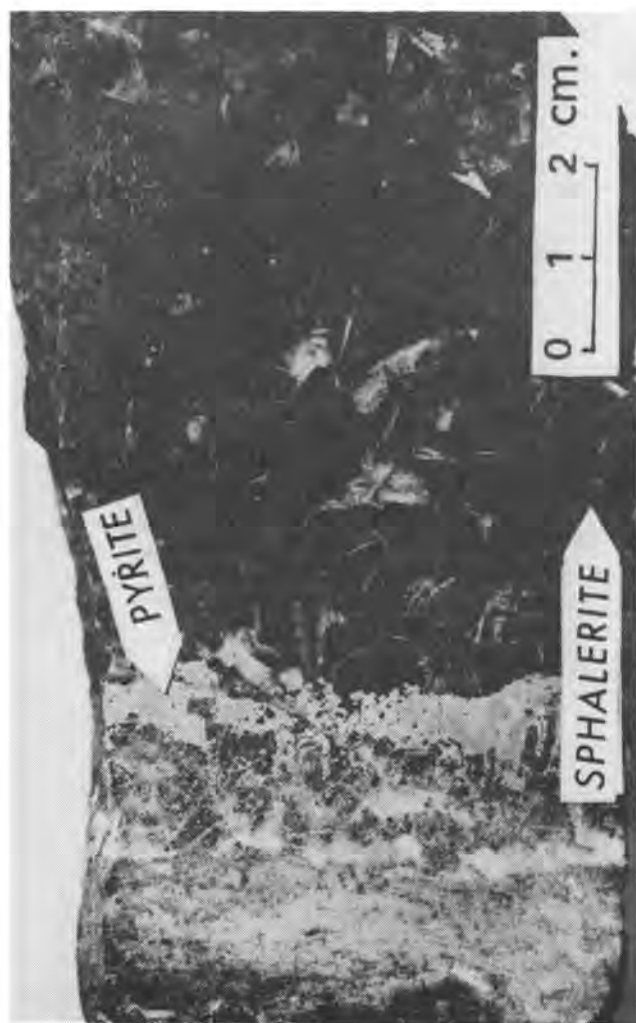
Plate 5.11. Polished section of ore sample from the Ruby extension of the Wrinch vein system, showing randomly arranged barite laths in sulphide matrix (Silver Queen mine).
