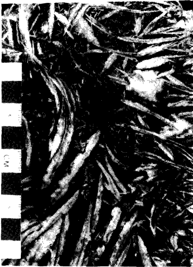
Plate 3-2-11. Magnesite pinolites (light grey) growing within a fine-grained dolomite matrix; Mount Brussilof mine.
