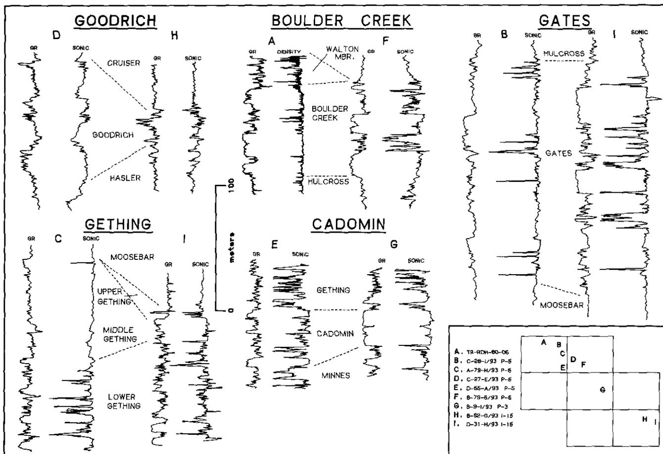
Figure 5-7-4. Geophysical log comparisons for Goodrich, Boulder Creek, Gates, Gething and Cadomin formations.
