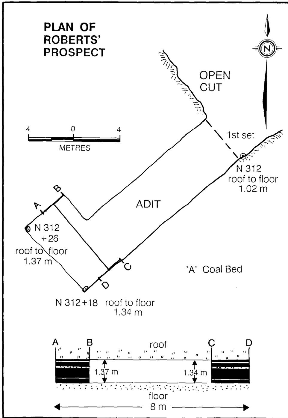
Figure 6. Plan view of Roberts Prospect, Chute Creek, with section through the face of the adit.
