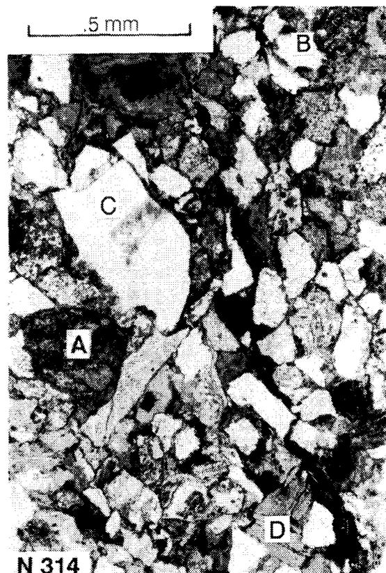
Plate 8. Photomicrograph of a Cumberland sandstone from Station N 314 (Figure 4); A - Volcanic rock fragment, B - Quartz, C - Plagioclase, D - Kaolinized feldspar.
