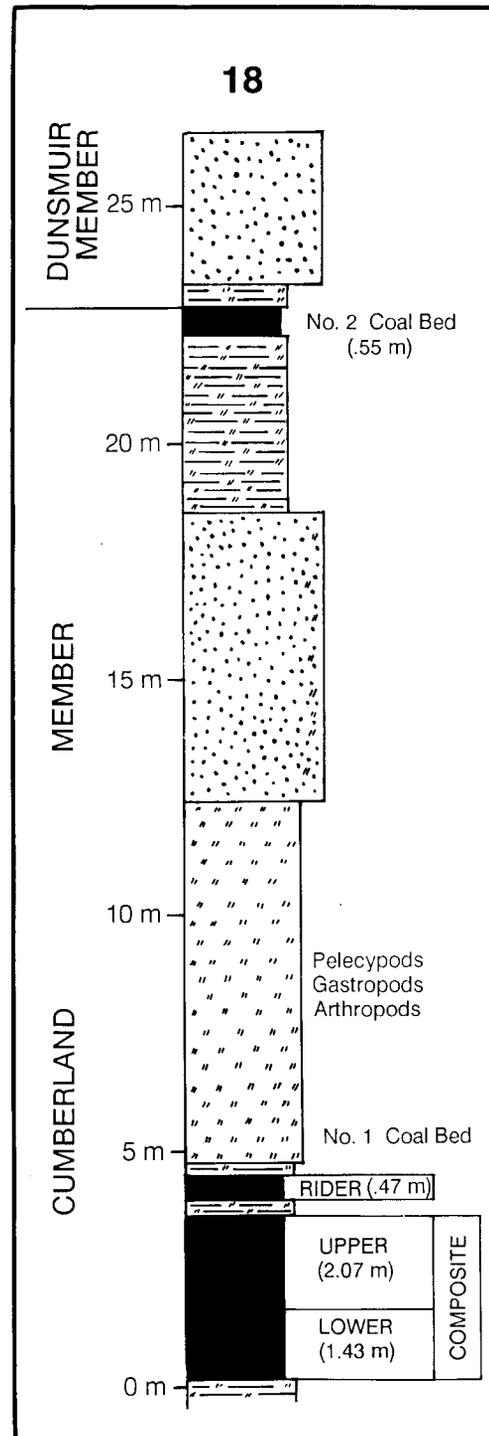
Figure 8. Section illustrating sample divisions for proximate analysis work from the Quinsam mine site, Station 18 (see Figure 7 for stratigraphic legend).
