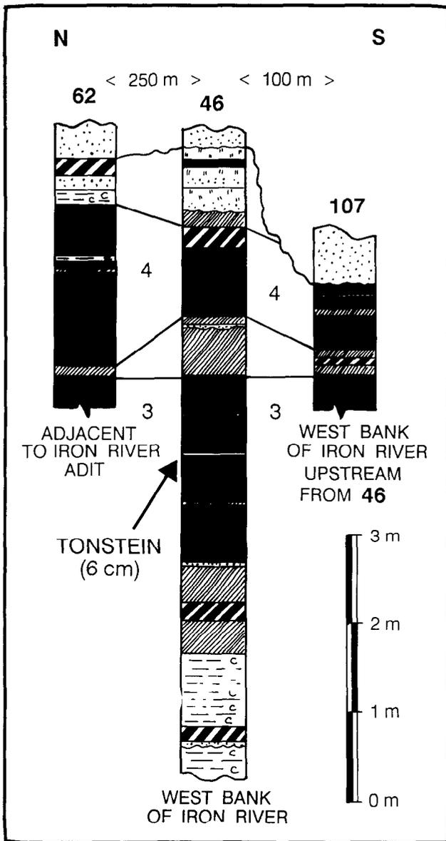
Figure 14. Detailed sections of coal beds No.3 and No.4 from the Quinsam area (see Figure 4 for station locations and Figure 7 for stratigraphic legend).
