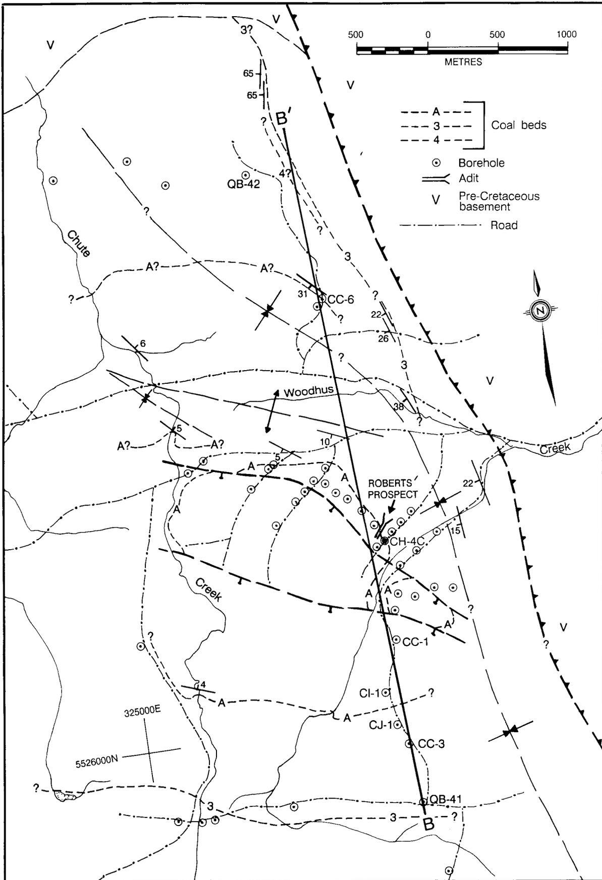
Figure 15. Locations of boreholes and adit used for interpretive cross-section in the Chute Creek area (see Figure 16).
