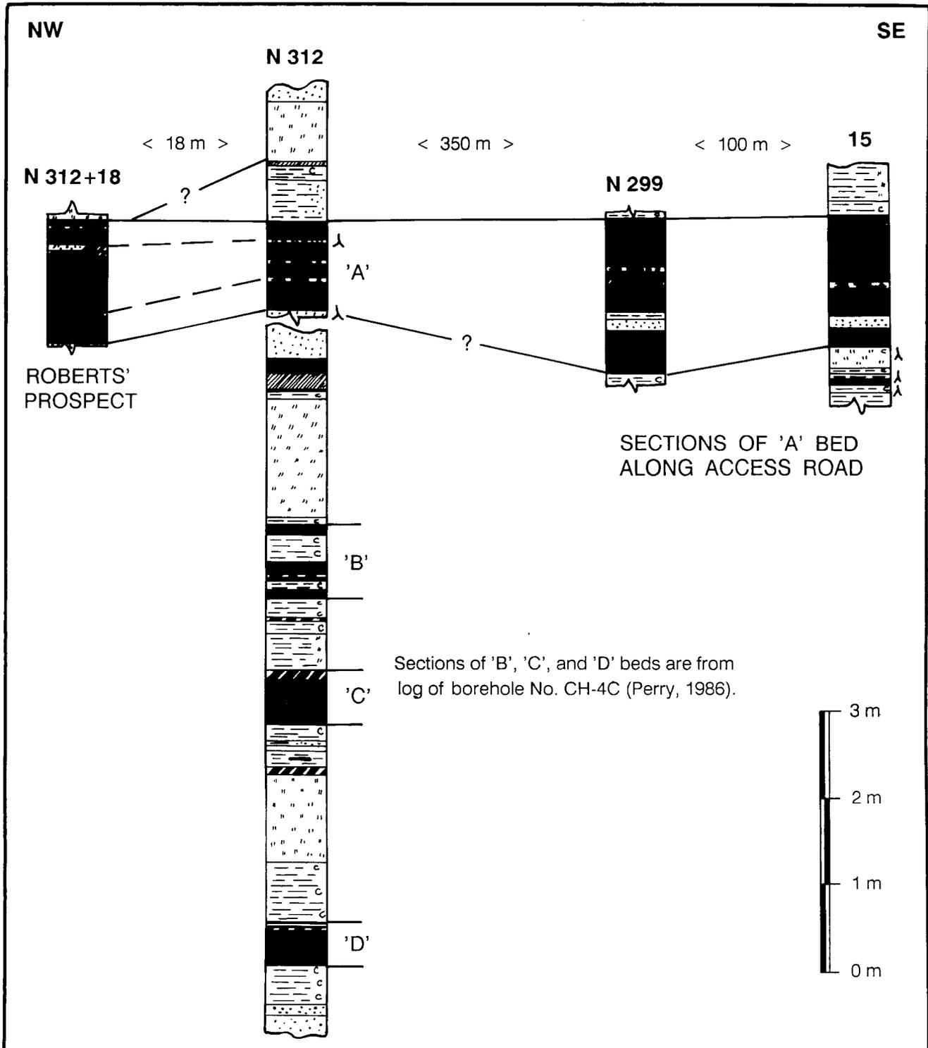
Figure 17. Details of coal beds A, B, C and D in the Chute Creek area, from measured sections and borehole data (see Figure 7 for stratigraphic legend).
