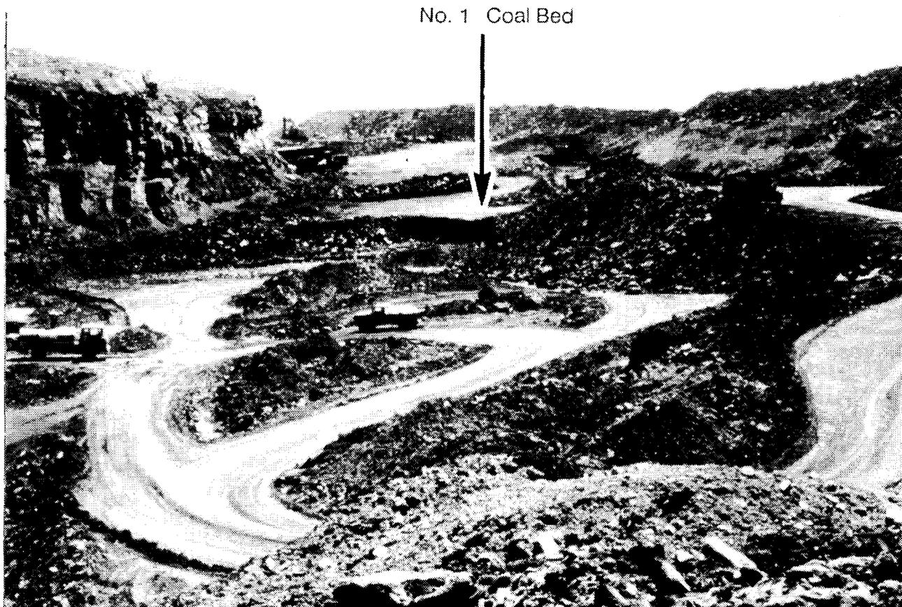
Plate 21. Open pit mining operation in Pit 2N on the Quinsam property. All the material on top of the No.1 coal bed has been removed in preparation for removing this seam.
