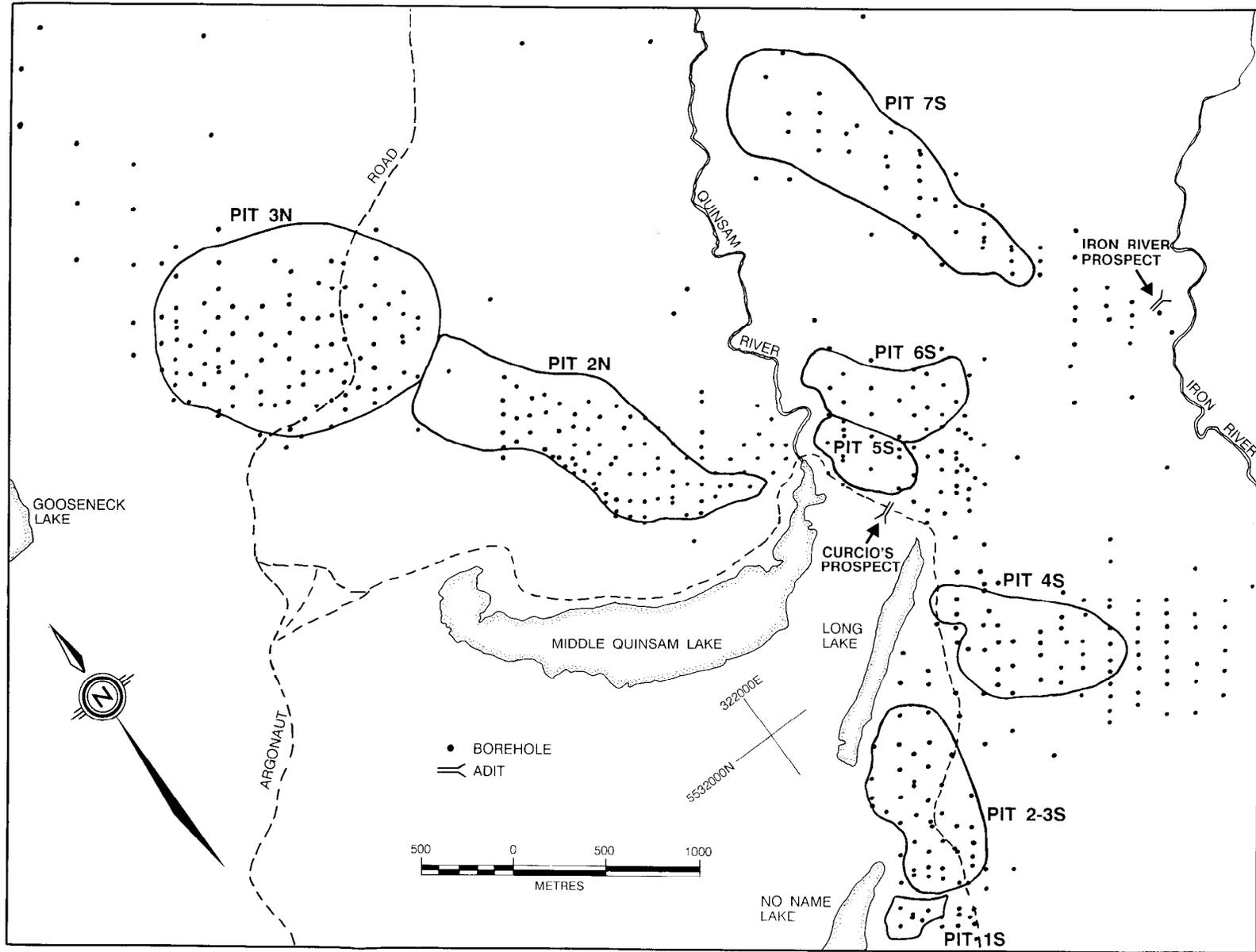
Figure 5. Quinsam area exploration map; indicating the drilling density and adit locations. The pits are reserve blocks of potentially mineable coal. Both surface and underground methods are necessary to mine these areas.
