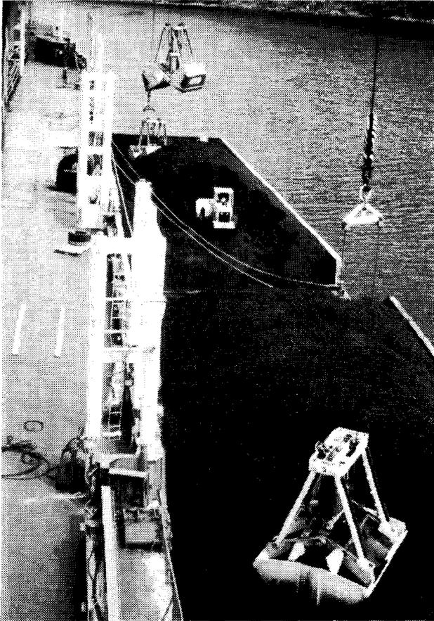
Plate 24. A Korean ship loading coal, from barges towed from Middlepoint, on a ship bound for Japan. The new facility at Texada Island has replaced this method.
