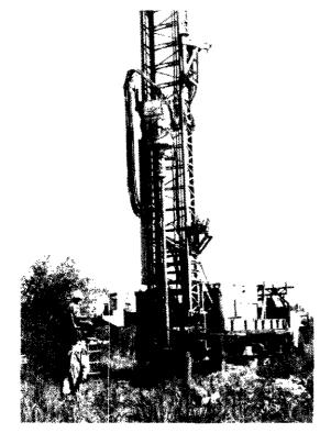
Plate 3-4-2. View of sonic drill used in neotectonic study to obtain solid core of unconsolidated sediment.
