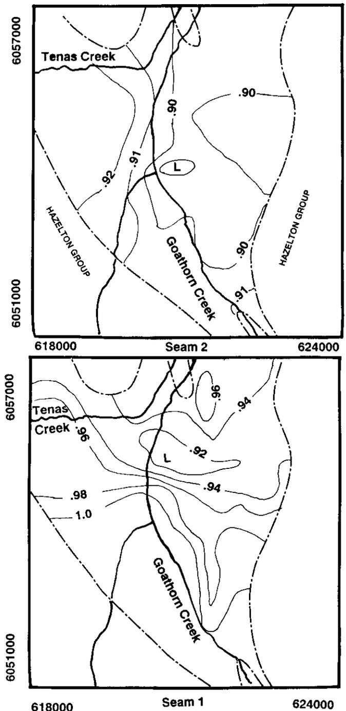
Figure 4-8-8. Contours of calculated mean maximum reflectance data for Seams 2 and 1.
