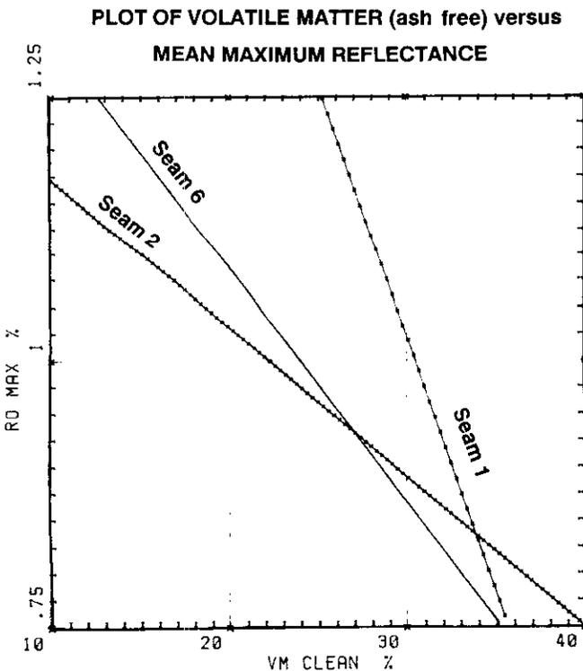
Figure 4-8-6. Mean maximum reflectance versus calculated volatile matter on an ash-free basis, Seams 6, 2 and 1. Contours of  $\bar{R}_{max}$  % calculated from VM data.
