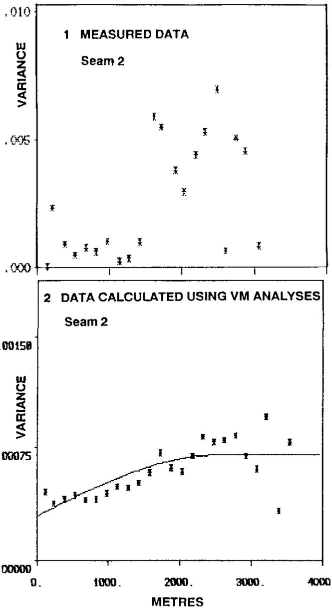
Figure 4-8-7. Variograms for mean maximum reflectance data and calculated mean maximum reflectance data; Seam 2.
