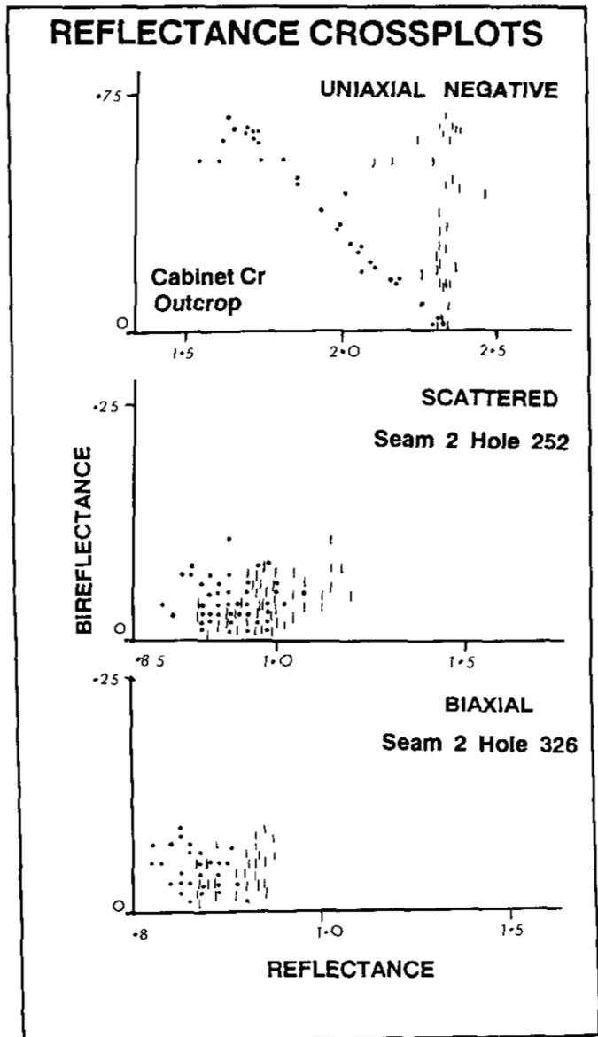
Figure 4-8-4. Examples of reflectance measurement populations for samples, illustrating different RIS.
