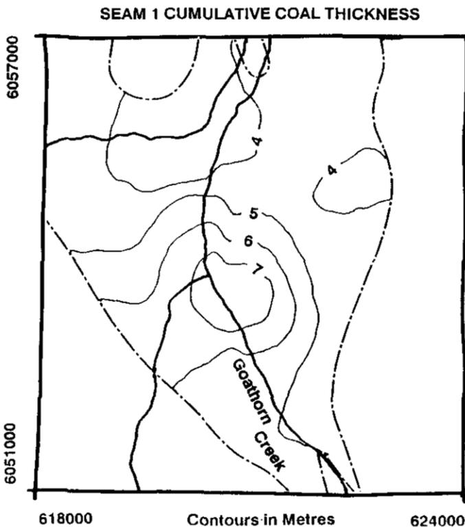
Figure 4-8-2. Cumulative coal thickness for the upper seams (2 to 10) and Seam 1; Goathorn Creek area.
