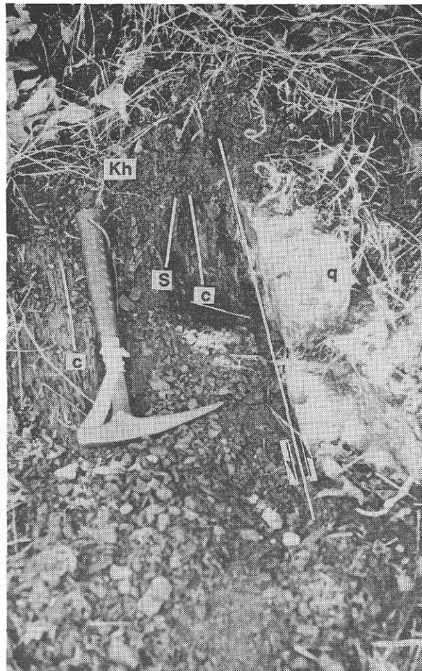
Plate 25. Fulford fault; quartz porphyry (q) of the Salt-spring Intrusive Suite adjacent to Haslam Formation argillite (Kh). Note the well-developed c fabric and moderate s fabric indicate that motion on the fault was northside (i.e. quartz porphyry) up. The fault dips 80° northwards (Maple Bay; NMA87-45-10: 5407148N; 455307E).
