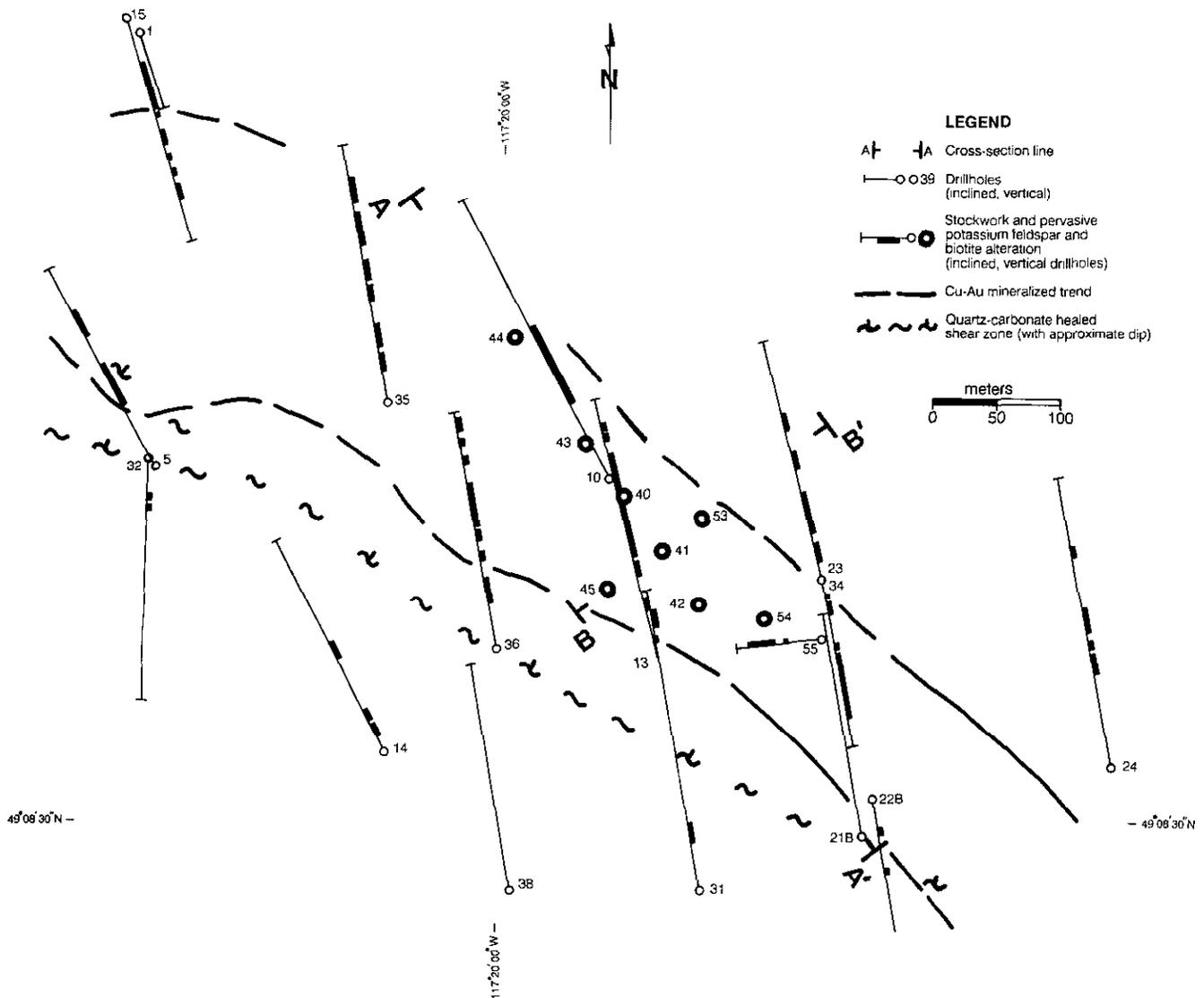
Figure 2-1-3. Drillhole plan for the Main zone, Katie property. Drillhole traces and the extent of alteration zones and mineralization are shown projected to surface.
