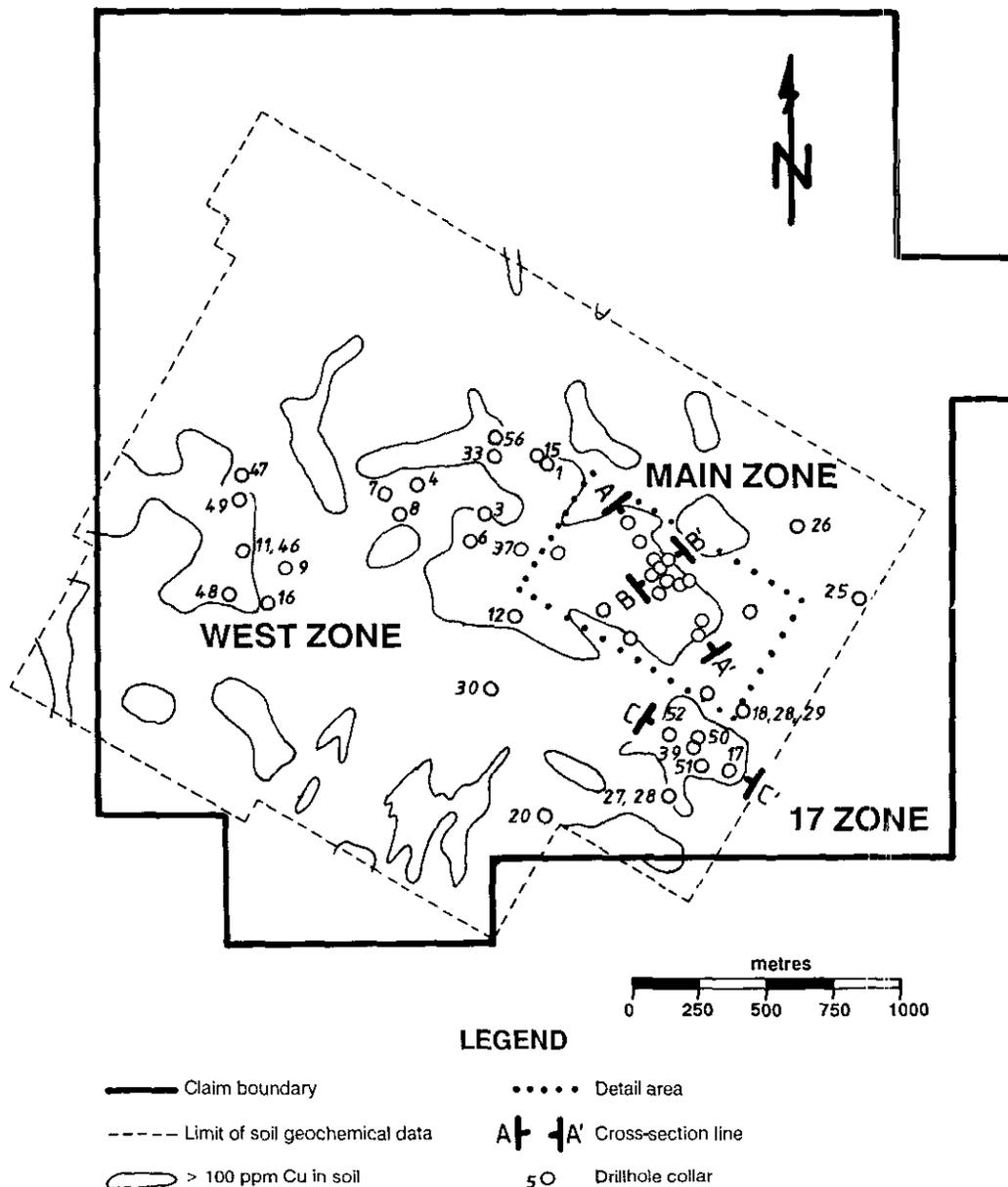
Figure 2-1-2. Drillhole plan for the Katie property. The location of Figure 2-1-3 is shown by the heavy dotted line. The locations of cross-section lines are also shown (see Figure 2-1-4).
