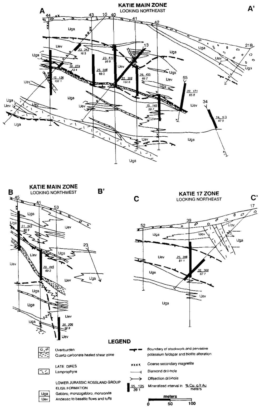
Figure 2-1-4. Cross-sections through the Main and 17 zones, Katie property. The locations of cross-section lines are shown on Figures 2-1-2 and 2-1-3.
