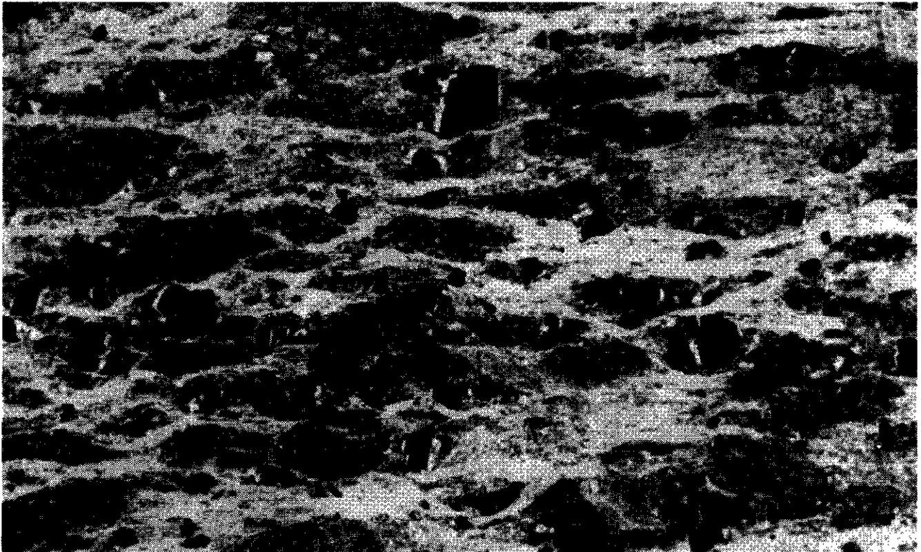
Plate 2-1-6. Protomylonite. Note rotated sulphide grains with quartz pressure shadows and replacement of feldspar by sericite and carbonate. Katie DDH 13-100.4 metres (ppl, field of view = 5.1 mm).
