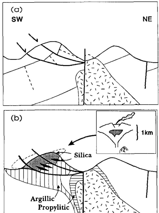
Figure 2-7-4. Structural style, diagrammatic cross-section; (a) large-scale fault block displacements of south and southwesterly dipping beds results in exposure of similar lithologies and stratigraphy in the map area; (b) tilting and low-angle normal faulting of hydrothermally altered rocks result in compression (telescoping) of alteration zones.
