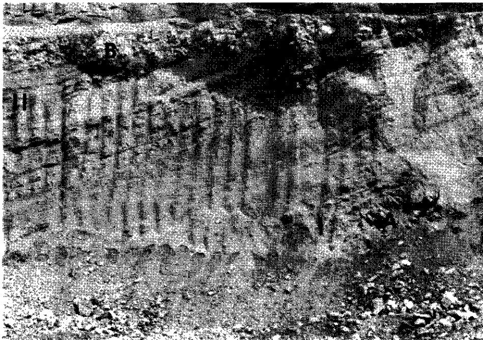
Plate 4-4-1. View of fractured bedrock (A) and lithostratigraphic units (I) and (II) at base of Valley pit excavation, Highland Valley Copper mine, British Columbia. Exposure is 12.5 metres high. Pebbly diamicton at top of photo is modern road fill (B). Unit I is interpreted as slope wash and grus.
