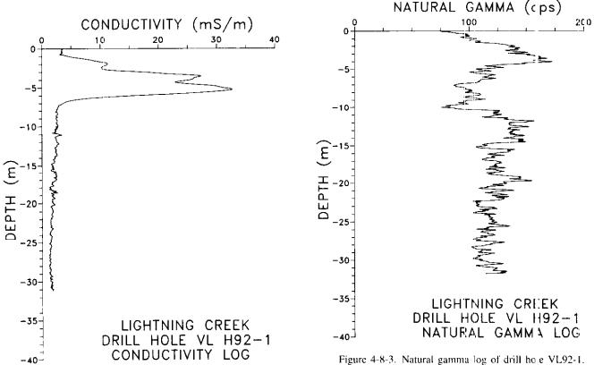
Figure 4-8-2. Conductivity log of drill hole VL92-1 at the Gallery Resources mine on Lightning Creek. High conductivity in the upper several metres of the hole reflects high silt and clay contents whereas low conductivity is indicative of gravelly deposits. (mS/m = millisiemens/metre).
