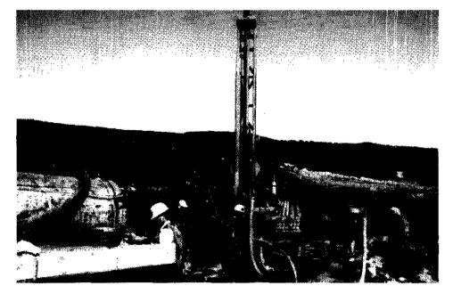
Plate 4-8-1. The reverse-circulation drill used in this study drilling hole number VI.92-3, due west of the Alice Creek mine. The cyclone on the right hand side of the drill is used to eatch the drill samples.
