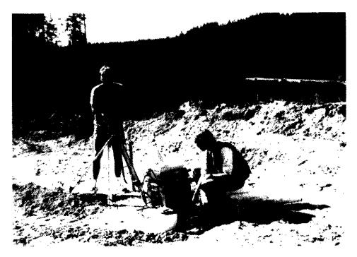
Plate 4-8-3. Geonics EM-39 logging system for apparent conductivity, naturally occurring gamma radiation and magnetic susceptibility. The apparent conductivity probe has been partially inserted into plastic (PVC) casing in the drill hole.
