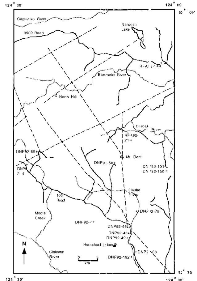
Figure 4-11-1. Location map of observation sites (+) and geographic names mentioned in the text. Dashed lines are seismic lines, solid lines are roads and grey lines are rivers.
