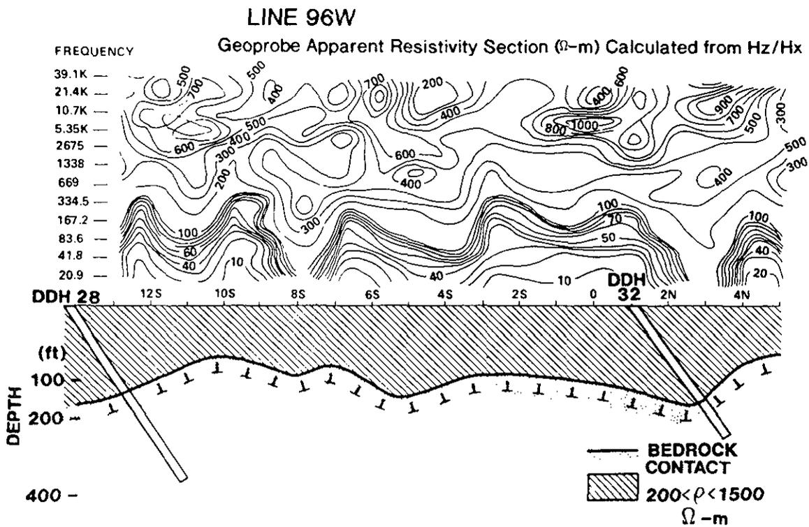
Figure 25-11. Geoprobe response along line 96W and a rough interpretation using a layered earth model.
