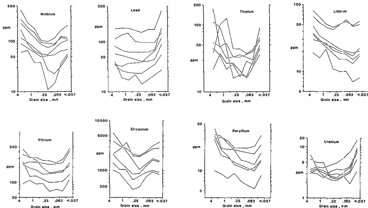
Figure 15-9. Abundance of Nb, Y, Be, Zr, Th, Li, Pb and U versus grain size of analyzed fraction of seven samples of oxidized till in the Strange Lake dispersal train, Labrador.
