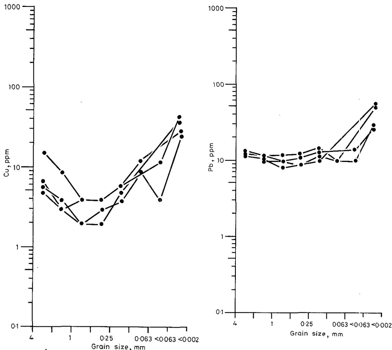
Figure 15-12. Abundance of copper and lead versus grain size of analyzed fraction of oxidized till at the Kazan Falls uranium occurrence, Kazan River, N.W.T.
