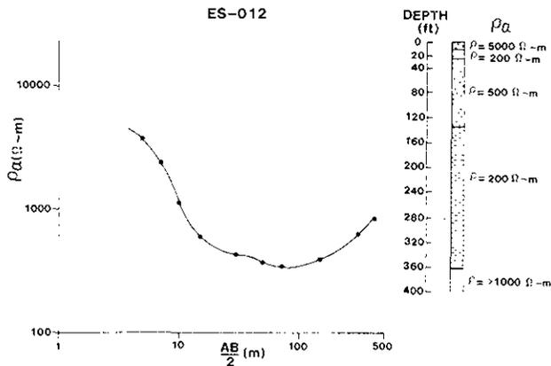
Figure 25-12. Schlumberger resistivity sounding (ES-012).
