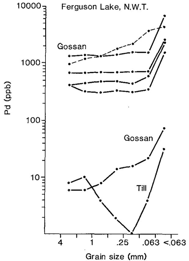
Figure 15-7 . Abundance of platinum (in 5 samples) and palladium (in 7 samples) versus grain size of analyzed fraction of gossanous sediment and of till (one sample, Pd only) from the Ferguson Lake nickel-copper occurrence, District of Keewatin. Curves are dashed and dotted for clarity.
