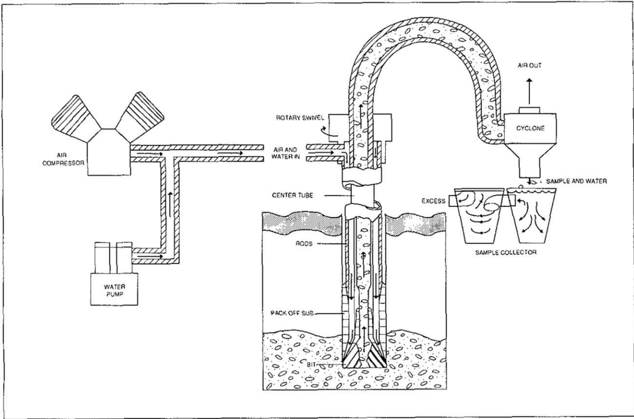
Figure 4-1. Schematic cross-section of a reverse-circulation drill; modified from Averill (1990).
