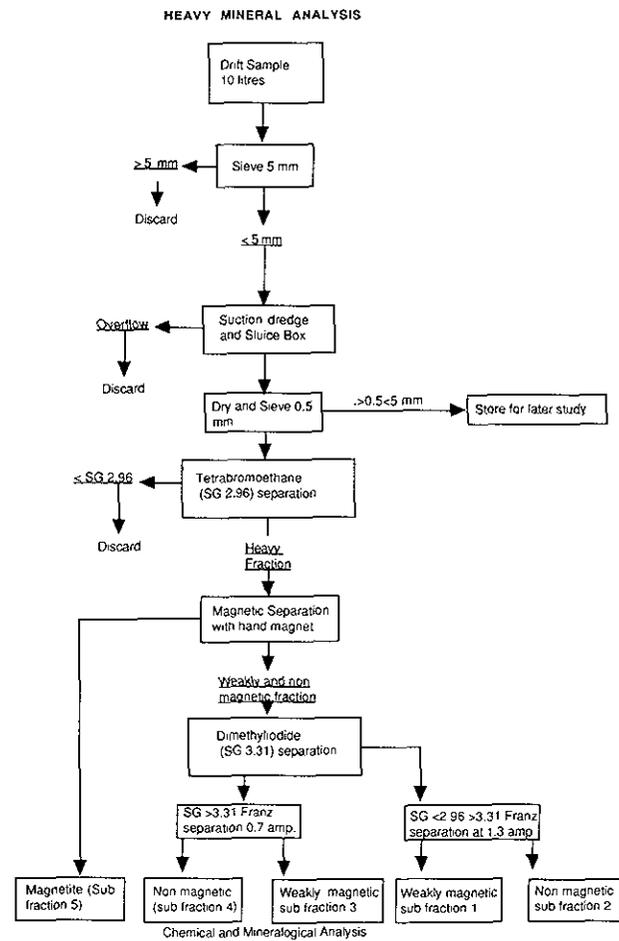
Figure 21-4. Processing and analytical scheme of drift samples from Sweden (Brundin and Bergstrom, 1981).
