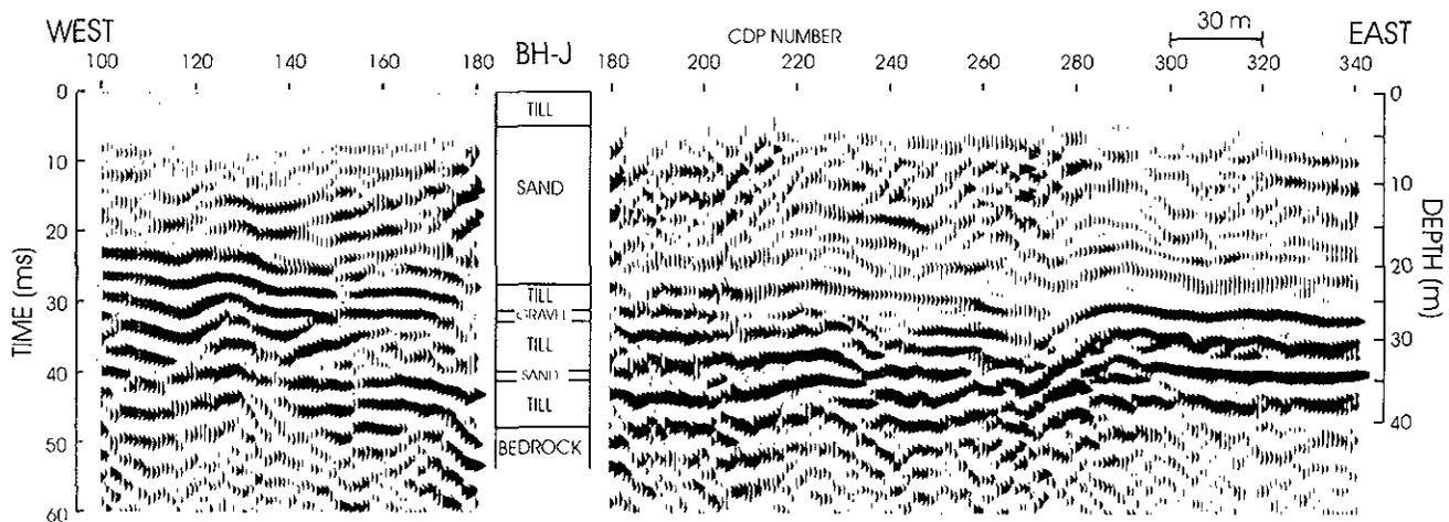
Figure 23-6. A six-fold CDP section approximately centred on borehole J. A simplified lithological log has been inserted in the section at the bore-hole location. The section clearly delineated the top of the till sequence at a depth of approximately 25 metres, and suggests the existence of a small bedrock valley between CDP numbers 225 and 280.
