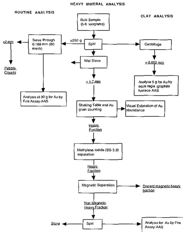
Figure 21-3. Processing and analysis of overburden samples from Waddy Lake, Saskatchewan (Averill and Zimmerman, 1986).
