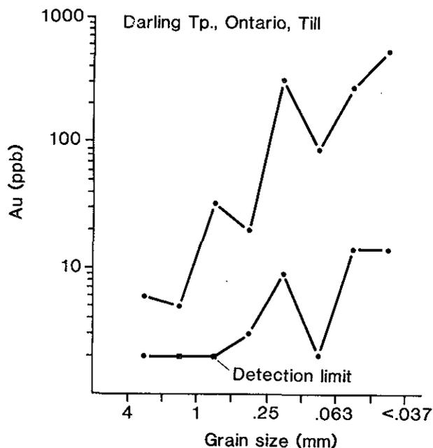
Figure 15-4. Abundance of gold versus grain size of analyzed fraction of oxidized anomalous (upper curve) and near-background (lower curve) till in Darling Township, Ontario.
