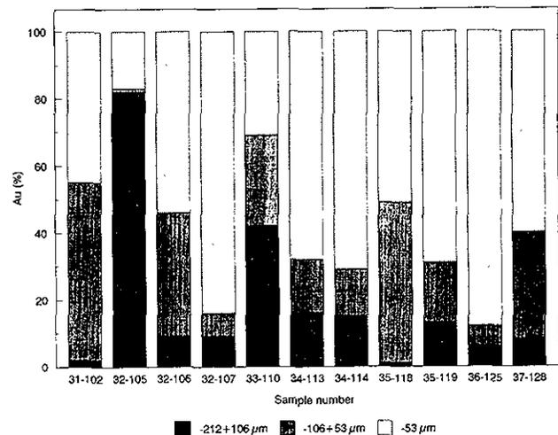
Figure 14-2. Proportion of gold in the -212+106µm, -106+53µm and -53µm fractions of A and B-horizons
