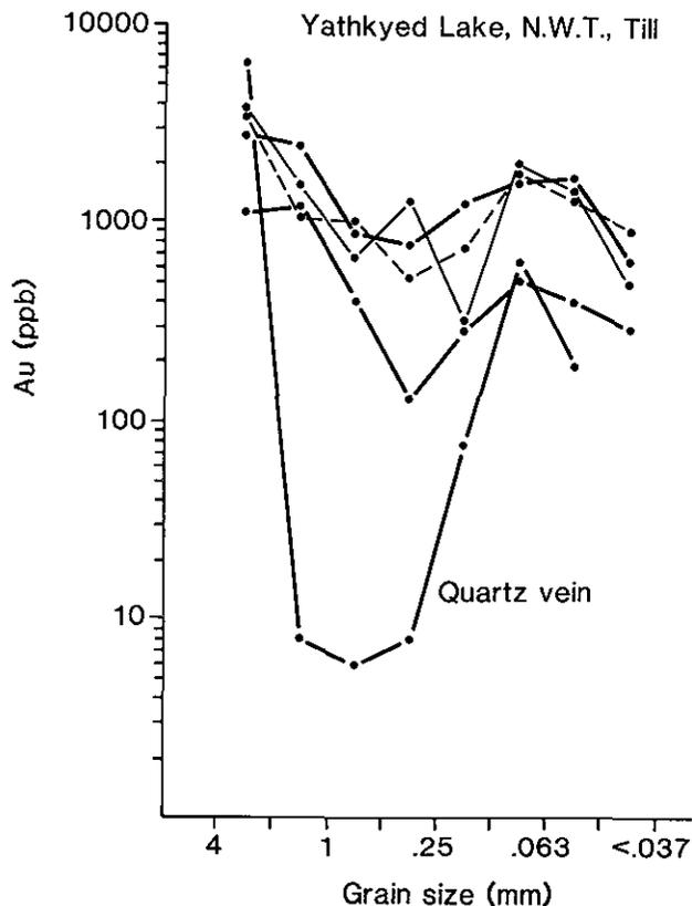
Figure 15-5. Abundance of gold versus grain size of analyzed fraction of oxidized till from near a quartz vein (one sample) and from near a stratiform deposit (four samples) near Yathkyed Lake, District of Keewatin, N.W.T. Curves were drawn with different patterns for clarity.
