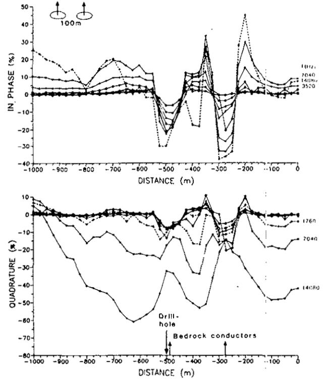
Figure 25-20. MaxMin data at all eight frequencies. The location of the follow-up survey for these two bedrock conductors is indicated in Figure 18 and corresponds to target 18 in Figure 15.
