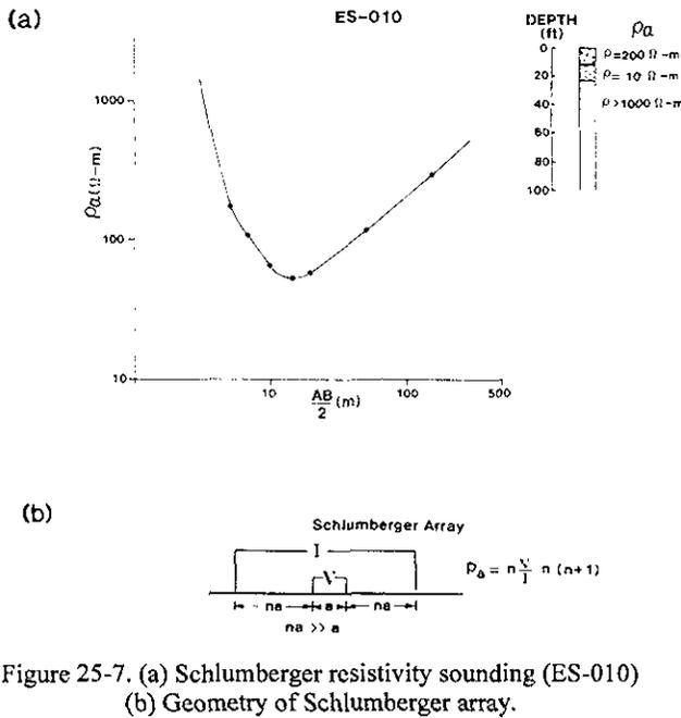
Figure 25-7. (a) Schlumberger resistivity sounding (ES-010) (b) Geometry of Schlumberger array.
