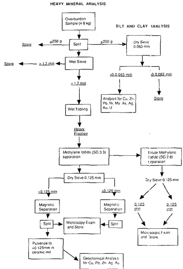
Figure 21-2. Processing and analysis of KLIP overburden samples (Routledge *et al.*, 1979).
