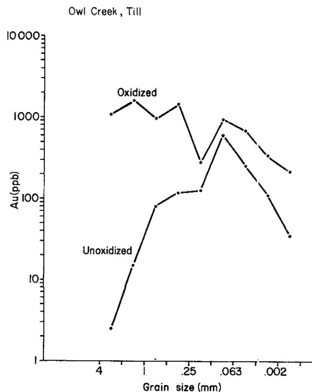
Figure 15-3. Abundance of gold versus grain size of analyzed fraction of a sample of unoxidized till and its oxidized equivalent at the Owl Creek mine, Timmins, Ontario.
