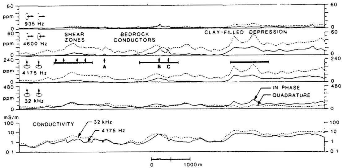
Figure 25-18. Composite profile of helicopter AEM data (in-phase and quadrature components at four frequencies, two coil configurations) and calculated conductivity based on horizontal coplanar data. This section goes from target 17 to target 24 in Figure 25-15.
