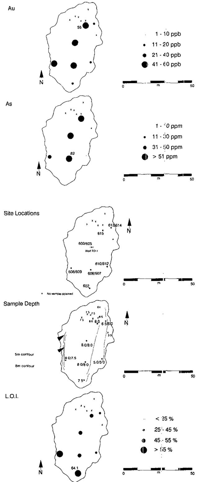
Figure 20-13. Wolf Pond, showing distribution of gold (ppb), arsenic (ppm) and loss on ignition (%), and site locations and sample depths (m).
