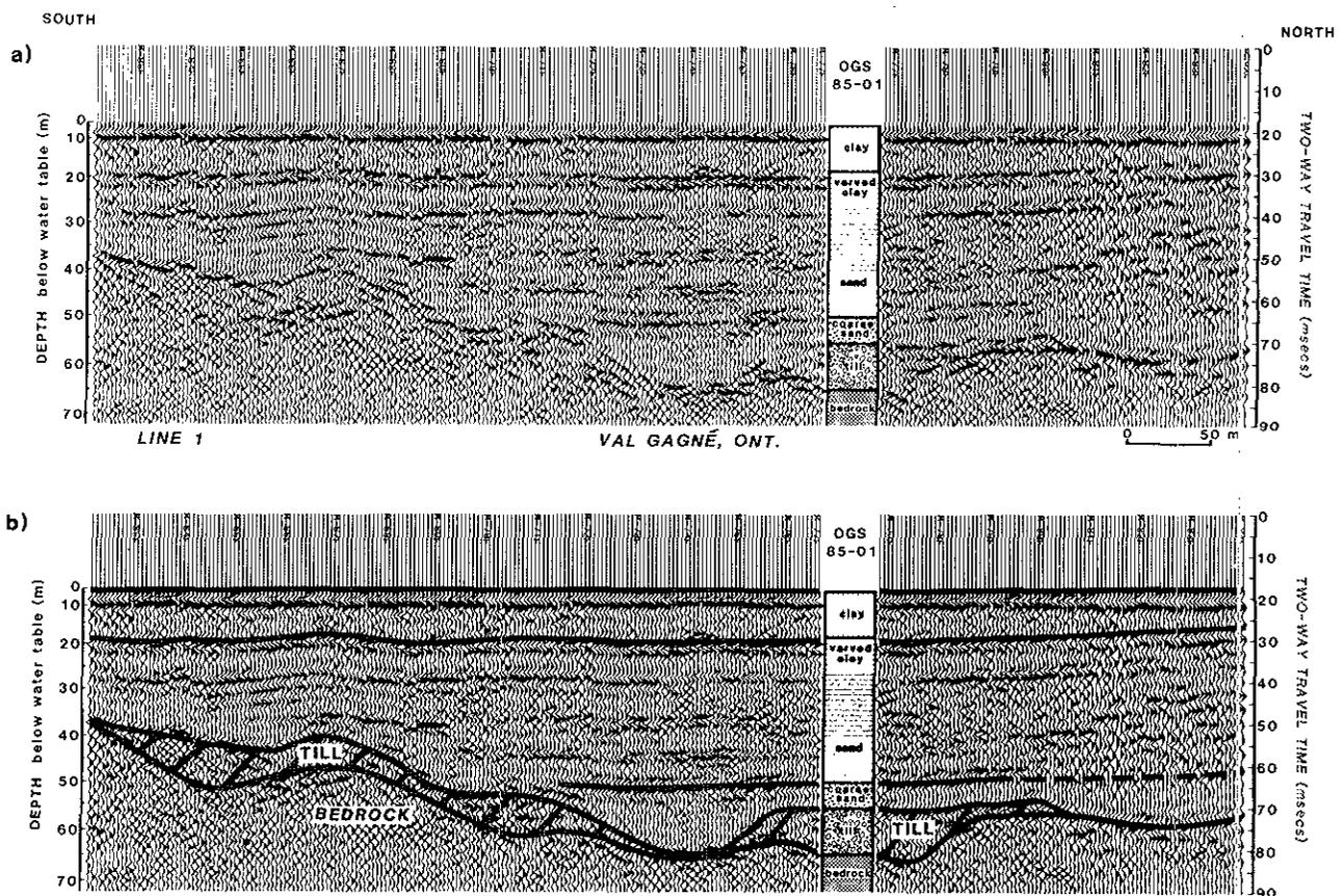
Figure 23-5. (a) Line 1 from Val Gagné, Ontario, with a simplified drill log shown at the location of OGS sonic-drill hole 85-01. (b) An interpretation of Figure 23-5a, indicating the extension of lithological units north and south of the borehole, and probable occurrences of till (from Pullan *et al.*, 1987).
