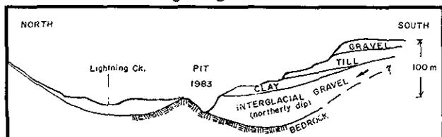
Figure 8-8. Diagrammatic cross-section, McGuire property, Lightning Creek.
