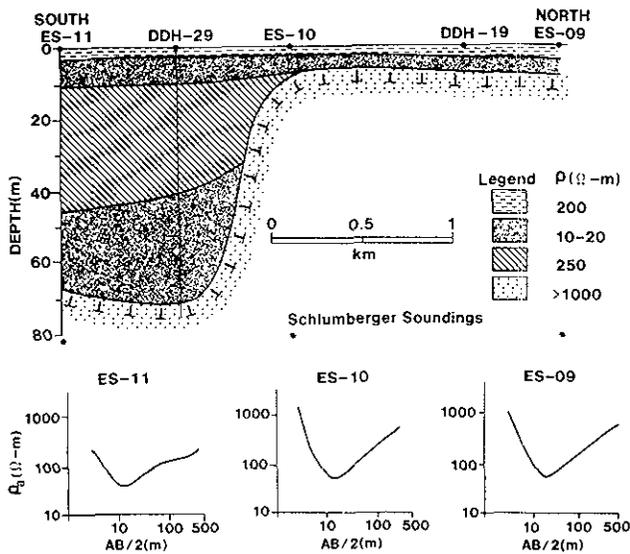
Figure 25-8. Resistivity section along line with drill hole 29 and sounding ES-010.
