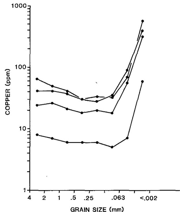
Figure 15-11. Abundance of nickel and copper versus grain size of analyzed fraction of oxidized till at Ferguson Lake, N.W.T.
