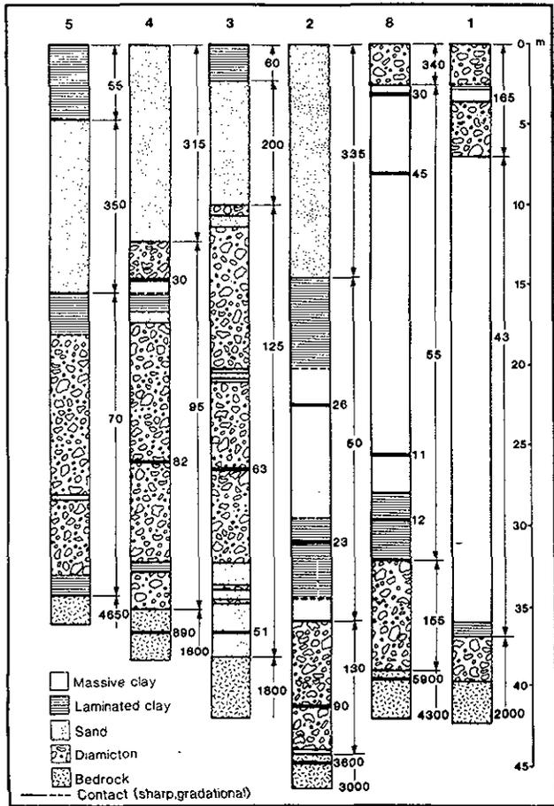
Figure 25-21. Stratigraphic logs of holes along the Fraserdale - Smooth Rock Falls transect. Numbers between arrows indicate resistivities ( $\rho$ -m) which were determined as the best fit to the HLEM data. The actual thicknesses of the indicated layers on the logs were used as fixed parameters in the inversion. Numbers next to the horizontal lines are resistivities determined in the laboratory on core samples.
