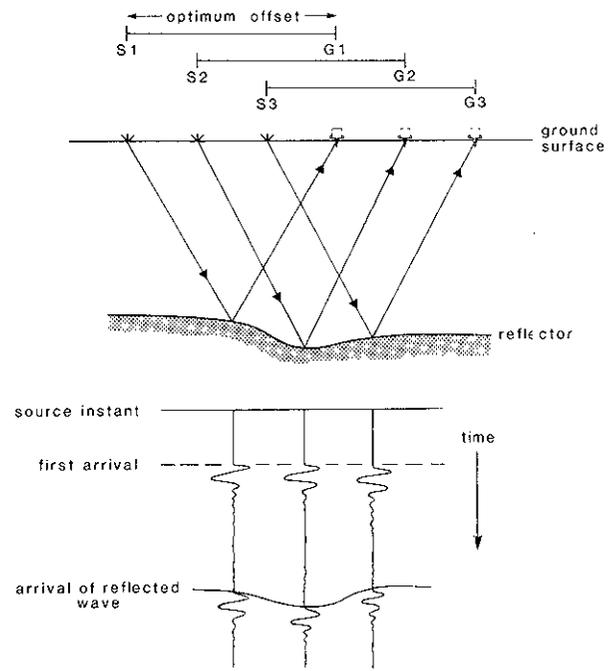
Figure 23-3. The schematic optimum-offset section shown at the bottom of the figure was produced by shooting first from S1 (source position 1) and recording the output at G1 (geophone 1), then from S2 to G2, and finally from S3 to G3.
