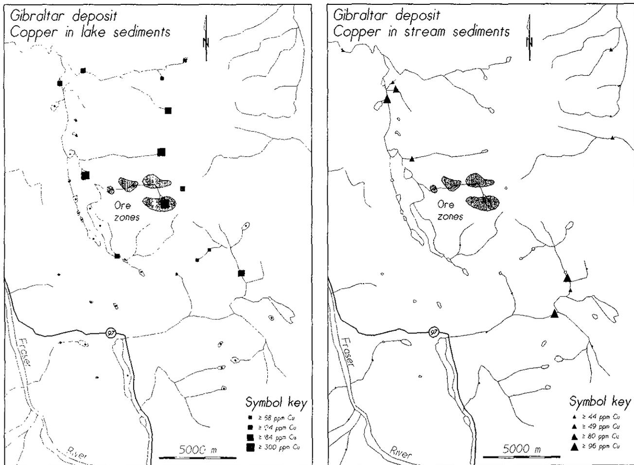
Figure 19-9. Copper in lake and stream sediments in the Gibraltar mine area (93B).
