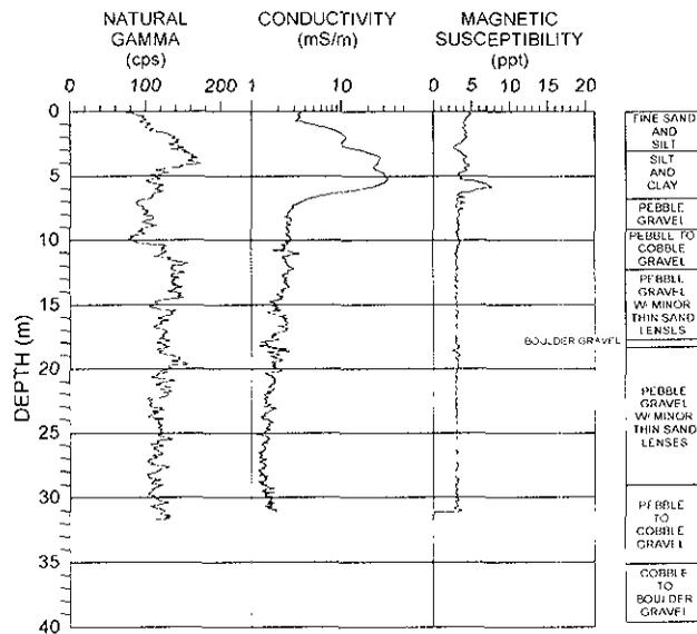
Figure 24-3. EM-39 borehole logs and generalized sample descriptions from hole VL H92-1, Lightning Creek, east of Quesnel, B.C.
