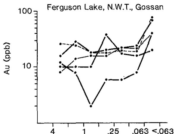
Figure 15-6. Abundance of gold versus grain size of analyzed fraction of five samples of gossanous sediment from the Ferguson Lake nickel-copper occurrence, District of Keewatin, N.W.T.
