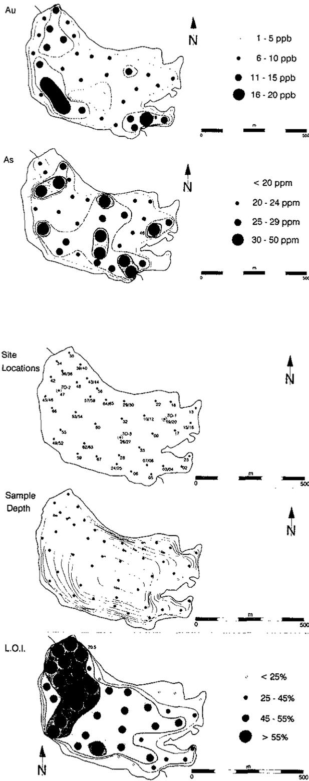
Figure 20-14. Clisbako Lake, showing distribution of gold (ppb), arsenic (ppm) and loss on ignition (%), and site locations and sample depths (m).
