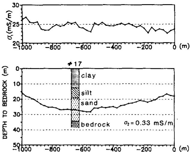
Figure 25-17. Overburden conductivity and depth to bedrock profiles obtained by ridge regression inversion of the MaxMin data in Figure 16. Drilling results are shown at position 650 m (from Palacky and Stevens, 1990).
