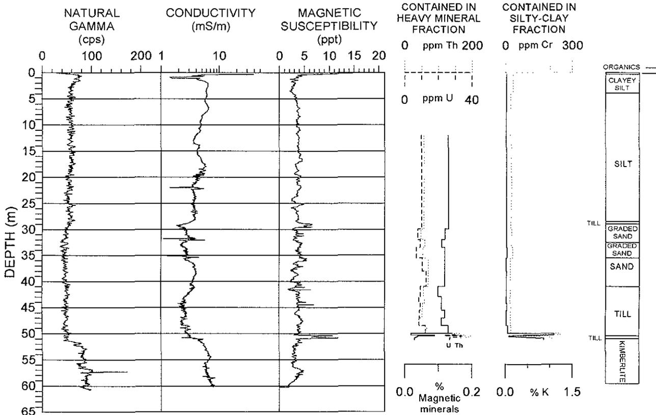
Figure 24-1: EM-39 borehole logs and selected geochemical results from hole B-30-03, a kimberlite prospect near Kirkland Lake, Ontario. U = uranium, Th = thorium, K = potassium, Cr = chromium.
