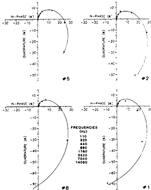
Figure 25-22. Argand diagrams displaying the HLEM observations (stars) and the responses from the best fit (solid curves) for locations 1, 2, 5 and 8. The layer parameters are given in Figure 25-20.
