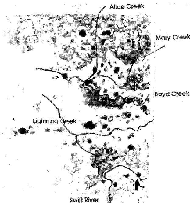
Figure 9-3. Computer classification, darkest polygons are prime exploration targets. 1:50 000 (see Figure 9-1 for location)
