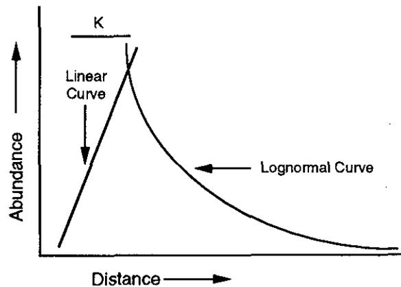
Figure 11-3. Schematic figure showing estimation of parameter K using proximal rise (linear function) and distal decline (lognormal function) for theoretical dispersal curve. Modified after Salonen and Palmu (1989).
