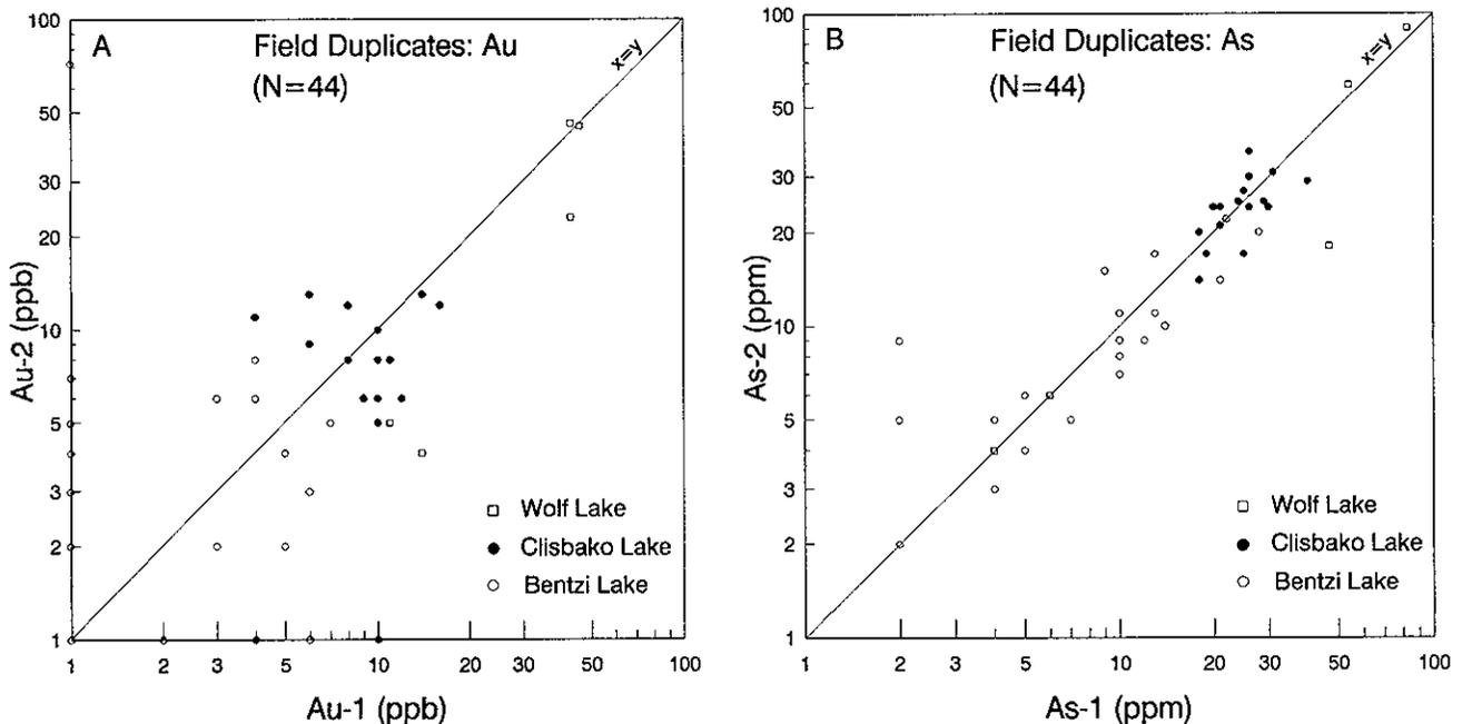
Figure 20-7. Log scatterplot of field duplicate A) gold determinations (ppb; INAA) and; B) arsenic determinations (ppm; ICP) from samples from Wolf (n=5), Clisbako (n=17) and Bentzi (n=22) Lakes.
