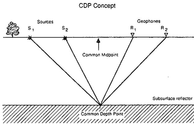
Figure 23-4. Illustration of the common depth point (CDP) concept. When 24-channel records are recorded at each shotpoint, and shotpoints coincide with every geophone location, the subsurface reflection points will be sampled 12 times, resulting in 12-fold CDP data after processing. (Steeple and Miller, 1990).
