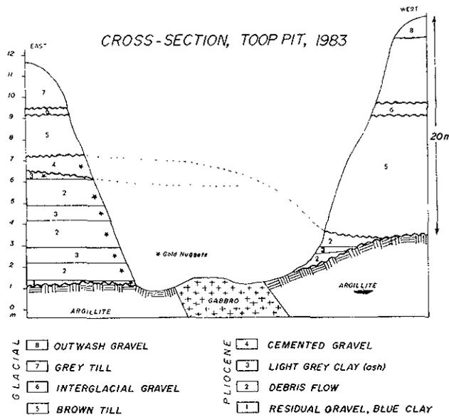
Figure 8-10. Cross-section and stratigraphy, Toop pit, 1983.
