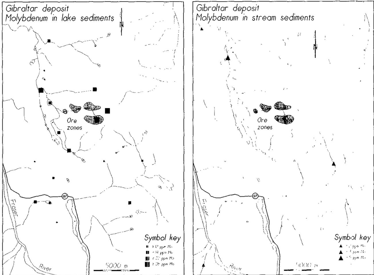
Figure 19-10. Molybdenum in lake and stream sediments in the Gibraltar mine area (93B).
