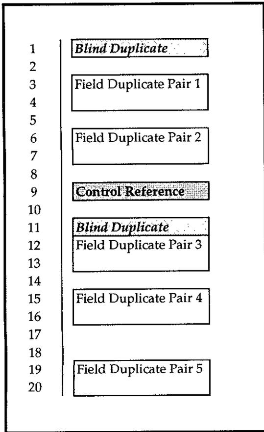
Figure 20-6. Typical sample collection scheme. The modified 20-sample collection block incorporates twelve routine samples and five field duplicates. Two blind duplicates and a control reference standard are inserted in prep laboratory prior to analysis.
