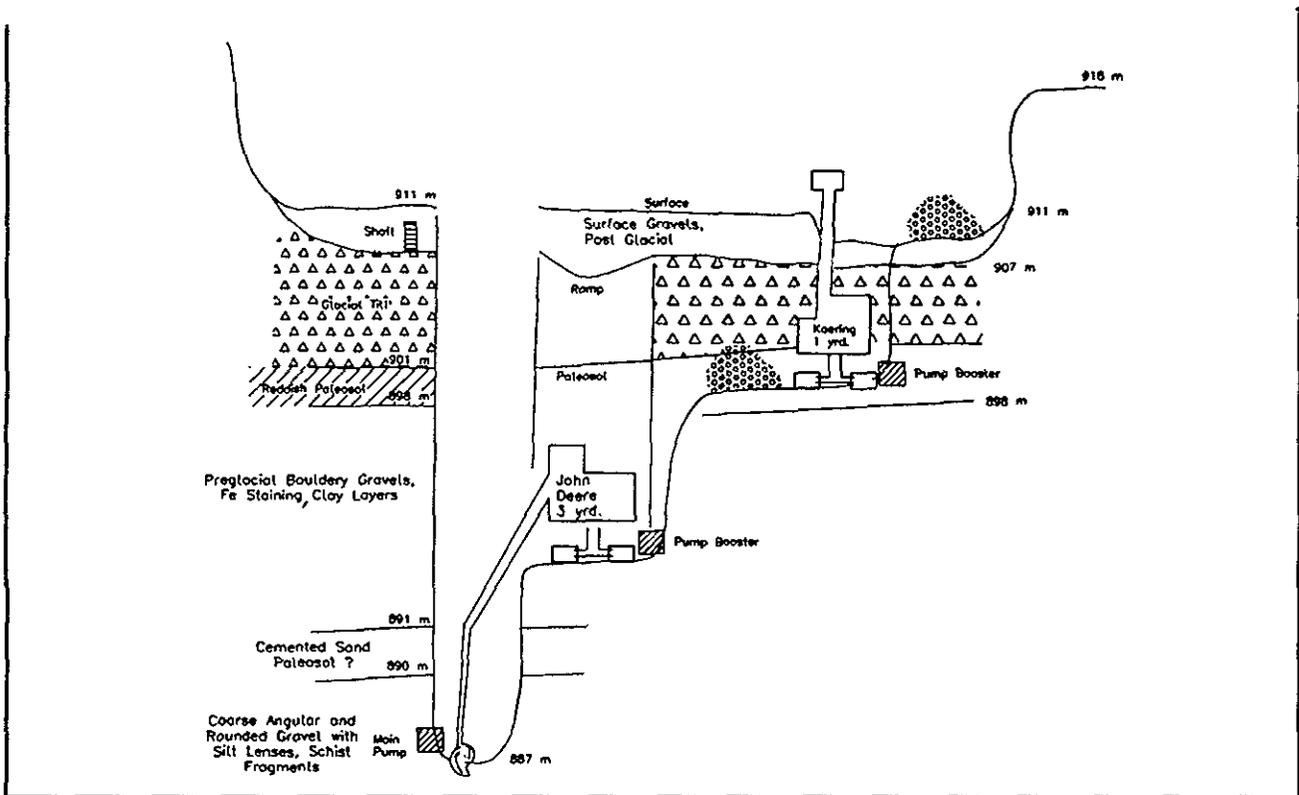
Figure 9-4. Meltwater-channel test hole, Auramet International Ltd., 93B/16E, August 12-16, 1985 (see Figure 9-1 for location).
