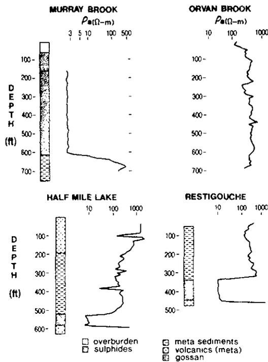
Figure 25-3. Resistivity logs from four massive sulphide deposits in New Brunswick.
