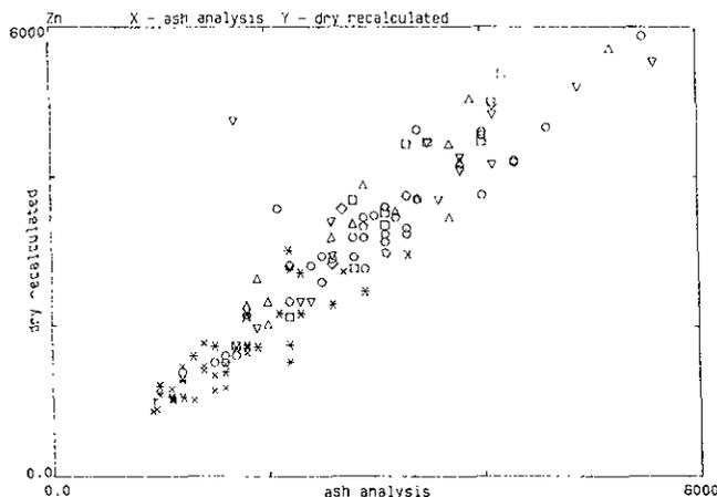
Figure 22-2. Plot of zinc content of dry tissues *versus* ash, demonstrating no loss on ignition to 470°C. Symbols represent different tissues from boreal species.
