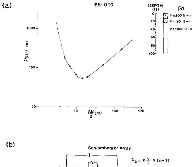
Figure 25-7. (a) Schlumberger resistivity sounding (ES-010) (b) Geometry of Schlumberger array.
