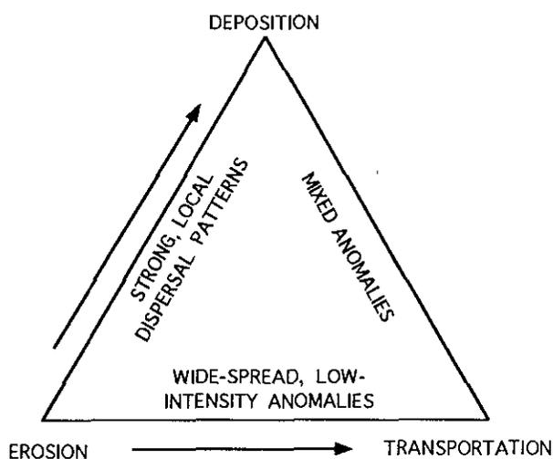
Figure 11-4. Ternary plot of glacial processes indicating relationship between erosion, transportation and deposition and effects on indicator dispersal patterns. Modified after Salonen (1989).
