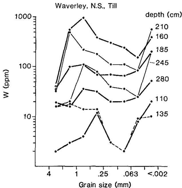
Figure 15-8 . Abundance of tungsten versus grain size of analyzed fraction of oxidized till at varying depths below surface at Waverley, Nova Scotia.
