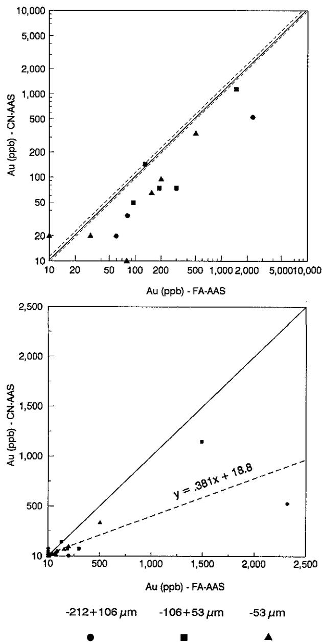
Figure 14-3. Comparison of analyses by CN-AAS and FA-AAS for each size fraction. Samples with gold values <10 ppb are excluded. For both figures the solid line represents the  $x=y$  line. (a) Data shown on a logarithmic scale. Dashed lines represent 20% limits. (b) Data shown on an arithmetic scale. Results of regression analysis (dashed line and equation) conducted at the .05% confidence level.
