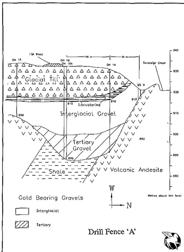
Figure 9-10. Drill fence 'A'. Schematic cross-section through "preglacial Sovereign Creek", Cariboo goldfield, B.C.
