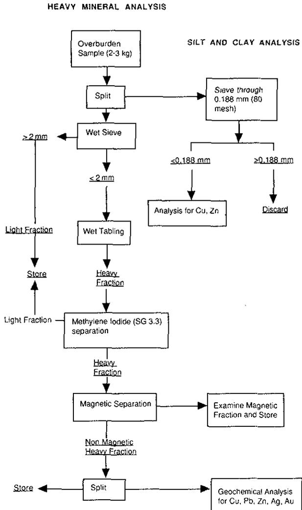
Figure 21-1. Processing and analysis of overburden samples from Ontario (Thompson, 1979).
