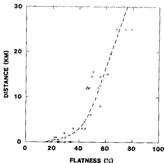
Figure 13-3. The relationship between gold particle flatness and distance of transport from the lode source for the Klondike. The triangle represents a sample containing some gold which originated in the White Channel gravel paleoplacer (Knight *et al.*, 1994).
