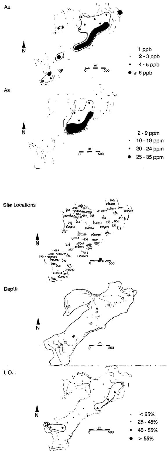
Figure 20-15. Bentzi Lake, showing distribution of gold (ppb), arsenic (ppm) and loss on ignition (%), and site locations and lake depth (m). Depth contours after Walsh and Philip (1977).
