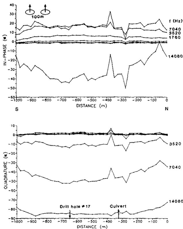
Figure 25-16. Results of MaxMin survey over a bedrock depression (location 17 in Figure 25-15).
