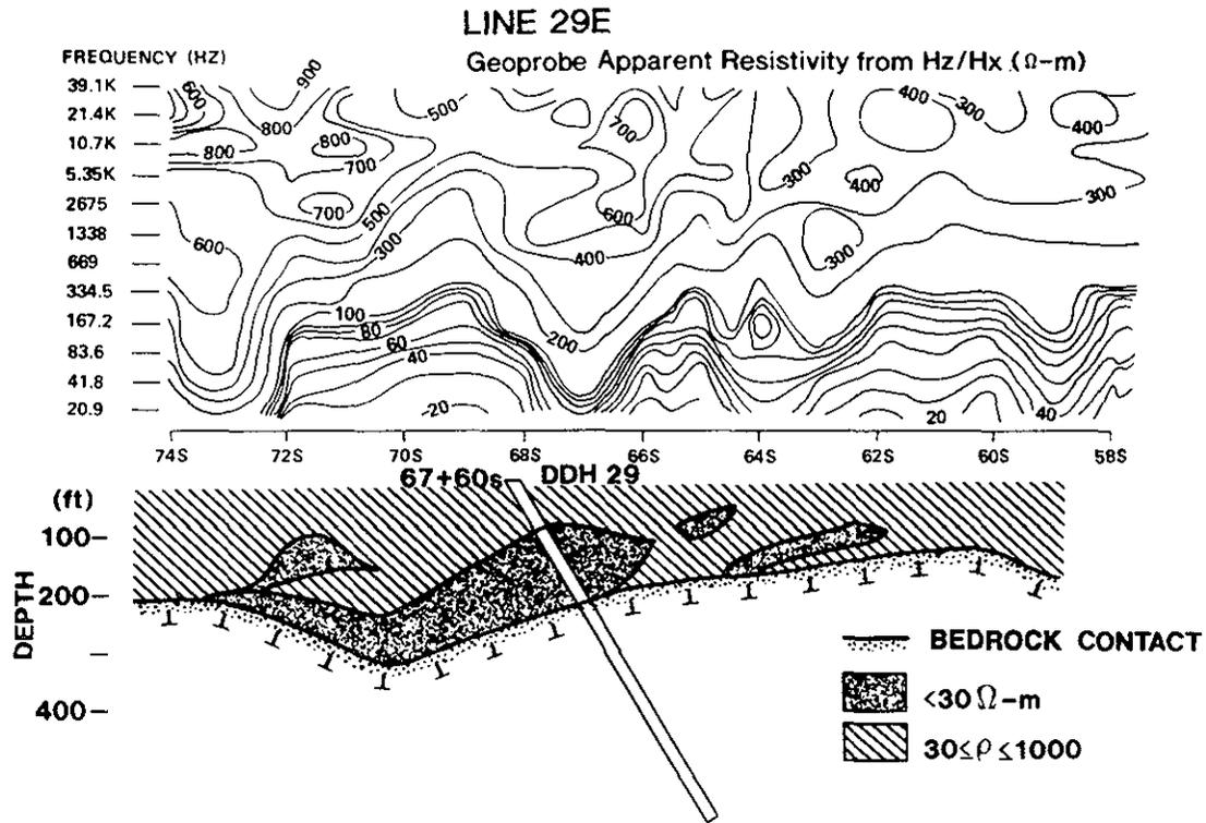
Figure 25-10. Geoprobe response over drill hole 29 and a rough interpretation using a layered earth model.
