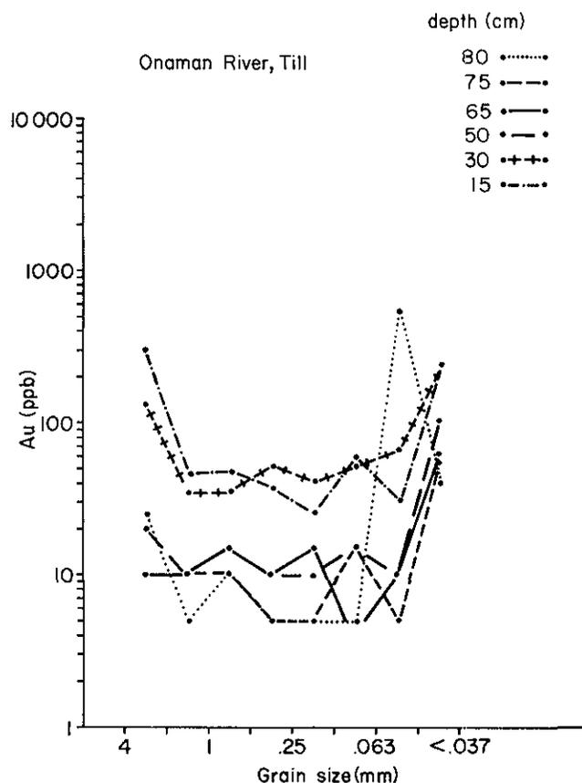
Figure 15-2. Abundance of gold versus grain size of analyzed fraction of oxidized till at varying depths below surface in a dispersal train at Onaman River, Ontario.
