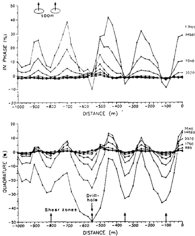
Figure 25-19. MaxMin data at all eight frequencies. The location of the follow-up survey for these shear zones is indicated in Figure 17 and corresponds to target 24 in Figure 25-15.
