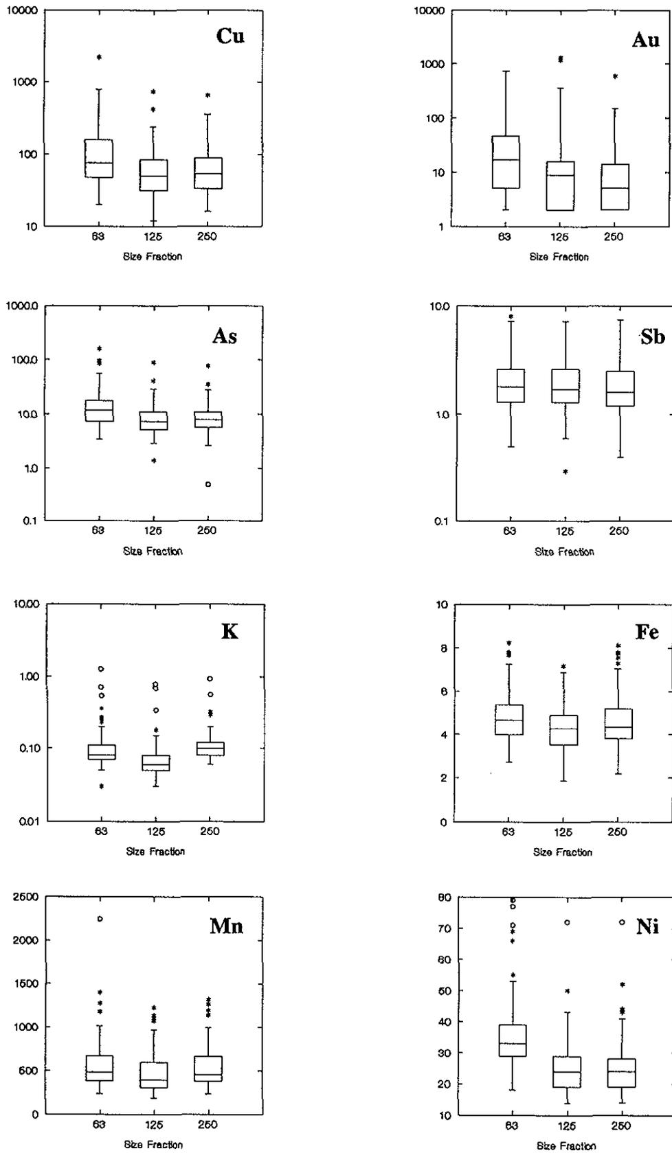
Figure 18-4. Box plots of element concentrations by size fraction for eight selected elements.
