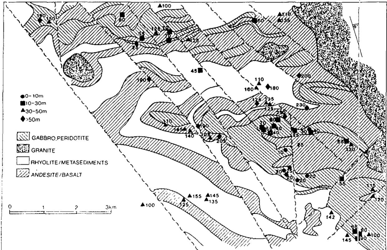
Figure 25-13. Geological map of Duff project area, together with depths of overburden at drill hole locations.
