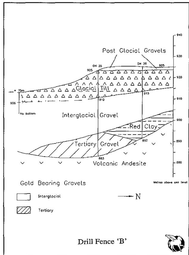
Figure 9-9. Drill fence 'B'. Schematic cross-section through "preglacial Sovereign Creek", Cariboo goldfield, B.C.
