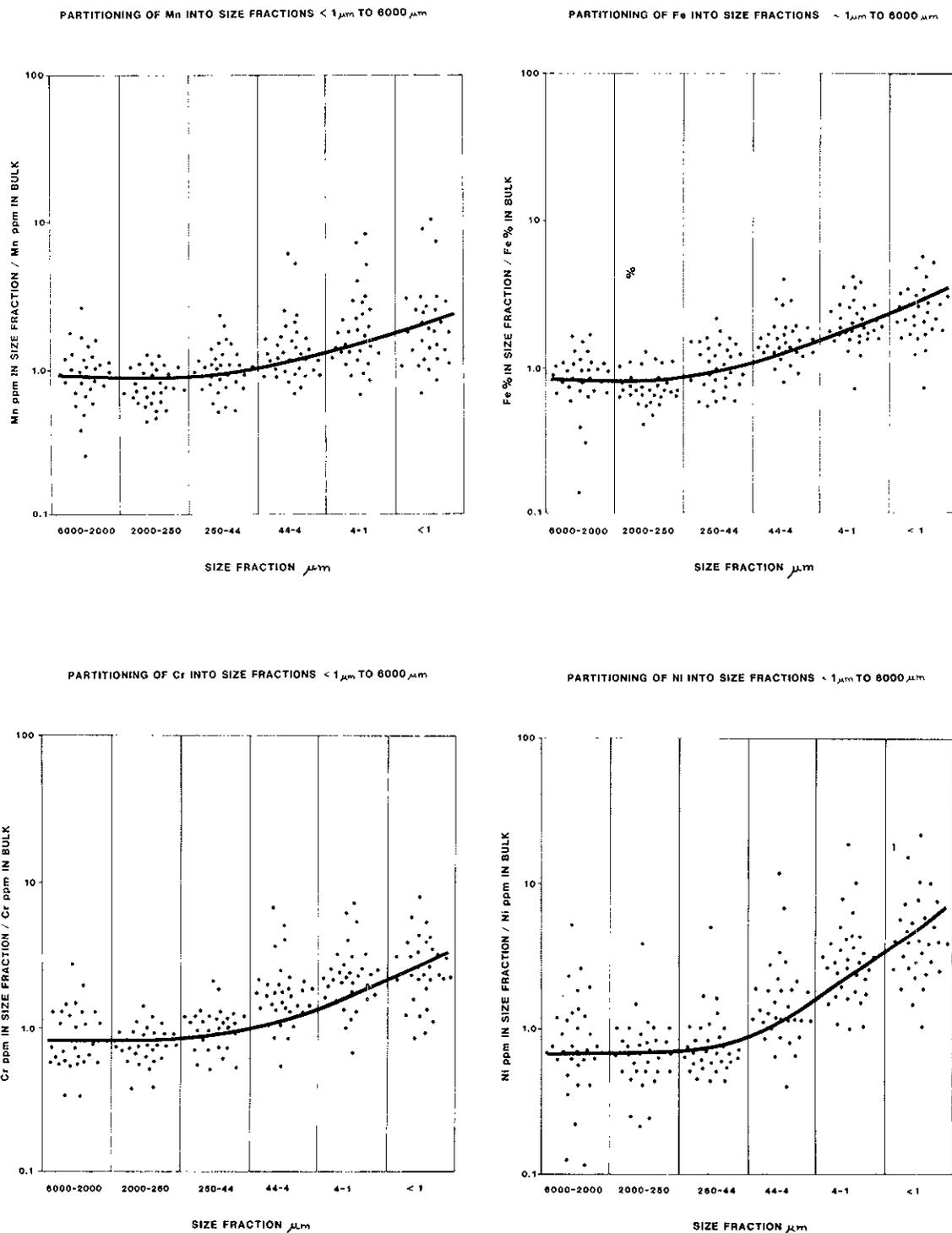
Figure 16-6. Logarithmic plots of the ratio of trace metal concentrations in selected size fractions <6000 micron to concentrations in bulk (<6000μm) fractions. Lateral spread of dots in size fraction cells is for convenience of plotting. Heavy lines are estimated trends drawn by hand approximately through median values.
