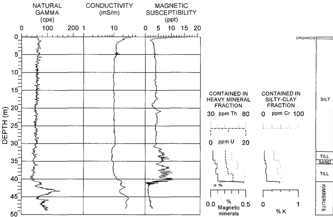
Figure 24-2: EM-39 borehole logs and selected geochemical results from hole B-30-10, a kimberlite prospect near Kirkland Lake, Ontario. This borehole is located approximately 200 metres south of B30-03. U = uranium, Th = thorium, K = potassium, Cr = chromium
