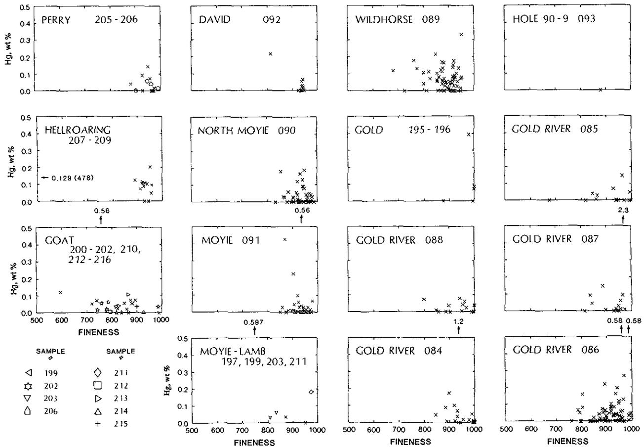
Figure 13-2. Scatter plots of fineness versus wt% mercury for the samples in Figure 13-1. Detection limit for mercury is 0.065 wt%.
