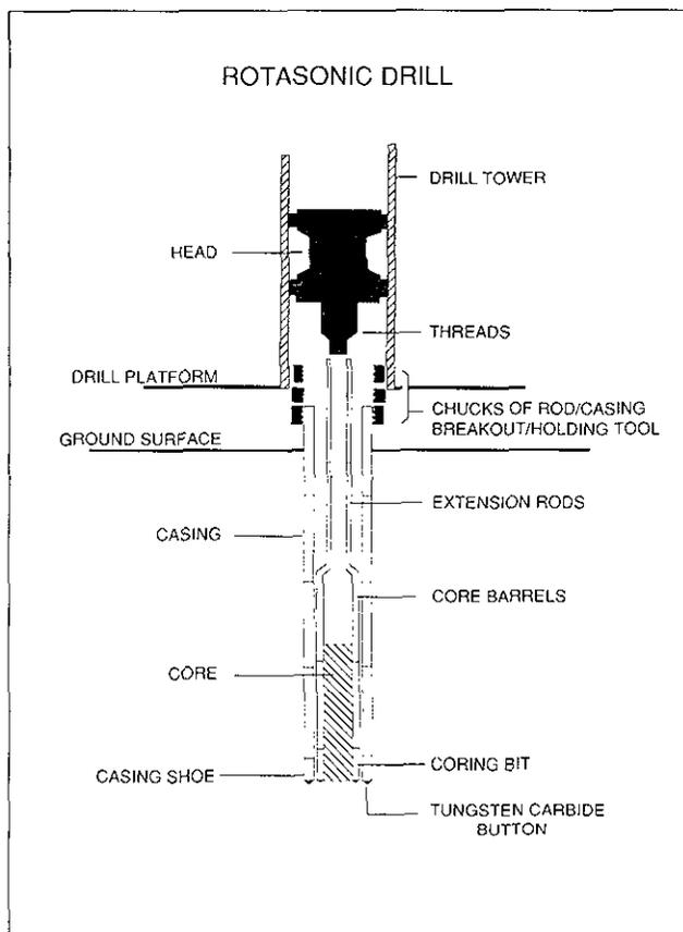
Figure 4-2. Schematic cross-section of a rotasonic drill; modified from McClenaghan (1991).
