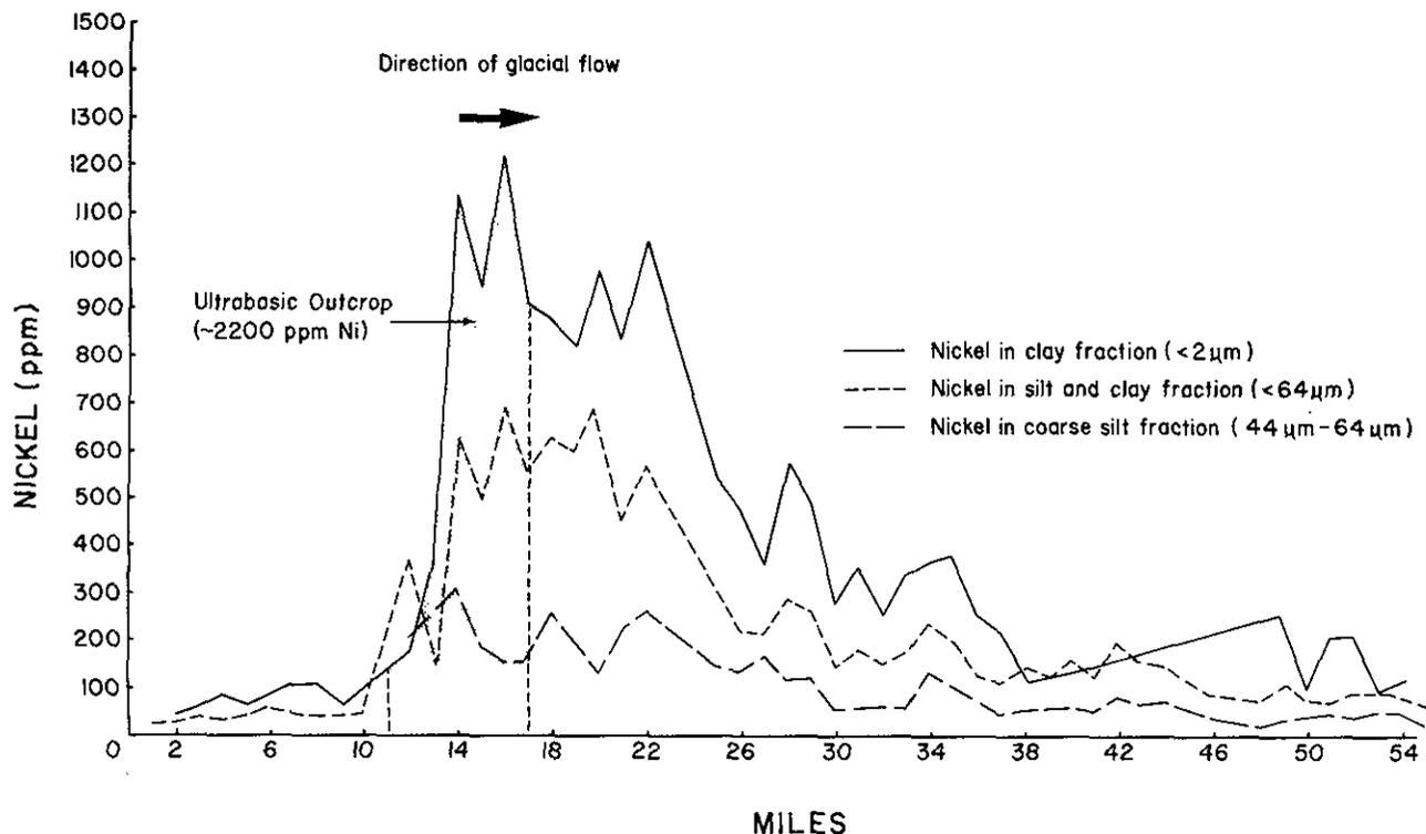
Figure 16-2. Profile of nickel concentrations in three size fractions of till along the axis of a dispersal train extending southeastward from ultramafic source outcrops near Thetford Mines, Quebec (modified from Shilts, 1991).
