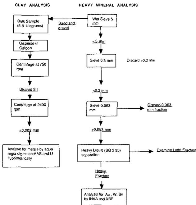
Figure 21-5. Processing and analysis for reversed drift samples from Eastern and Central Canada (Stea *et al.*, 1986).
