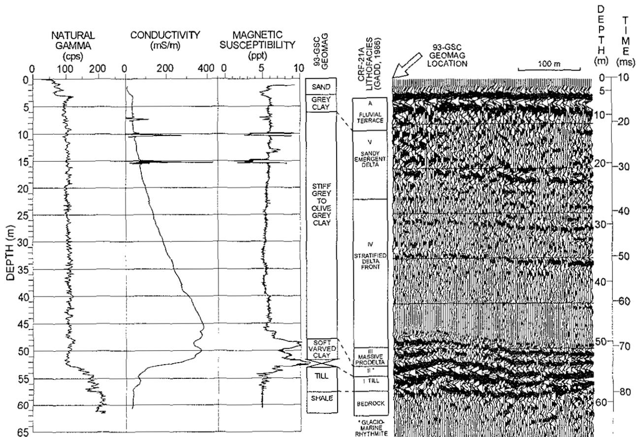
Figure 23-4: EM-39 borehole logs and high-resolution seismic section at the Anderson Road borehole, 93-GSC GEOMAG. Time, shown to the right of the seismic section, is measured as two-way travel time in milliseconds, and is converted to depth (on the adjacent scale) with interval velocity corrections.
