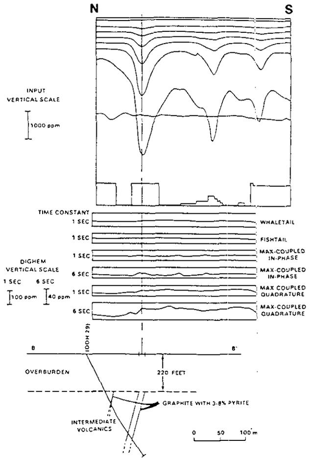
Figure 25-9. Input and Dighem responses over drill hole 29.
