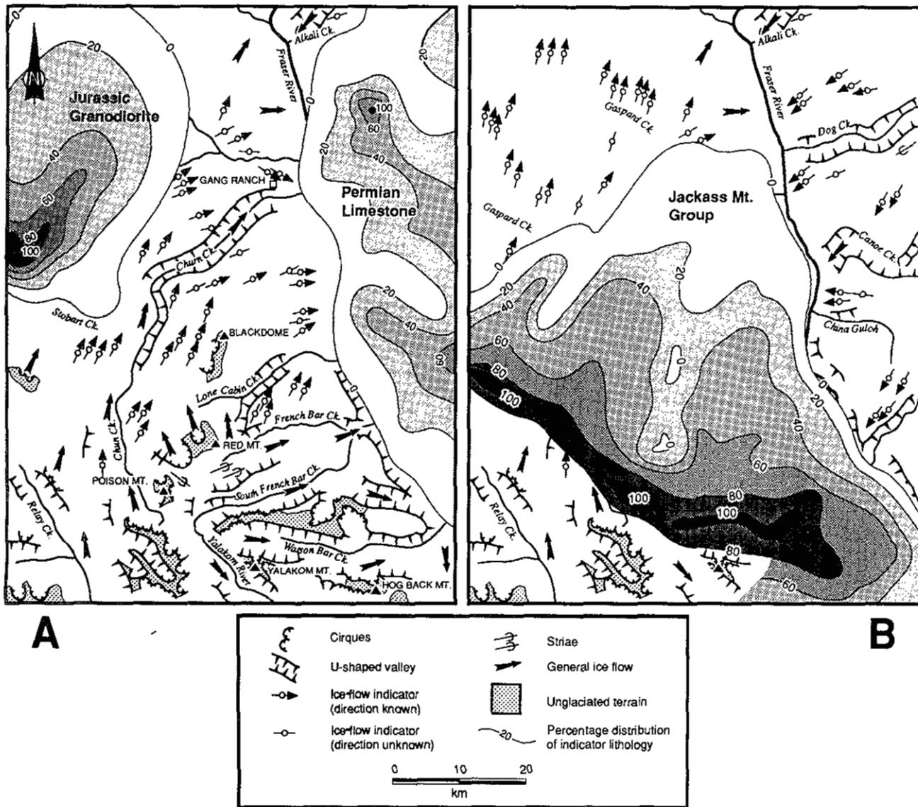
Figure 12-4. Dispersal patterns of clast lithologies in till, for: (a) Jurassic granodiorite and Permian limestone, (b) Jackass Mountain Group clastic sediments. Note change in glacial directional indicators and paucity of clast dispersal due to an ice divide at the Fraser River.
