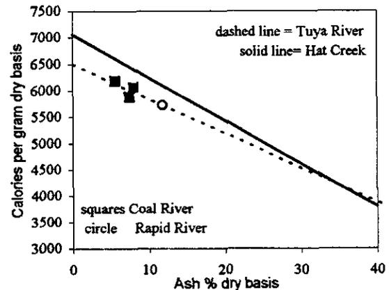
Figure 5. Plot of heat value *versus* ash, dry basis, for a number of Tertiary lignites from British Columbia.
