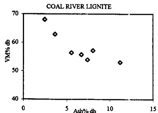
Figure 3. Plot of ash versus volatile matter, dry basis, for Coal River lignite data.
