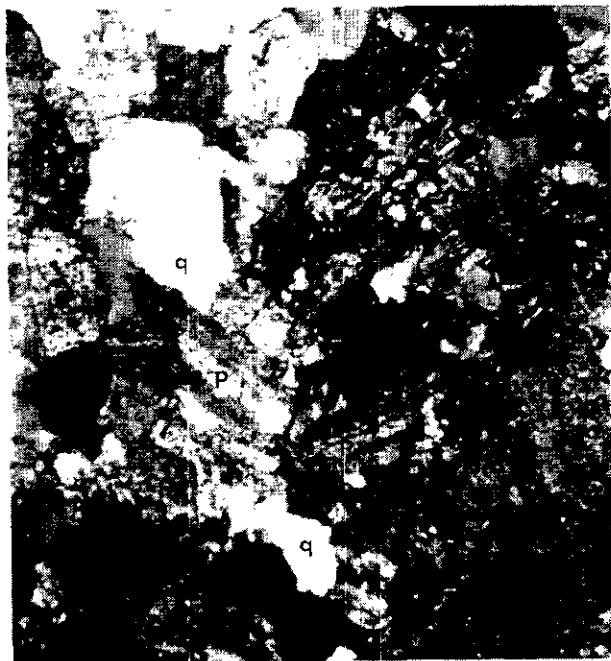
Figure 3. a) photomicrograph of rhyolite crystal tuff (96A-2) showing a broken quartz grain (photograph width 5 mm), b) photomicrograph of tonalite (96A-7) showing equigranular texture (photograph width 5 mm), p = plagioclase, q = quartz.
