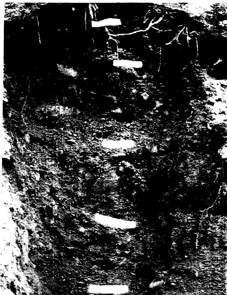
Photo 2. Vertical sampling profile at the Trail Peak property in colluvial sediments overlying till.
