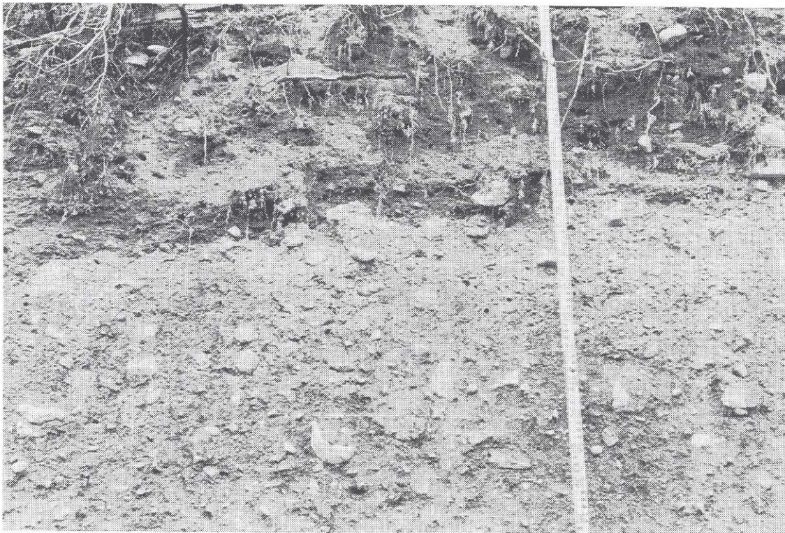
Photo 3. Massive gravelly sand (colluvium), about 70 centimetres thick, overlying 1 metre of massive, sandy diamicton interpreted as glacial debris-flow deposits (resedimented till).
